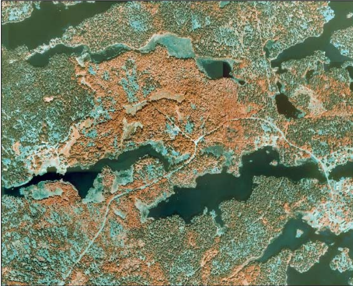
Figure 4-6. Example of a processed infra red image. Bluish and greenish tint is found where pine dominates and where the ground is comparatively dry, and brownish tint where the ground is wet or the trees carry leaves.
