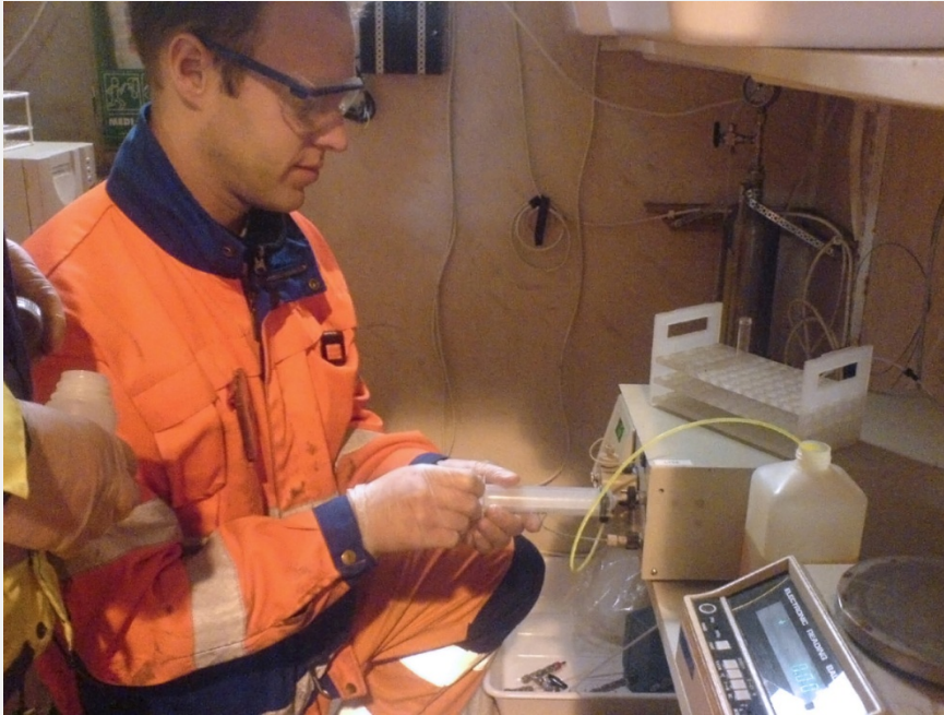
Injection of tracer in fracture.
