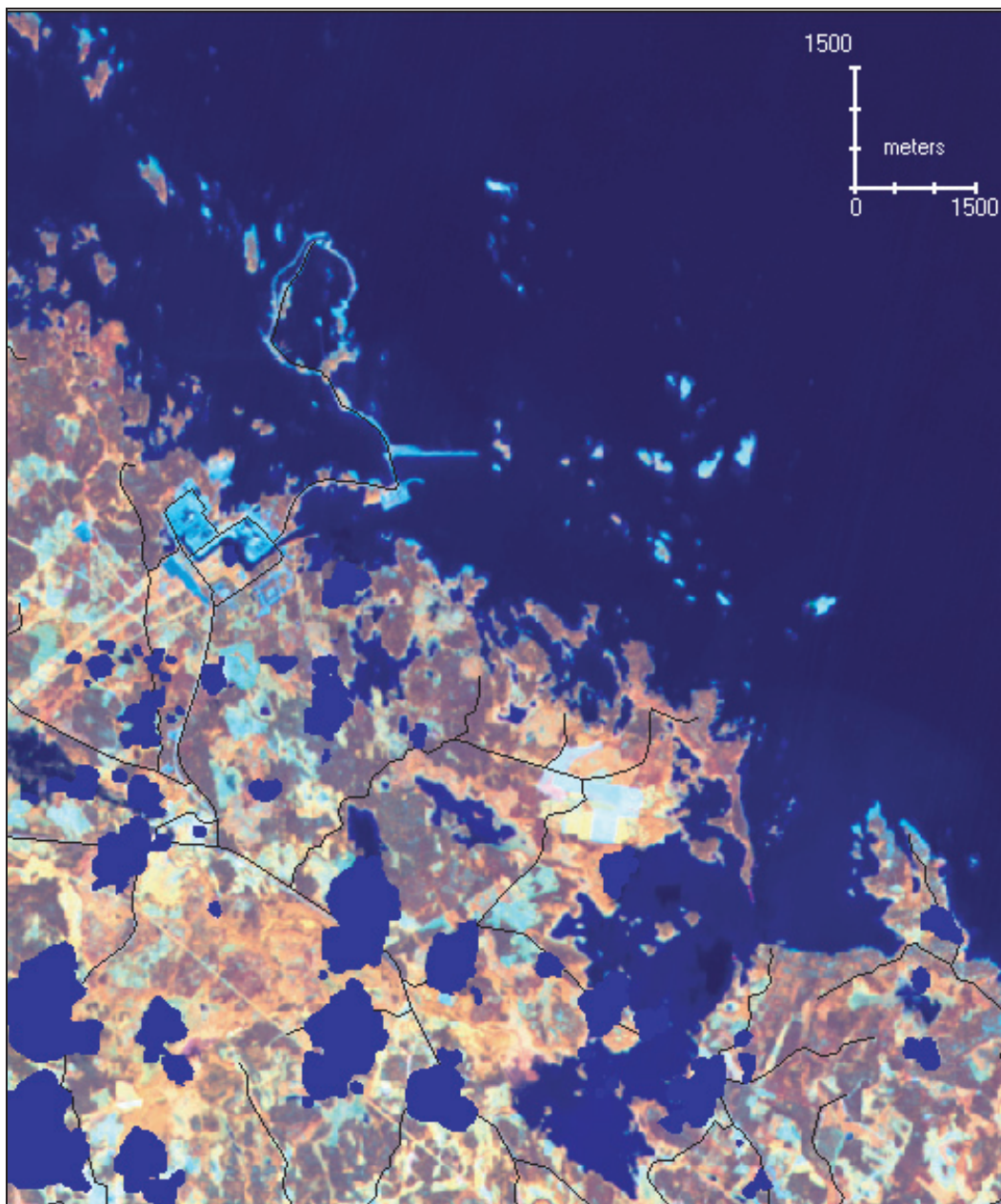
Figure 3-2. The cloud mask for the Forsmark area. Clouds and cloud shadows are shown in blue colour.
