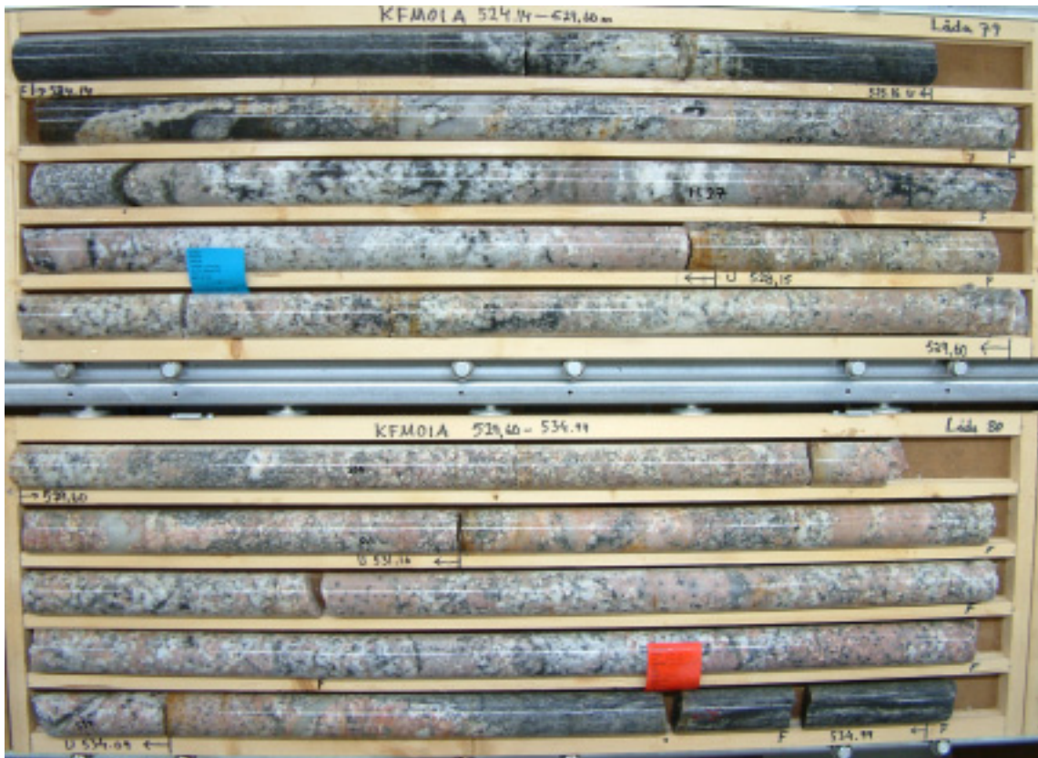
Picture A3-4. Core of KFM01A, lower segment of the -500 m section (at Length 524.14–524.8 m along KFM01A).
