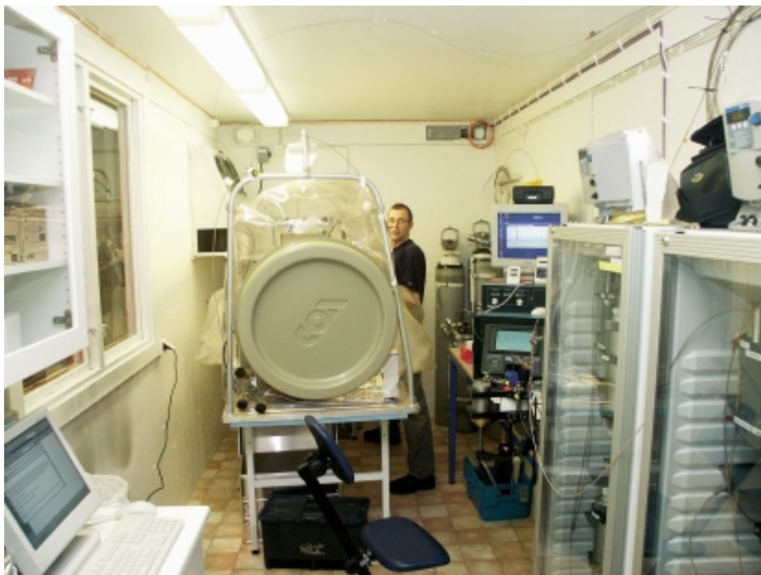
Figure 2-20. The Microbiology Laboratory environment at the MICROBE 450-m site is equipped with three circulation systems (right), an anaerobic box (forward), an in situ gas extractor and a Kappa 5 gas chromatograph (right of the anaerobic box).
