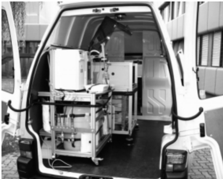
Figure 2-16. Equipment for Laser-Induced Breakdown-Detection (LIBD) of colloids. The equipment is installed in a van in order to allow mobility and on-line measurements.
