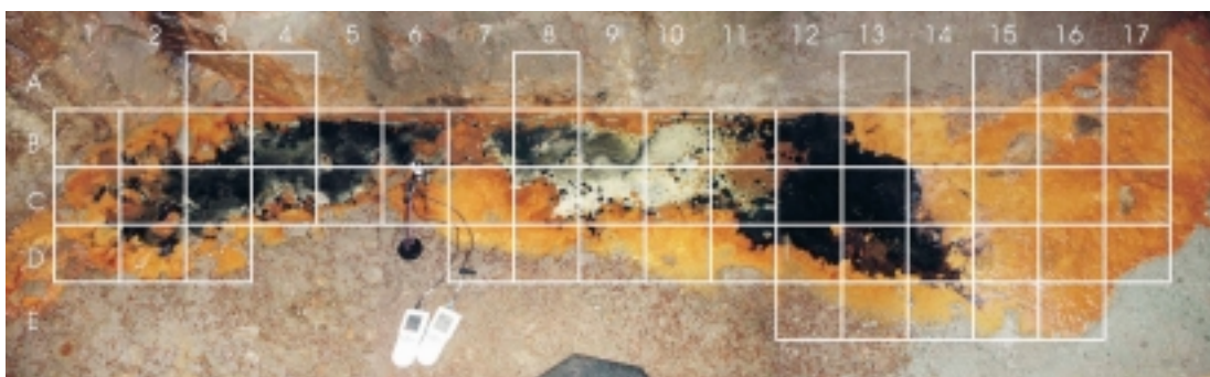
Figure 2-23. The 907-m ditch site is characterised by a shallow, elongated water pond that overflows into the main tunnel ditch to the right in the image. Brown material is BIOS. The black colour is from iron sulphide precipitates and the white material is calcium carbonate. The overlaid grid created an organised environment and enabled pH, oxygen and redox measurements in three dimensions (Figure 2-24). Field instruments are shown in the bottom of the figure. Grid size is about 25 x 25 cm.
