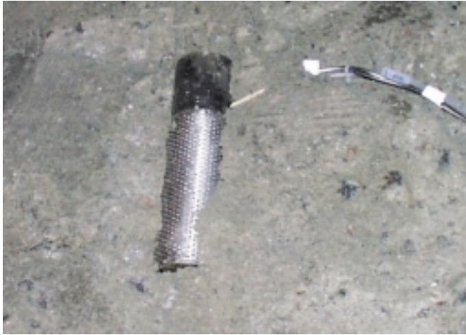
Figure 5-14. DPP sensor installed close to the rock face.
