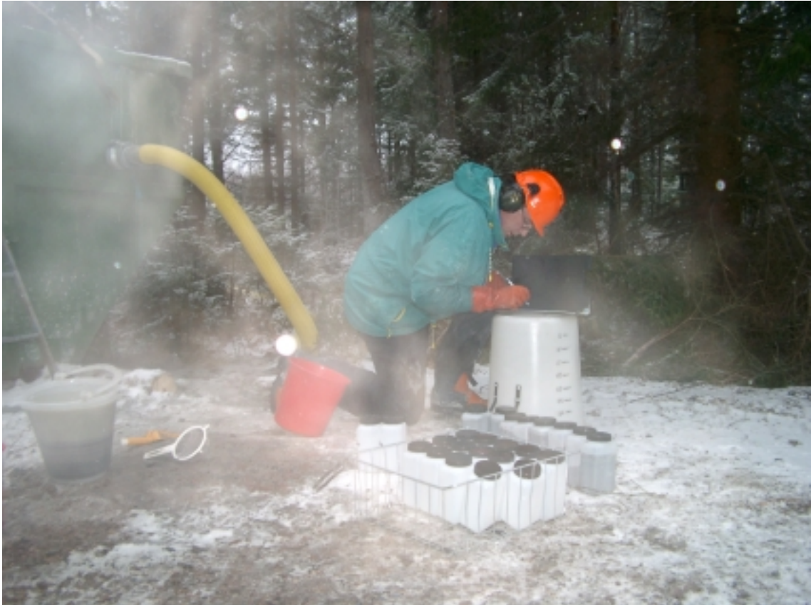
Figure 4-3. Sampling of one sample per 3 metre drill length of drill cuttings from the bedrock. Photo Alf Sevastik.
