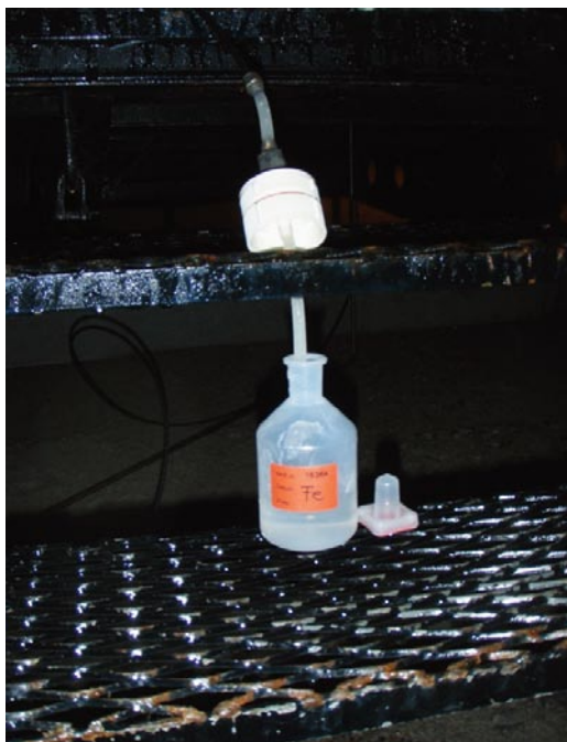
Figure 5-1. Water sampling. The photograph shows the water outlet, the filter holder for on-line filtering and a sample bottle.
