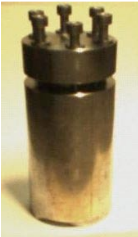
Figure 6-8. Autoclave for test of (U,Zr)N compatibility with water under LWR conditions.
