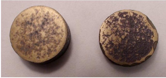
Figure 6-6. Unpolished ZrN pellets sintered by the SPS technique.
