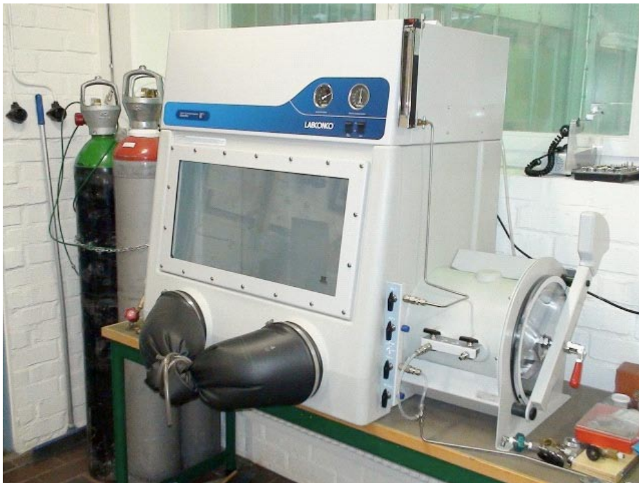
Figure 6-1. Glove box installed in the uranium laboratory at KTH.
