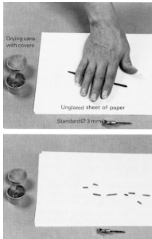
Figure 8-13. Determination of the plastic limit. Upper: Rolling of sample. Lower: Required final state. Glazed sheets of paper may also be used.
