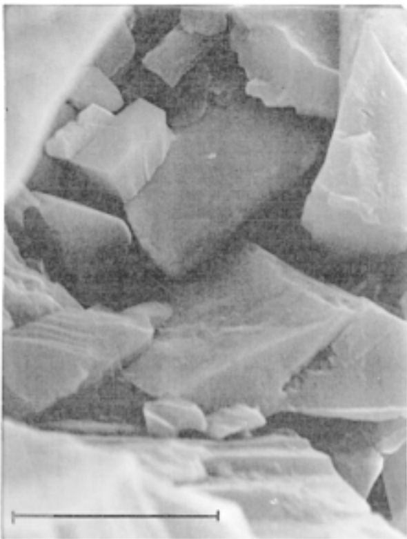
Figure 6-8. Silt grains (quartz) of glacial origin. The length of the bar represents 10 \mu\text{m} .
