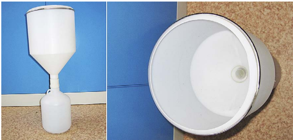
Figure 3-1. The sampler used in summer at the site for sampling of precipitation at the island of Äspö.
