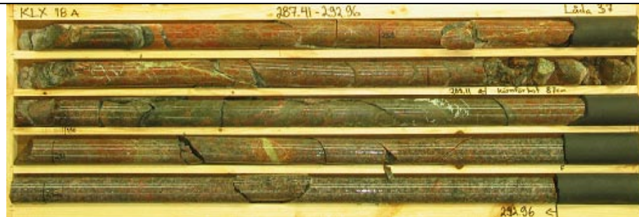
KLX18A 287-293 m borehole length. Part of DZ3, including core zone 287.29-290.70 m.
