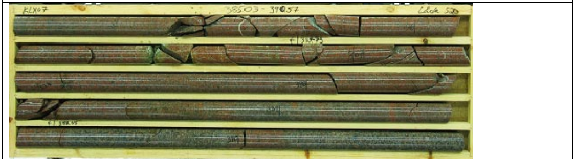
KLX07A 385.03-390.57 m borehole length. Part of DZ7, including core zone 386.3-386.7 m.
