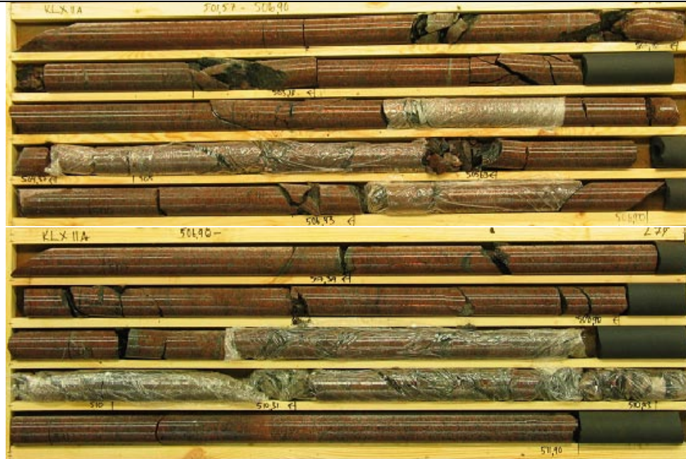
KLX11A 501.57-511.90 m borehole length. Part of DZ11 including core zone 509.0-511.0 m.
