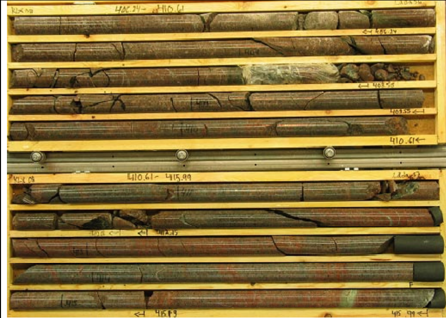
KLX08A 406.24-415.99 m borehole length. Part of DZ6, including core zone (405.77- 408.50 m)
