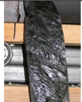
Slickensided fracture surfaces in the dolerite.
