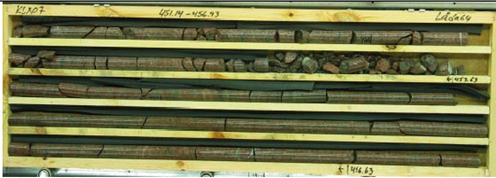
KLX07 451.14- 456.93 m borehole length. Part of DZ9 including core zone 452.80-453.8 m.
