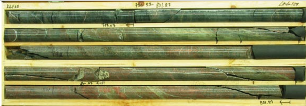
KLX03A 796.6-801.9 m borehole length. Part of DZ1c, including core zone 797-798 m.
