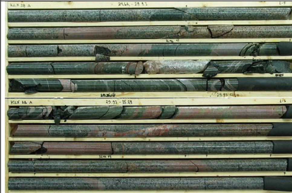
KLX28A 24.62-35.23 m borehole length. Part of DZ1 including core zone (27.7-30.35 m)
