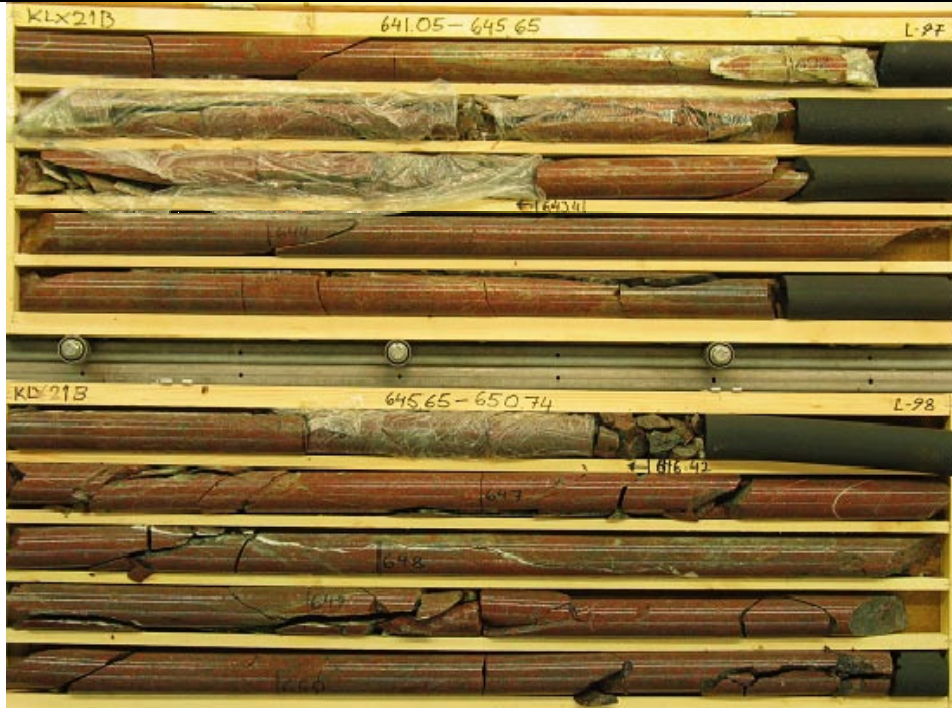
KLX21B 641.05-645.65 m Borehole length, part of DZ12 (595-707 m Borehole length). Note the zone is interpreted as have an orientation parallel to the Borehole. No defined core zone.
