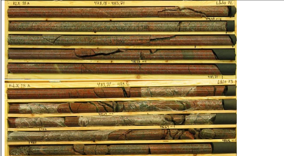
KLX18A 478.18-489.10 m borehole length. Part of DZ9, including core zone 484.1-487.0 m.
