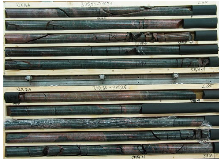
KLX16A 335-345 m borehole length. Part of DZ12 including core zone.
