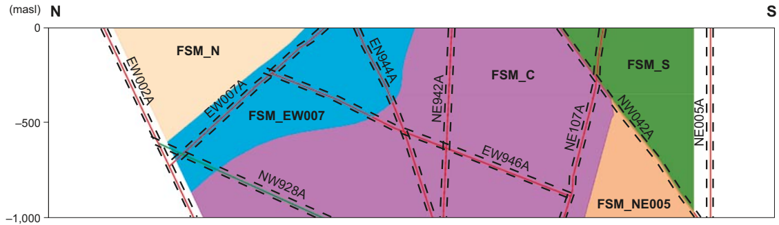
Figure 5-4. 2D vertical N-S section of the conceptual model for fracture domains in the local model volume /SKB 2009/.
