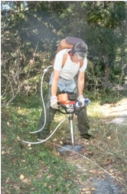
Figure 4-1. a) Petrophysical sampling by use of water cooled drill machine. b) Orientation of drill core by use of sun compass.
