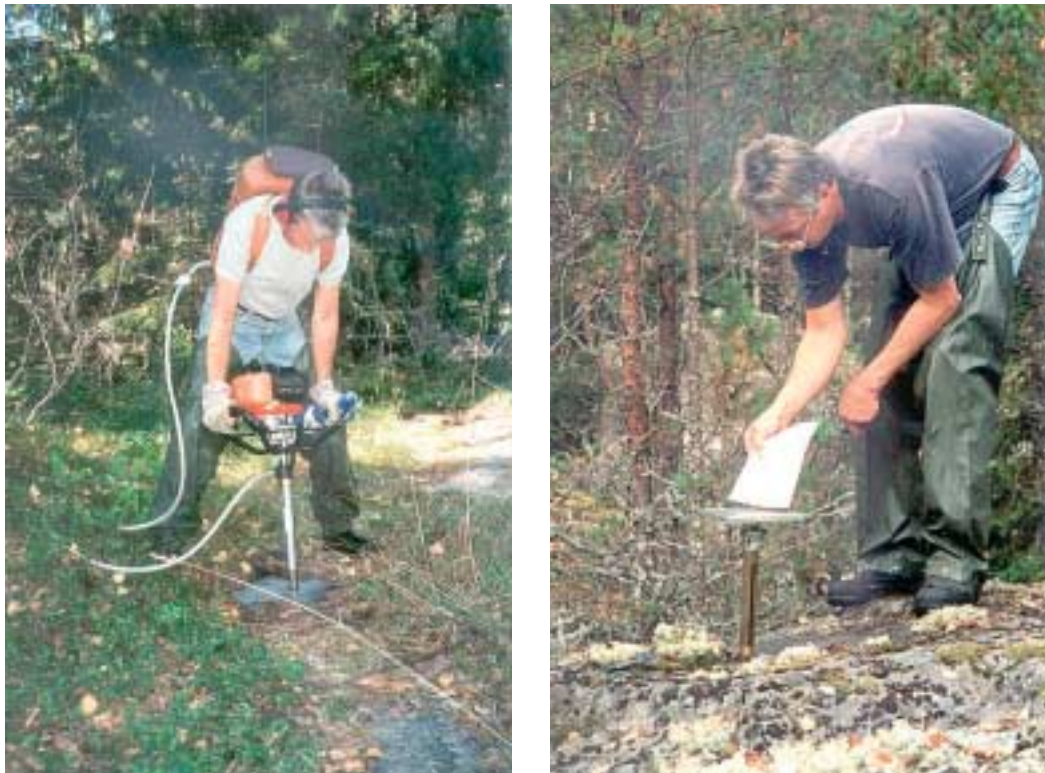
Figure 4-1. Drilling of a petrophysical sample and orientation of core using a sun compass.
