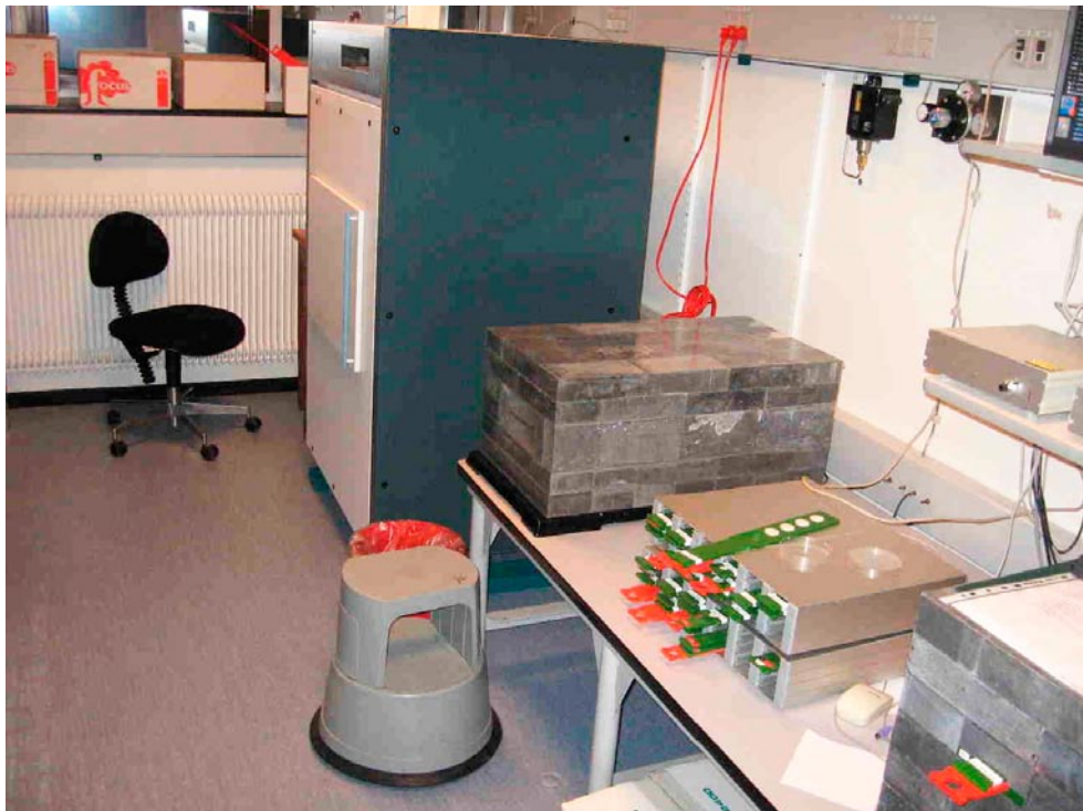
Figure 4-2. The Quantulus LSC is the cabinet shown in the background behind a set-up of the ordinary anticoincidence shielded GM gas flow counters in a lead cave in the foreground.
