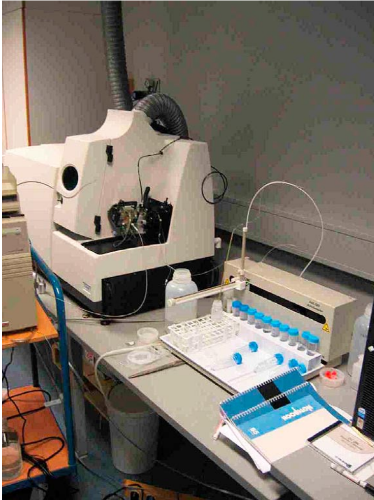
Figure 4-4. The ICP-MS system used for the analysis of Th and U isotopes.
