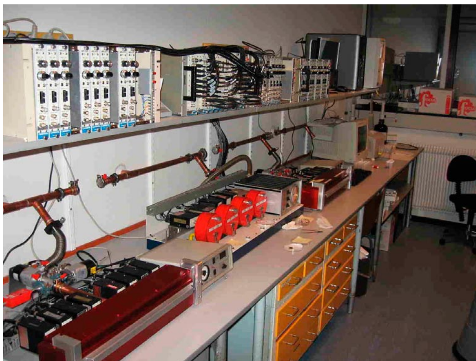
Figure 4-3. The solid state alpha spectrometry system used for the alpha spectrometry of thorium.
