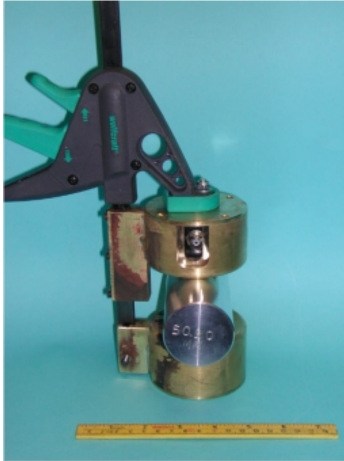
Figure 2-1. NGI's apparatus for measuring acoustic P-wave travel time transverse borehole core.
