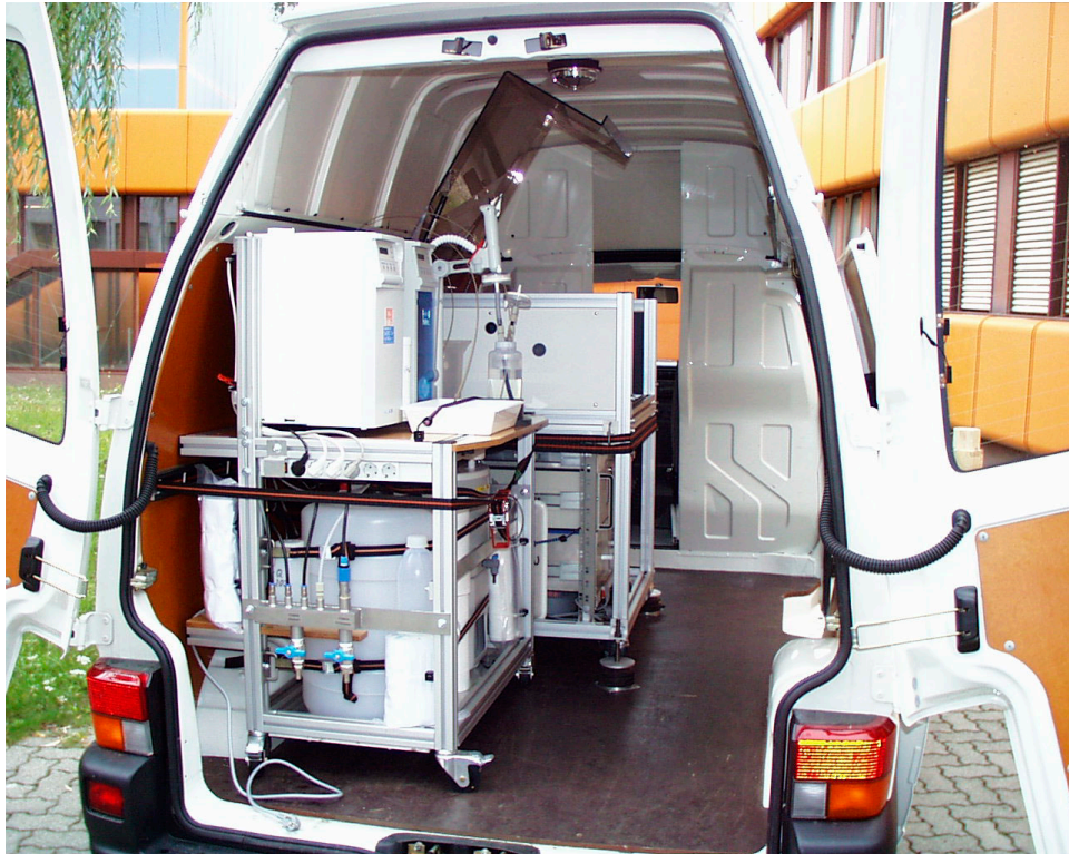
Figure 2-6 The equipment for Laser-induced Breakdown-Detection (LIBD) of colloids is installed in a van in order to allow mobility and on-line measurements at a bore hole.
