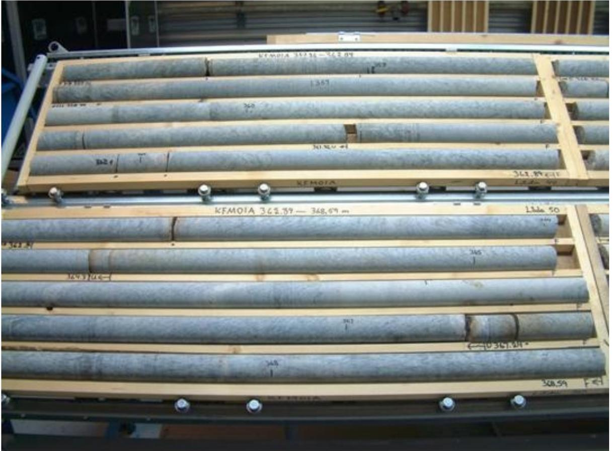
*Figure 8-1. Example of 'background rock mass quality', from 357 to 369 m.*
