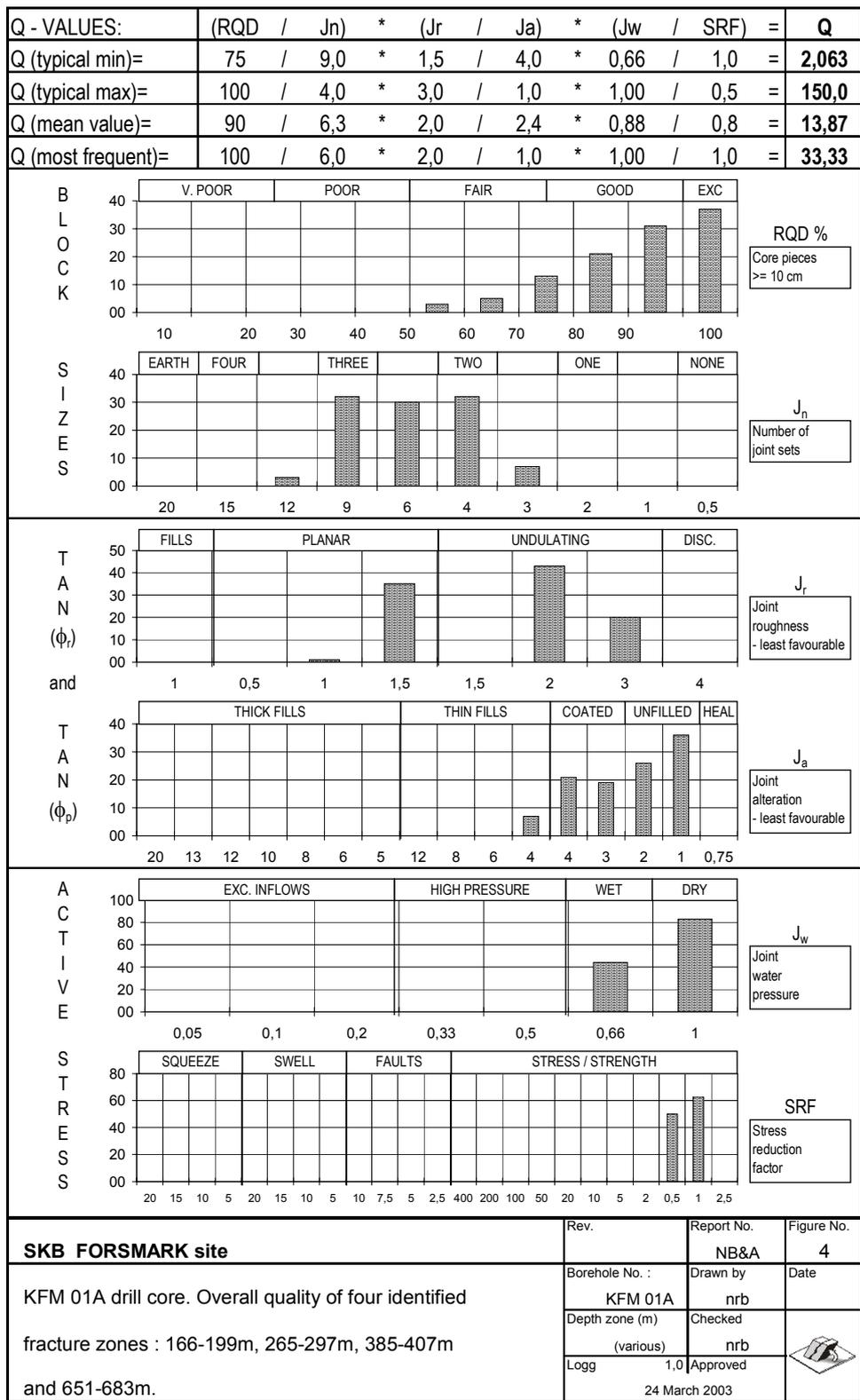
Figure 5-1. Q-parameter histograms for the four identified fracture(d) zones.
