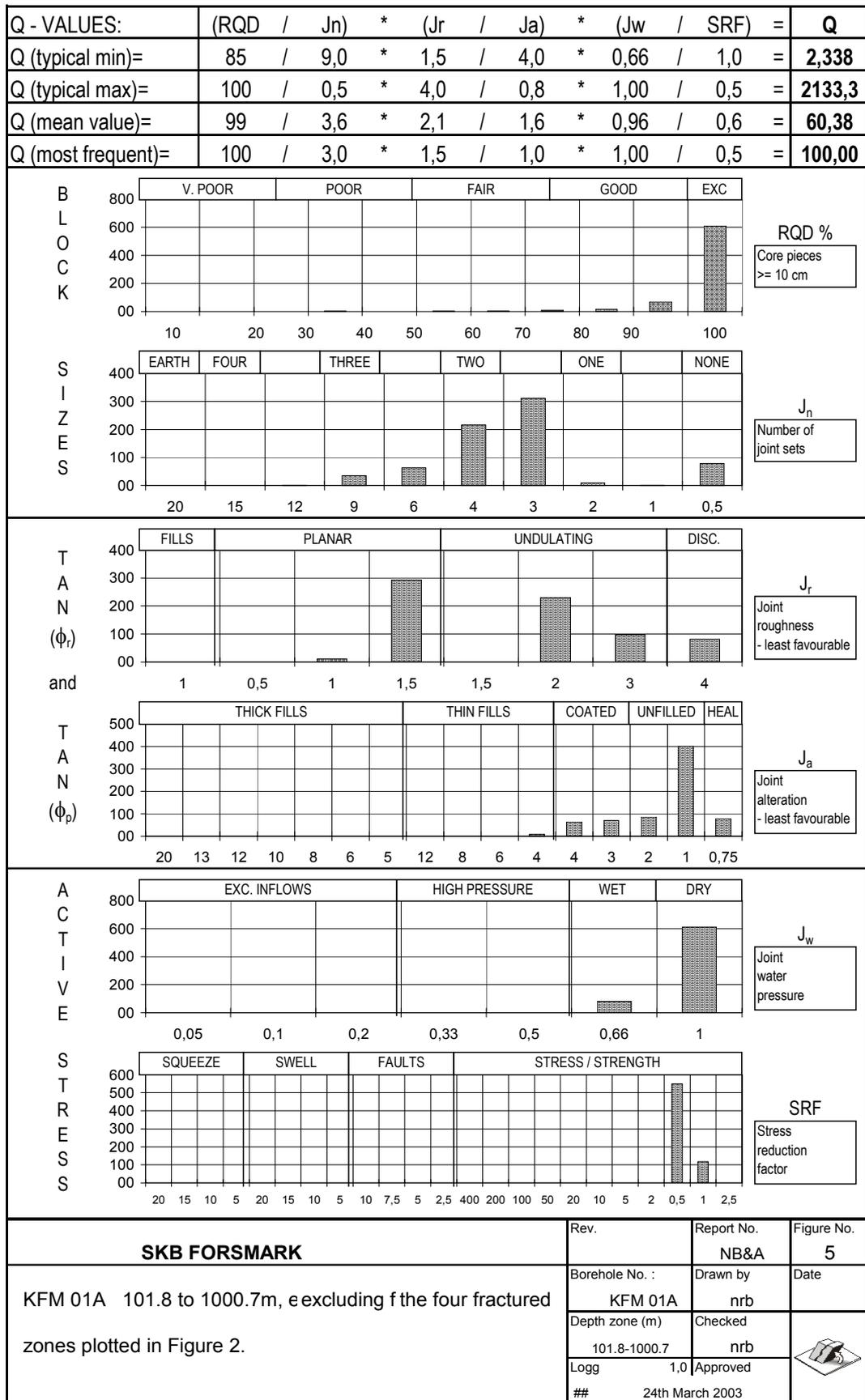
Figure 6-1. Q-parameter histograms for the 'average' rock mass, with the four fracture(d) zones excluded.
