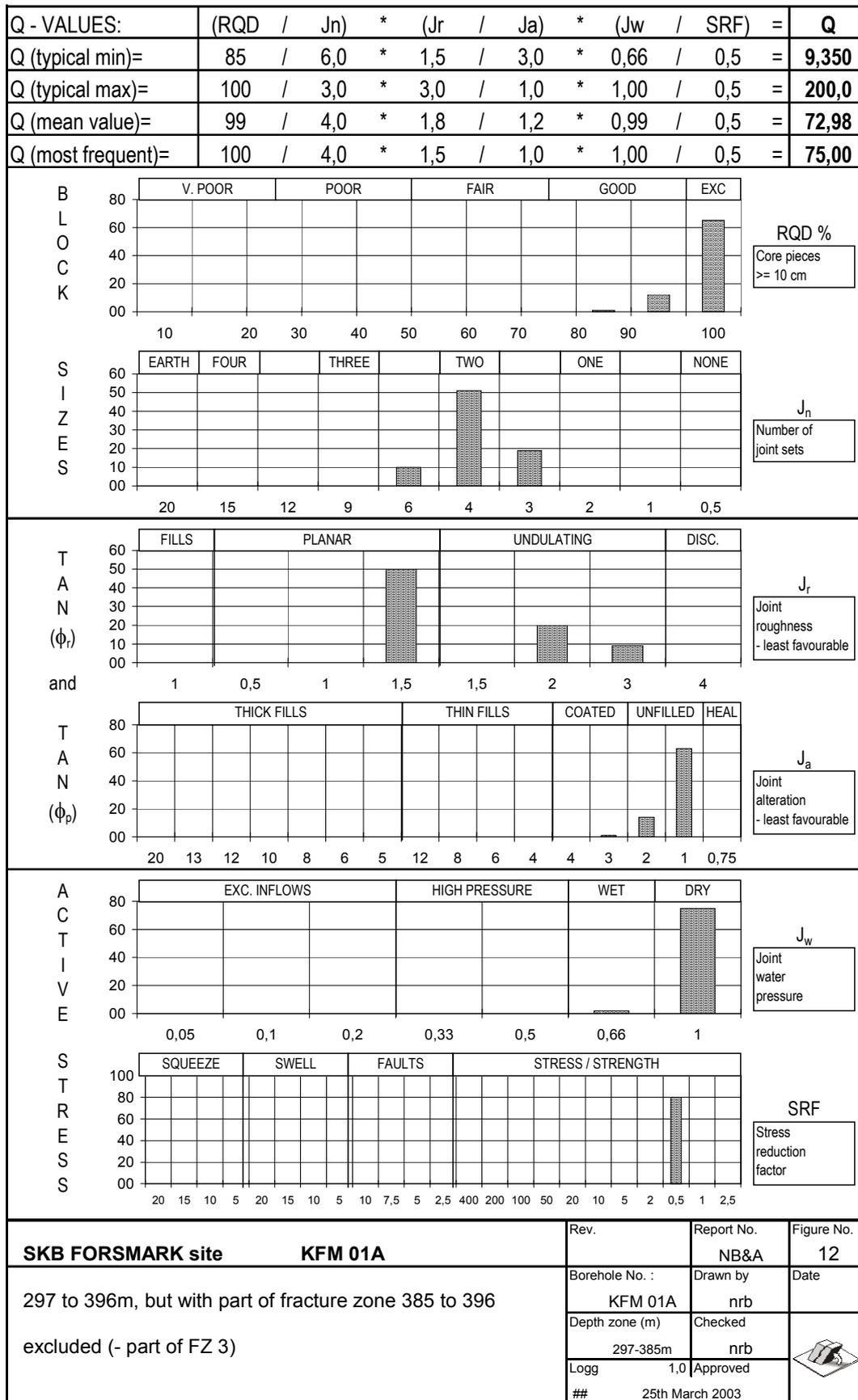
Figure 8-2. Q-histograms for mid-depth 'slice' 297-385 m.
