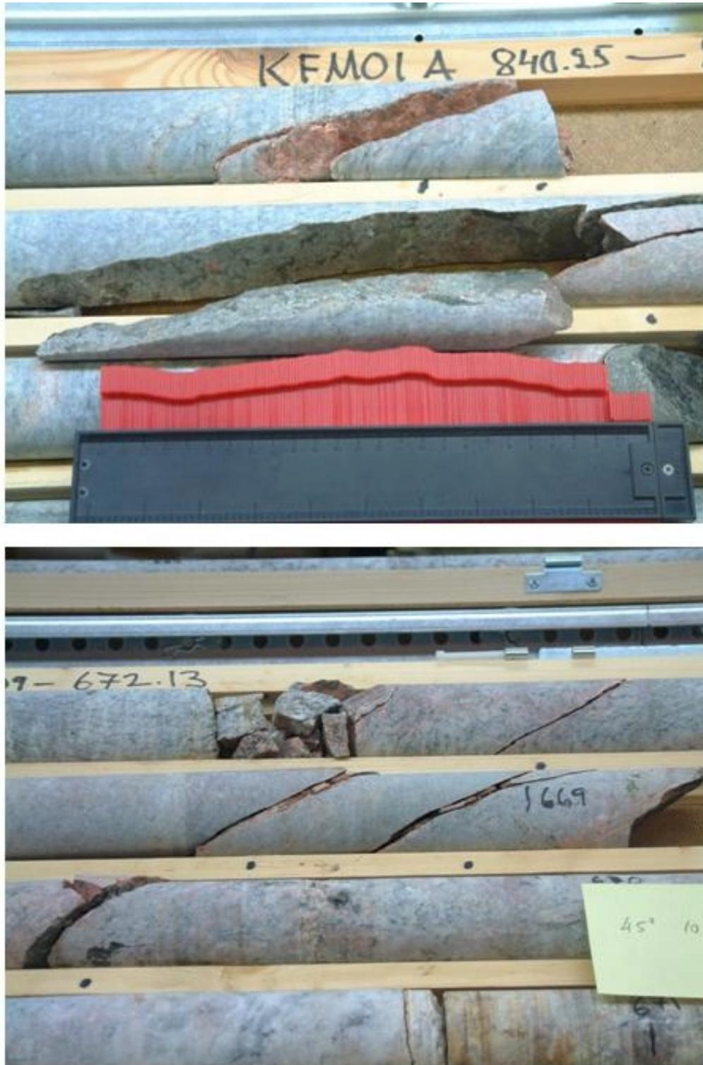
**Figure 3-2.** a) Example of joint roughness  $J_r = 3$  (typical of 'steep dipping' joints) and b) of  $J_r = 1.0$  to  $1.5$  in the case of a thinly filled discontinuity (with  $J_a = 4$ ). The latter is from the fourth identified fracture(d) zone, termed FZ 4 here.
