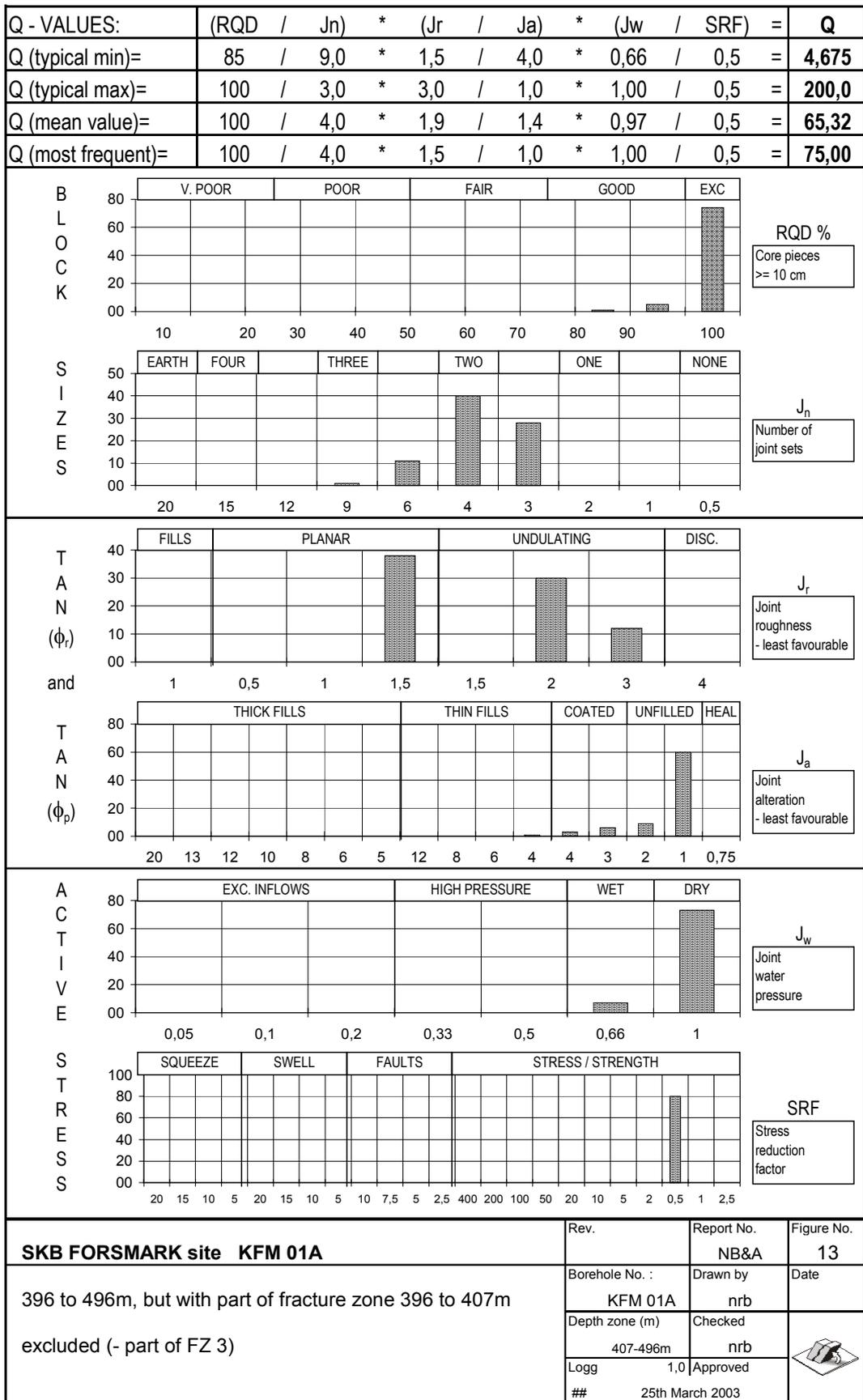
Figure 8-3. Q-histograms for mid-depth 'slice' 407–496 m.
