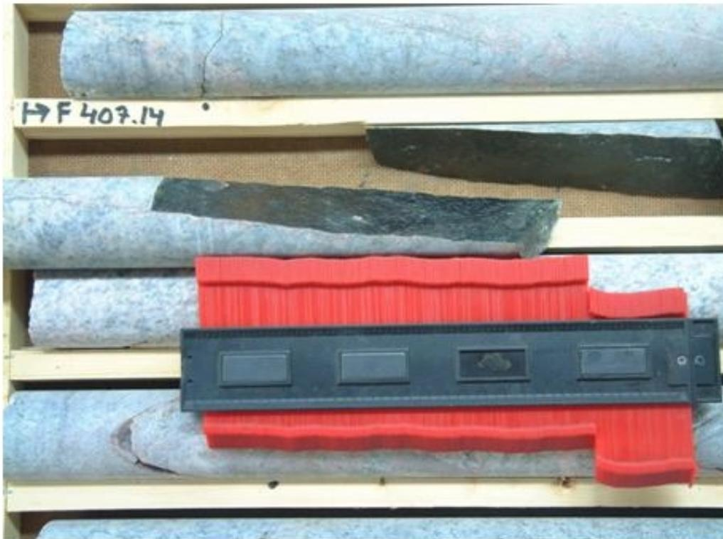
**Figure 3-1.** a) Example of joint roughness  $J_r = 1.5$  and b)  $J_r = 2$  (the most frequent), and of '+/- 45° dip' and 'steeply dipping' joints.
