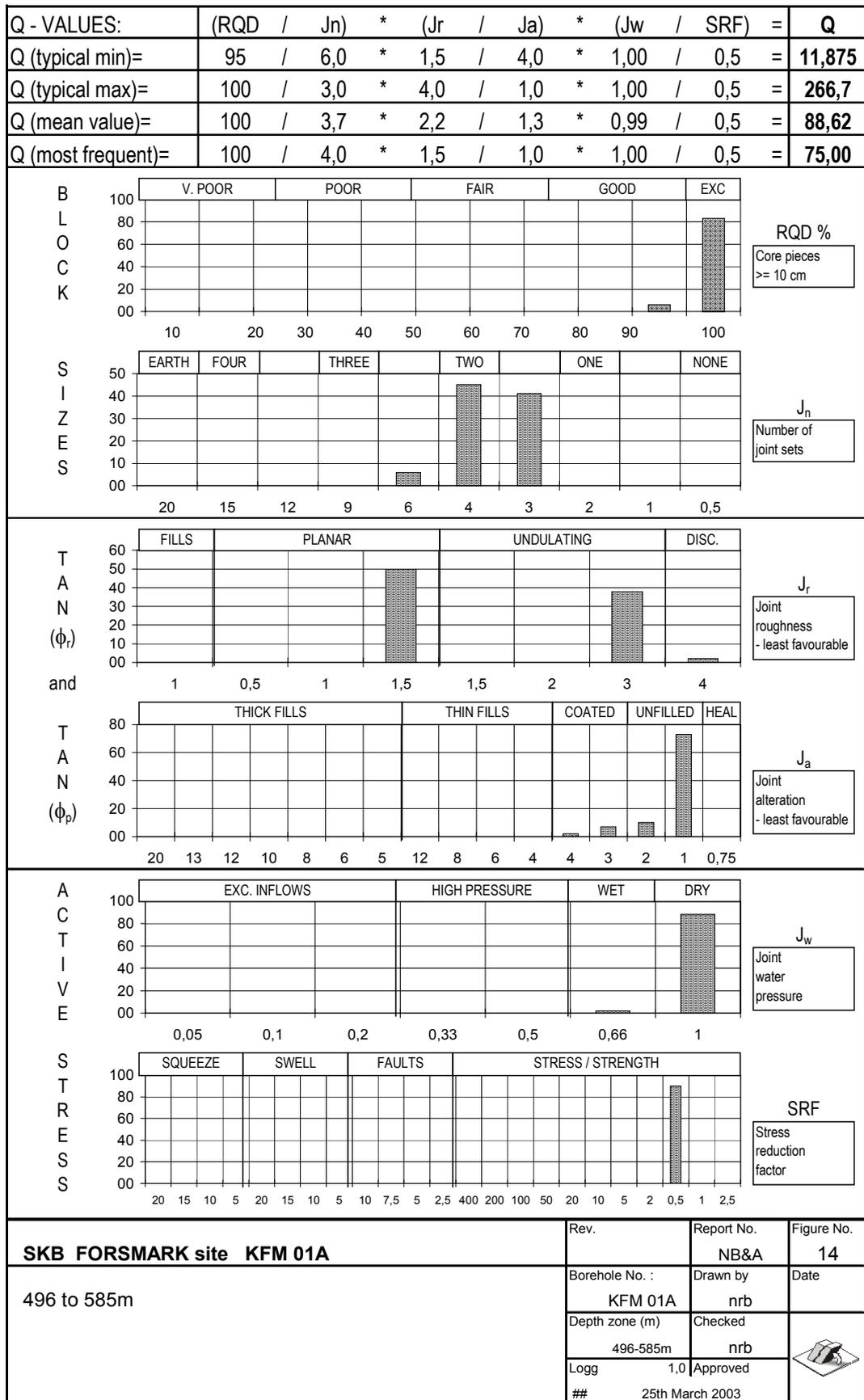
Figure 8-4. Q-histograms for mid-depth 'slice' 496–585 m.
