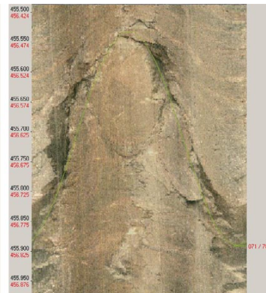
Figure 5-6. A sealed fracture that looks like a crush in the BIPS-image, despite an intact core.
