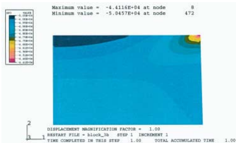
Figure 8-15. FEM-derived stress focus at upper edge of compacted block /6/.
