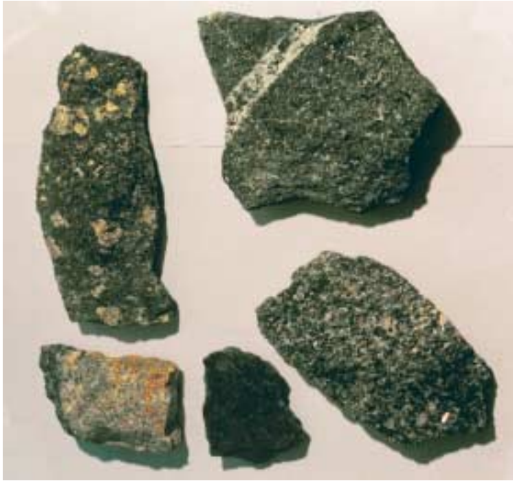
Figure 4-17. TBM chips with typical platy shape. The large diameter a is 1.2 to 2.2 times the intermediate diameter b , which is 2-3 times the smallest diameter c .
