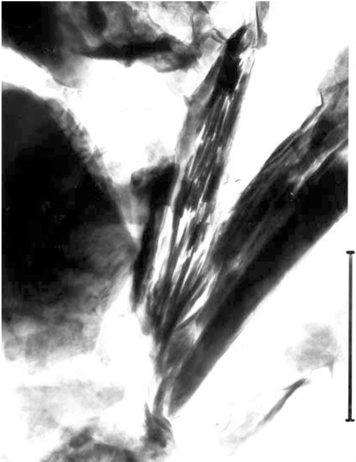
Figure 3-8. Transmission electron micrograph of postglacial clay with mica grain (center) degraded by weathering or shearing, by which a large number of internal surfaces have been exposed. Scale is 100 \mu\text{m} .
