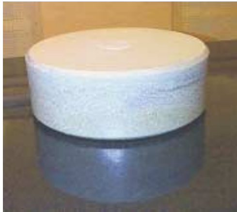
Figure 7-7. Block compaction. Upper: Available gradation of bentonite materials. They can all be used for preparing highly compacted blocks but the size distribution of the IBECO materials may be preferable. The lower picture shows a block compacted under 100 MPa pressure using the IBECO C material where one can identify the presence of large compressed grains. After wetting the materials becomes virtually homogeneous. The density including 10% water content is 2200 \text{ kg/m}^3 .
