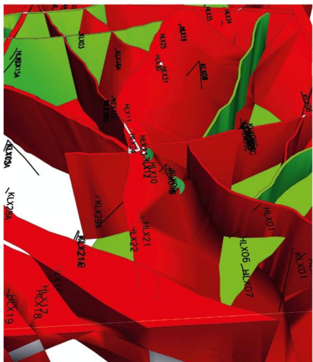
Figure A1-30. Test in January–February 2005 with HLX10 as pumping borehole. A few deformation zones south of ZSMEW007A, ZSMNW928, ZSMNE012A and ZSMNE107A removed to show responses. Top of figures: west part of the local model area. Response indexes are mapped on the boreholes. Pumping hole plotted as a black disc. The larger the disc (green or blue) for a response index is, the better hydraulic contact with pumped borehole section can be assumed. No-response is indicated with a grey sphere. A borehole without discs or spheres have not been measured.
