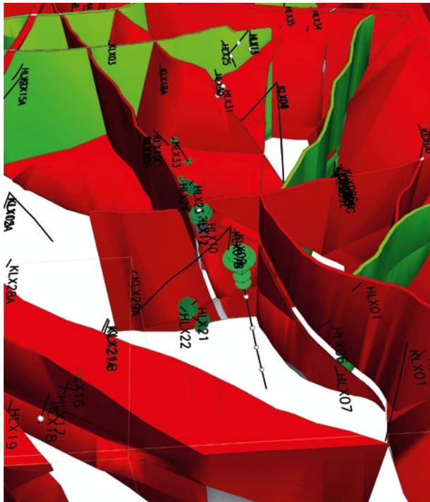
Figure A1-31. Test in January–February 2005 with HLX10 as pumping borehole. A few deformation zones south of ZSMEW007A, ZSMNW928, ZSMNE012A and ZSMNE107A removed to show responses. Top of figure: west part of the local model area. Response indexes are mapped on the boreholes. Pumping hole plotted as a black disc. The larger the disc (green or blue) for a response index is, the better hydraulic contact with pumped borehole section can be assumed. No-response is indicated with a grey sphere. A borehole without discs or spheres have not been measured.
