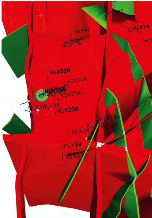
Figure A1-18. Test in November 2006 with KLX20:2 (99.5–180 m as pumping borehole. Top of figures: north part of local model area. Response indexes are mapped on the boreholes. Pumping hole plotted as a black disc. The larger the disc (green or blue) for a response index is, the better hydraulic contact with pumped borehole section can be assumed. No-response is indicated with a grey sphere. A borehole without discs or spheres have not been measured. (RVS_INFO 13144402).
