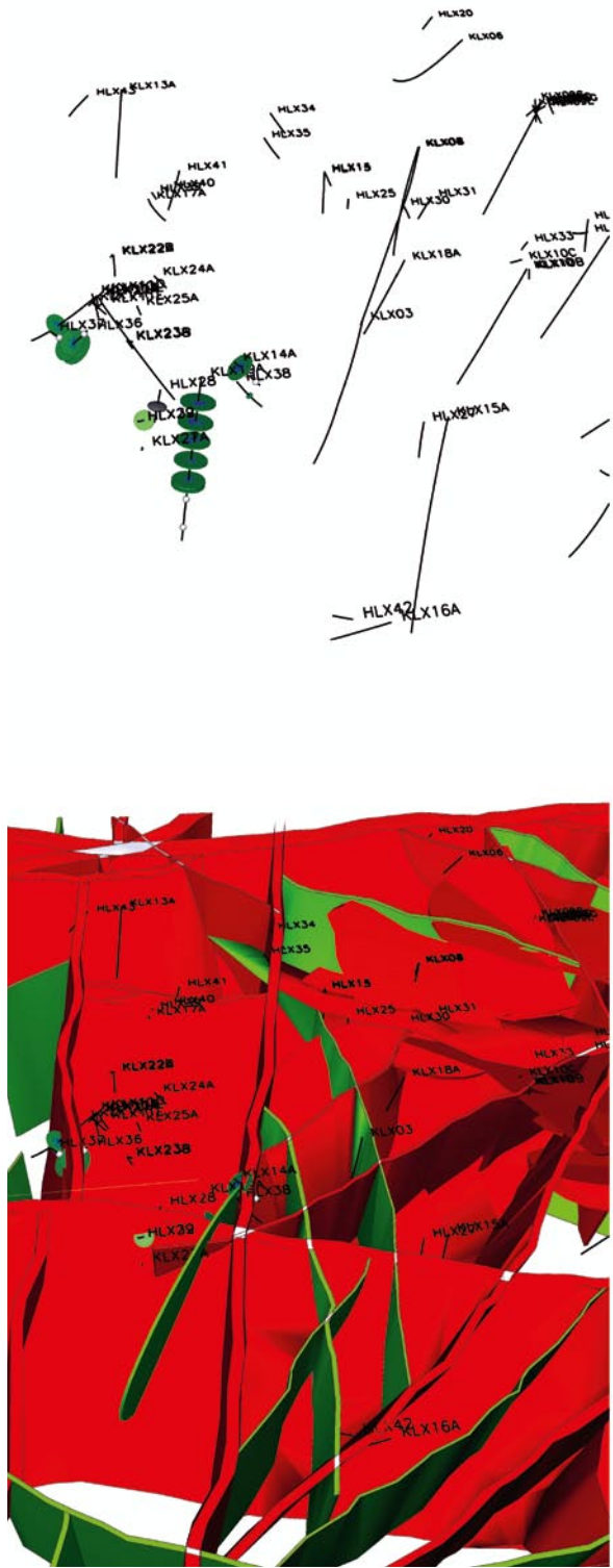
Figure A1-9. Test in April 2007 with HLX28 as pumping borehole. Top of figures: north part of local model area. A steeply dipping dolerite dyke striking NNE intersects KLX19A below the responses in the borehole. Response indexes are mapped on the boreholes. Pumping hole plotted as a black disc. The larger the disc (green or blue) for a response index is, the better hydraulic contact with pumped borehole section can be assumed. No-response is indicated with a grey sphere. A borehole without discs or spheres have not been measured.
