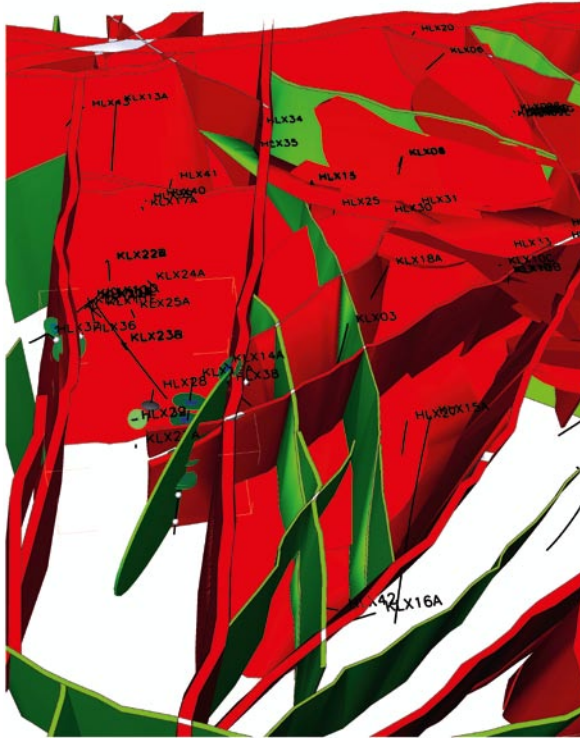
Figure A1-10. Test in April 2007 with HLX28 as pumping borehole. Top of figures: north part of local model area. Deformation zone ZSMNW042A and hlX28_dz1 (a subhorizontal disc intersection HLX28) are removed in the figure to better show responses. A steeply dipping dolerite dyke striking NNE intersects KLX19A, KLX19_DZ5-8_DOLERITE, below the responses in the borehole. Response indexes are mapped on the boreholes. Pumping hole plotted as a black disc. The larger the disc (green or blue) for a response index is, the better hydraulic contact with pumped borehole section can be assumed. No-response is indicated with a grey sphere. A borehole without discs or spheres have not been measured.
