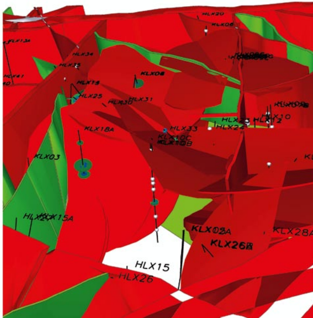
Figure A1-37. Test in September 2006 with KLX08A:3 (357–497 m) as pumping borehole. Top of figures: north-west part of local model area (DZ modelled as discs around boreholes are shown). Deformation zones ZSMEW007, ZSMNE942A, ZSMNE944A, ZSMNE107A and ZSMNE946A removed to show responses. Response indexes are mapped on the boreholes. Response indexes mapped on the structural model. Pumping hole plotted as a black disc. The larger the disc (green or blue) for a response index is, the better hydraulic contact with pumped borehole section can be assumed. No-response is indicated with a grey sphere. A borehole without discs or spheres have not been measured (RVS_info: KLX08–13140113).
