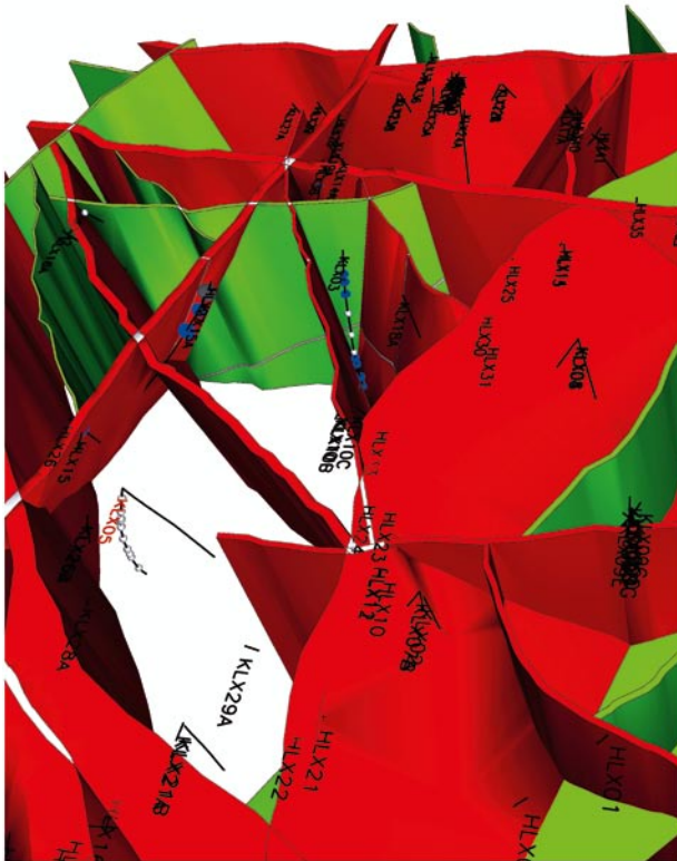
Figure A1-5. Test in May–June 2007 with HLX27 as pumping borehole. Top of figures: western part of local model area. Deformation zones ZSMEW946A and ZSMNS945A are removed in the figure to better show responses. Response indexes are mapped on the boreholes. Pumping hole plotted as a black disc. The larger the disc (green or blue) for a response index is, the better hydraulic contact with pumped borehole section can be assumed. No-response is indicated with a grey sphere. Boreholes without discs or spheres have not been measured.
