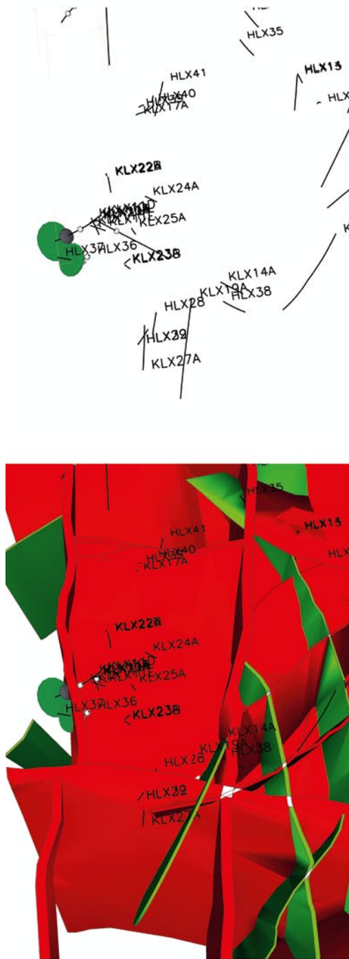
Figure A1-15. Test in November 2006 with KLX20:1 (250.2–306.2 m) as pumping borehole. Top of figures: north part of local model area. Response indexes are mapped on the boreholes. Pumping hole plotted as a black disc. The larger the disc (green or blue) for a response index is, the better hydraulic contact with pumped borehole section can be assumed. No-response is indicated with a grey sphere. A borehole without discs or spheres have not been measured. (RVS_INFO 13144401).
