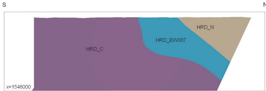
Figure 4-7. Illustration of the SDM-Site Laxemar Hydraulic Rock Domain Model, vertical section from south (left) to north at Easting's X = 154,800 m, cf Figure 4-6.
