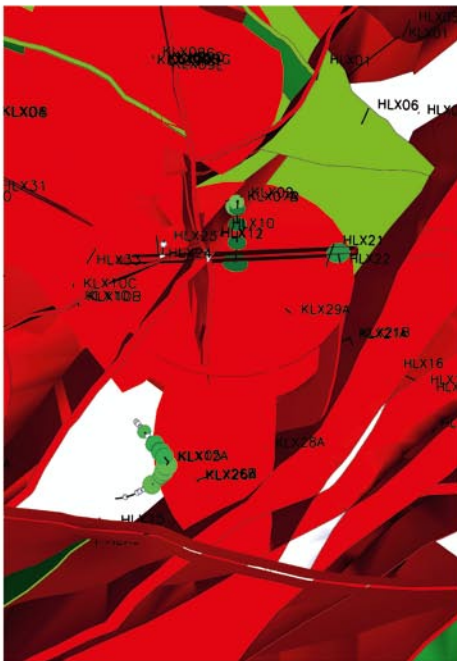
Figure A1-42. Test in March 2007 with KLX21B (11.9–858.8 m) as pumping borehole. Top of figures: north part of local model area (DZ modelled as discs around boreholes are not shown in uppermost figure but in the lower figure). Deformation zones ZSMEW007A is removed in the figures. Response indexes are mapped on the boreholes. Response indexes mapped on the structural model. Pumping hole plotted as a black disc. The larger the disc (green or blue) for a response index is, the better hydraulic contact with pumped borehole section can be assumed. No-response is indicated with a grey sphere. A borehole without discs or spheres have not been measured.
