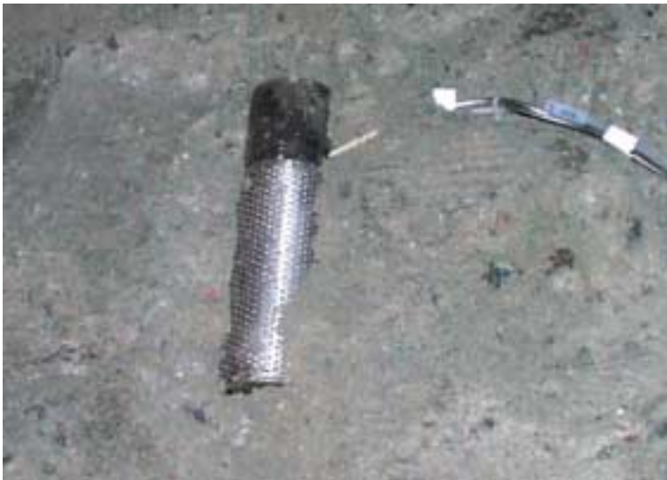
Figure 6-4. DPP sensor installed close to the rock face.
