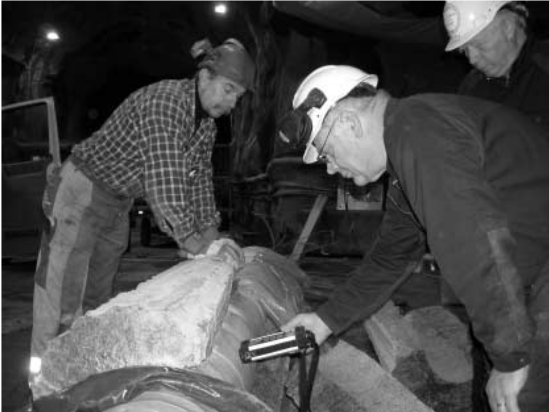
Figure 4-16. First check of radioactivity from tracer elements in the A0 parcel just after uptake and removal of the covering rock.
