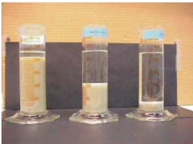
Figure 3-9. The salinity of the water affects the colloid generation. The experiment shows different degrees of sedimentation of bentonite clay dependent of the ion content in the water. The experimental conditions: Dry bentonite, 10 g/250 ml in contact with 0.01, 0.1 and 1 M solution at 20°C after 1.5 weeks.
