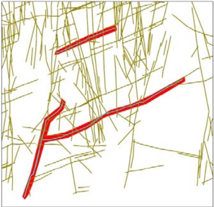
Figure 2-11. Illustration of linkage on the fracture traces from outcrop ASM100235. a) The entire network, b) detail of the reconnected network. c) highlighting, in red, of 3 reconnected traces and d) corresponding original segmented traces.
