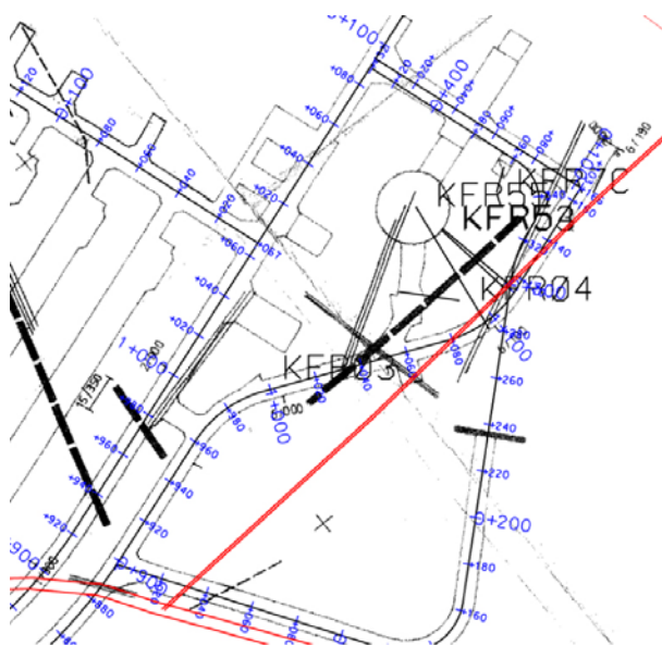
A8-6. A plan view showing the position of ZFMNE0870B in the overview drawing of the tunnel mapping (black dashed line in the centre of the figure) and the surface trace of the zone (offset parallel red line).
