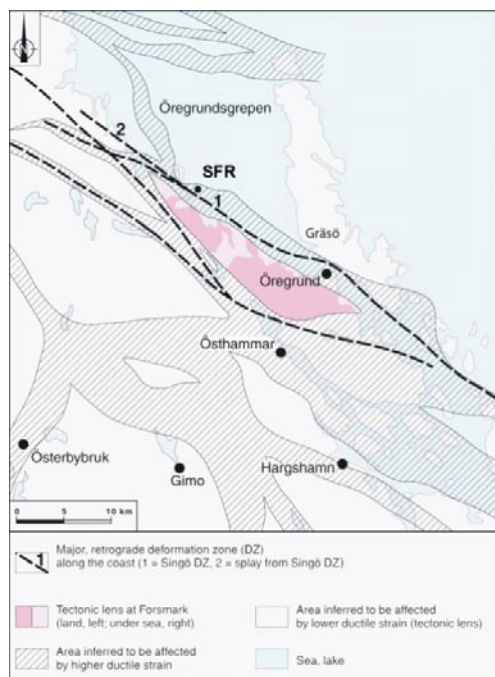
Figure 1-1. Map showing the structural framework in the Forsmark area with ductile high-strain belts that anastomose around tectonic lenses of lower ductile strain. The major retrograde deformation zones surrounding the Forsmark tectonic lens are also shown. Modified after /Stephens et al. 2007/.
