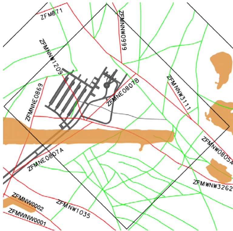
Figure 5-2. Intersection at the current ground surface of deformation zone traces with focus on the local model area. Confidence in existence: high=red, medium=green, low=grey.
