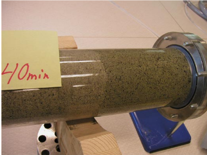
Figure 6-5. Example of the propagation of a saturation front in a 30/70 mixture (inflow 0.01 l/min, salinity 1%).
