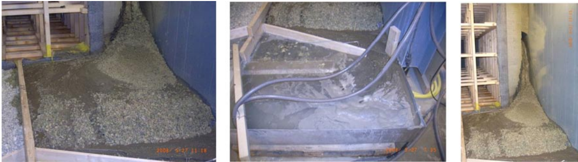
Figure 6-43. Erosion in Test 10 (2.5 l/min inflow at rear of chamber).
