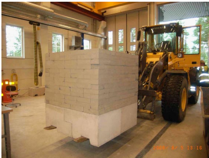
Figure 7-10. Testing of the stability of a module. Notice the larger bottom blocks and layers of differently placed and oriented blocks for increased stability.
