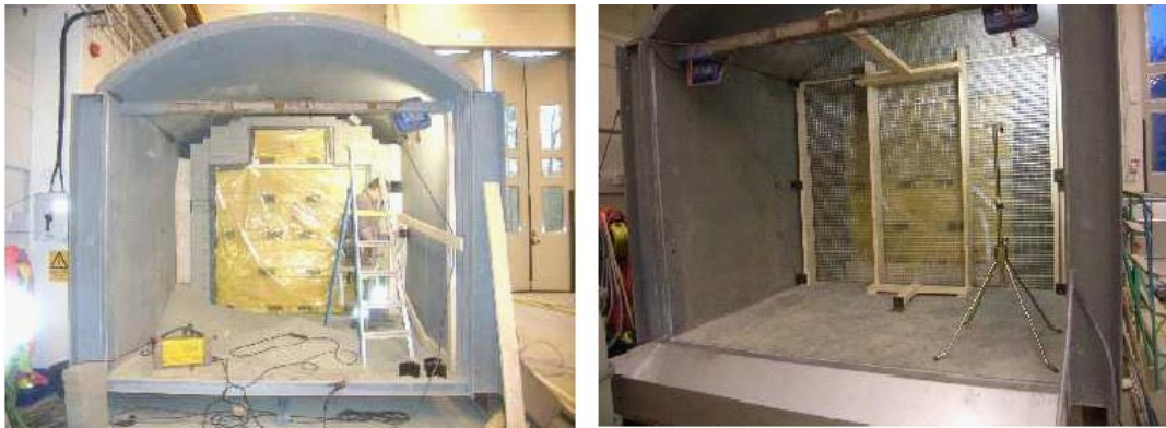
Interior of chamber during test assembly where blocks entirely surround central void
