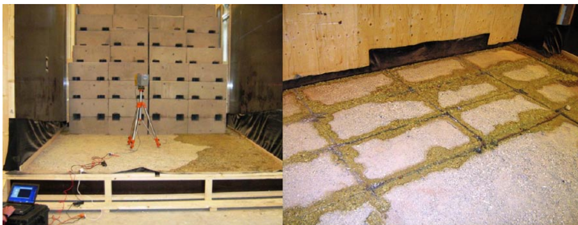
Figure 6-44. Floor material tests in the bentonite laboratory at Äspö showing on the left how water moved along sides and towards front of pellet materials and on the right how saturation had propagated underneath the blocks.
