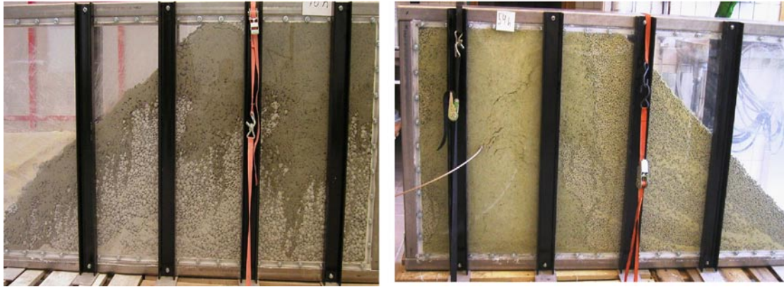
Figure 6-7. Differences in the wetting patterns of MX-80 pellets (on the left) and Cebogel pellets (on the right), 48 hours after the inflow (0.01 l/min) started. The Cebogel pellets show more uniform wetting compared to MX-80 pellets. It should be also noted that with low inflow rates the wetting also takes place upwards and radially, and not only downwards as the result of gravimetric effects.
