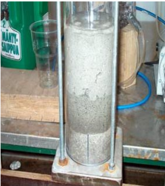
Figure 6-4. Example of the saturation tests performed by /Kuula-Väisänen et al. 2008/. The test setup consisted of a plexiglas tube with inner diameter of 0.1 m. Water was fed to the system from above until the the test cell was filled with water. After that the water pressure head was increased from 0.5 m up to 40 m (corresponding to pressure of max 0.393 MPa and \sim 4 bar). The specimens were allowed to swell in the free space above the blocks. The specimens consisted of blocks (with initial height of 50 mm) and a combination of blocks and pellets.
