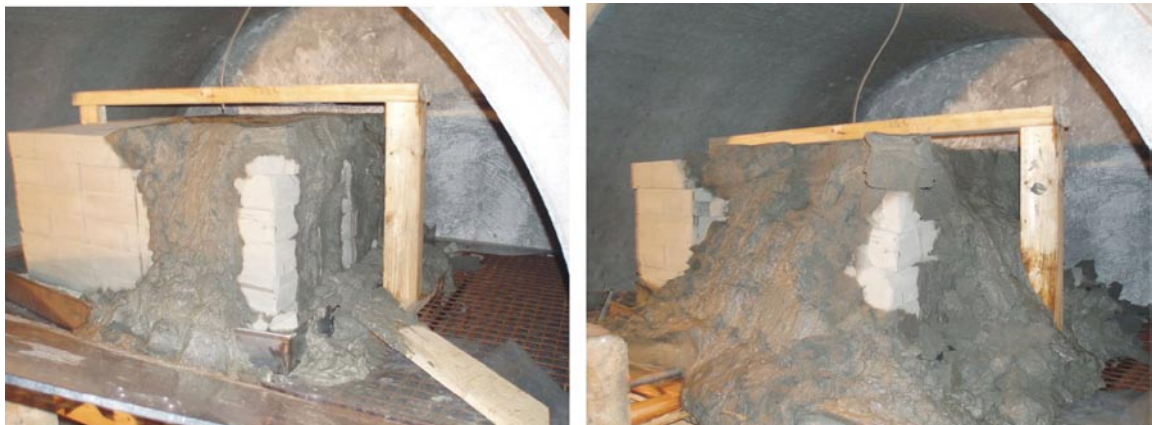
Figure 6-16. Effect of water dripping on unprotected and unsupported clay block assembly. (Water dripped from mid-point of wooden crossbars /Dixon et al. 2008a, b/).
