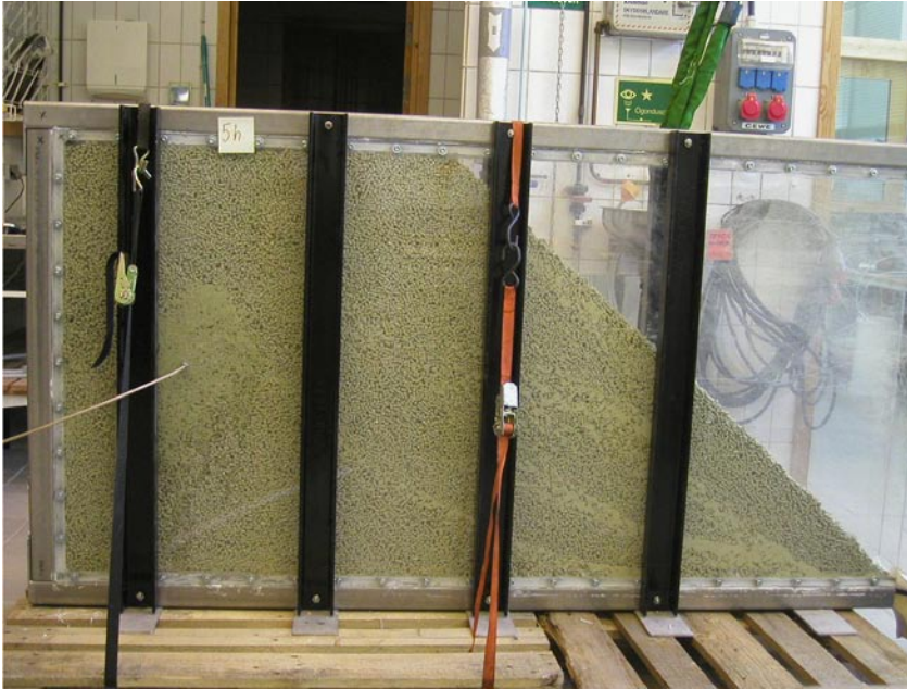
Figure 6-3. Example of large slot tests performed by /Sandén et al. 2008/ for different types of pellet materials. The test setup is simulating the pellet filled section between the backfill blocks and the rock. The artificial slot had dimensions of 2 \times 1 \times 0.1 m.
