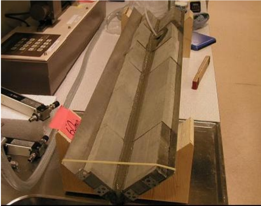
Figure 6-1. Example of the block saturation/erosion tests performed for pre-compacted Friedland-clay blocks by /Sandén et al. 2008/. In these tests a one meter long steel profile with inclination of 1° was filled with backfill blocks. A constant water flow was applied at one end and the amount of eroded material was measured in the other end.
