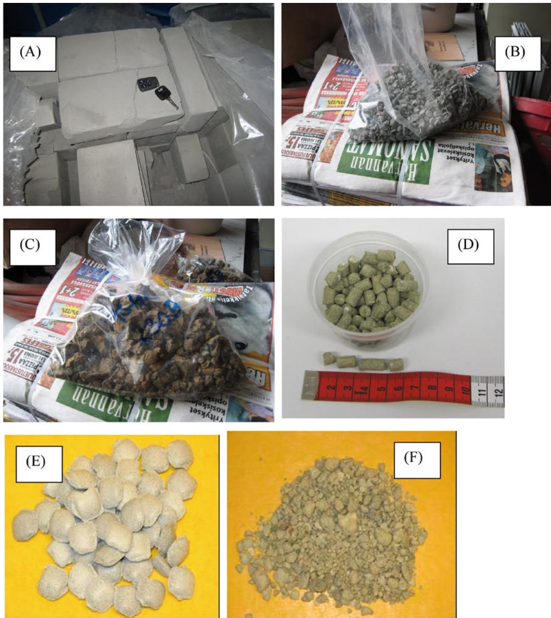
Figure 5-1. Photographs of some Baclo test materials. A) Friedland clay blocks produced in Bjuv, B) Friedland-clay granules, C) Asha 230 B bentonite before homogenisation by mixing, D) Cebogel pellets and E) MX-80 pellets, F) Minelco granules.
