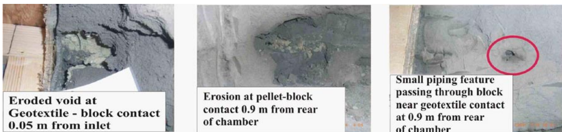
Figure 6-37. Piping features initially present along pellet-block interface in Test 12 /Dixon et al. 2008c/.
