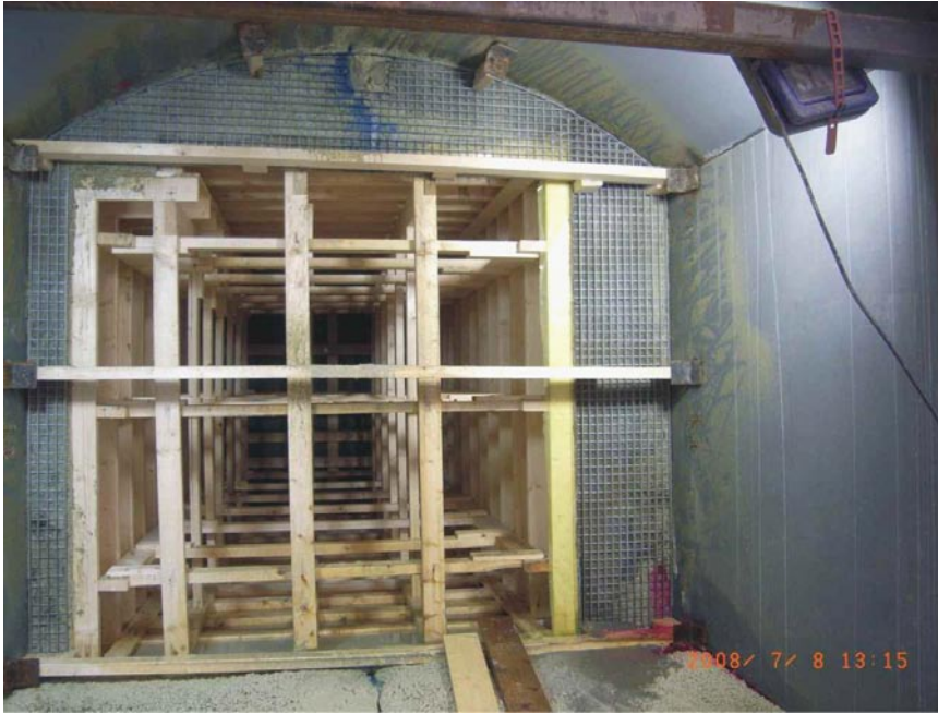
Figure 6-40. Assembly 6 (Tests 11 and 12) at the end of testing Test 12. (Note blue tracer exiting a crown of chamber and pink tracer in lower right corner.)
