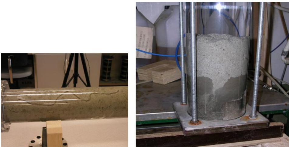
Figure 6-6. Formation of preferential flow paths in MX-80 pellets /see Sandén et al. 2008/ and in combination structure consisting of Friedland clay blocks and MX-80 pellets /see Kuula-Väisänen et al. 2008/.
