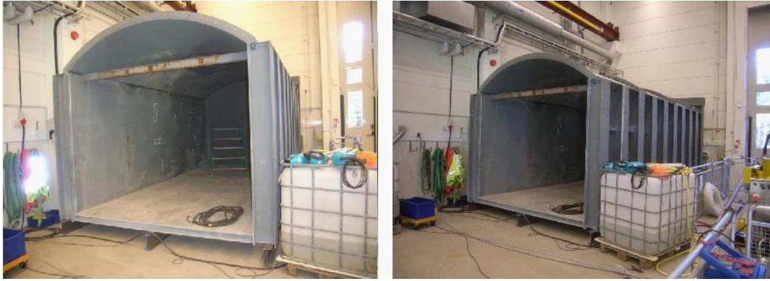
Interior and side view of 1/2-Scale chamber, note tanks used to supply water and hold outflow
