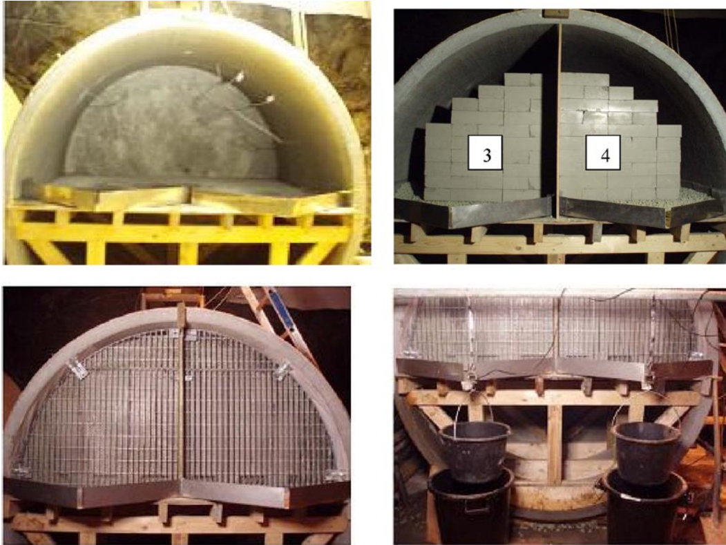
Figure 6-15. Photographs showing assembly of 1/12 scale tests. (Note water inflow lines in upper left photograph, water collection buckets have load cells measuring mass of material entering the collection system.)
