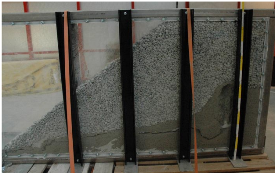
Figure 6-8. Formation of preferential water pathway through MX-80 pellets when the inflow was 1 l/min, /see Sandén et al. 2008/. Note also the more gravimetrically-influenced flow pattern compared to that observed at lower inflow rates ( \leq 0.1 l/min).
