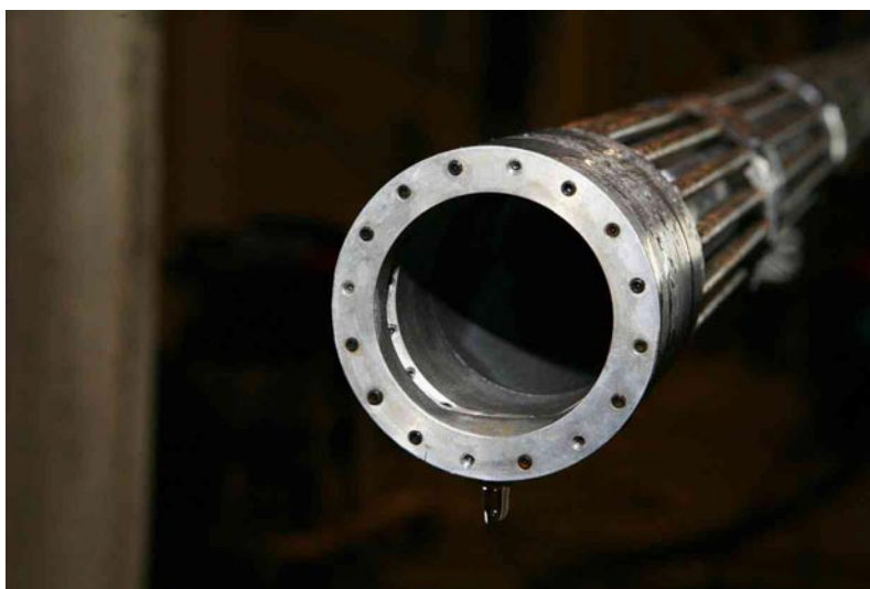
Figure 7-11. The picture shows the nozzle of the tube for blowing pellets with holes for adding water for reducing generation of dust.
