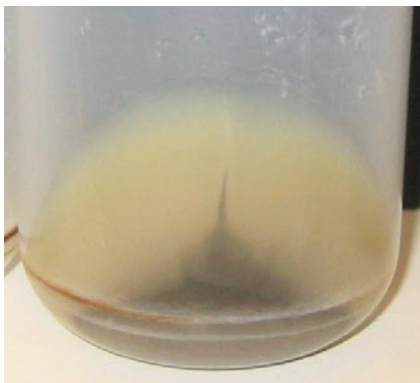
Figure 4-4. Remaining solid phases after removal of water from a MX-80 suspension.
