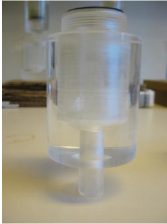
Figure 4-2. The filtration cell. Figure 4-3. Parts included in the filtration cell.
