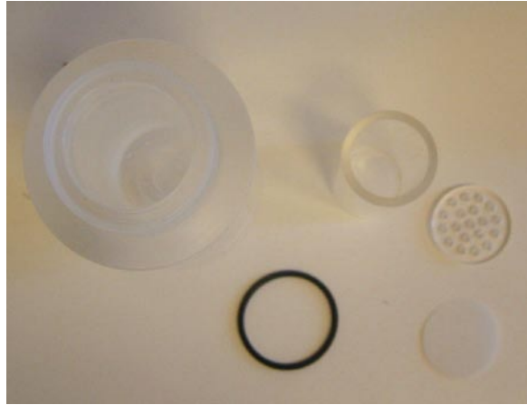
Figure 4-2. The filtration cell. Figure 4-3. Parts included in the filtration cell.
