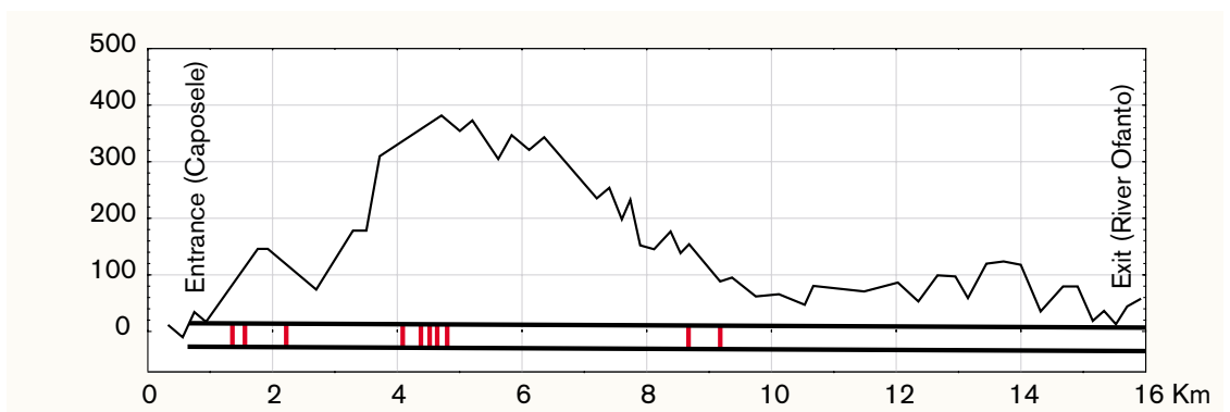
Figure 3-5. Longitudinal profile of the Pavoncelli tunnel in Italy and location of the most important damages (c.f. Table 3-1) induced by the November 23, 1980 M=6.8 earthquake. Strong tectonic stresses developed during the earthquake and some faults were reactivated /Revised after Cotecchia et al, 1986/.
