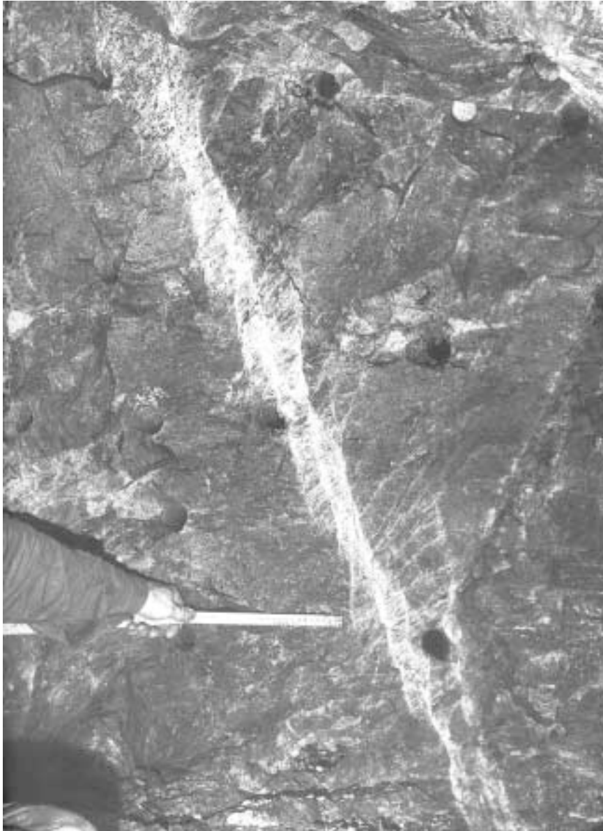
Figure 3-17. Photo on a typical “shear rupture” as suggested by /Ortlepp, 1997/. The photo is from Rupture # 18, West Claims. /Segall and Pollard, 1980/ later used the findings from the 70’ies in their famous work.
