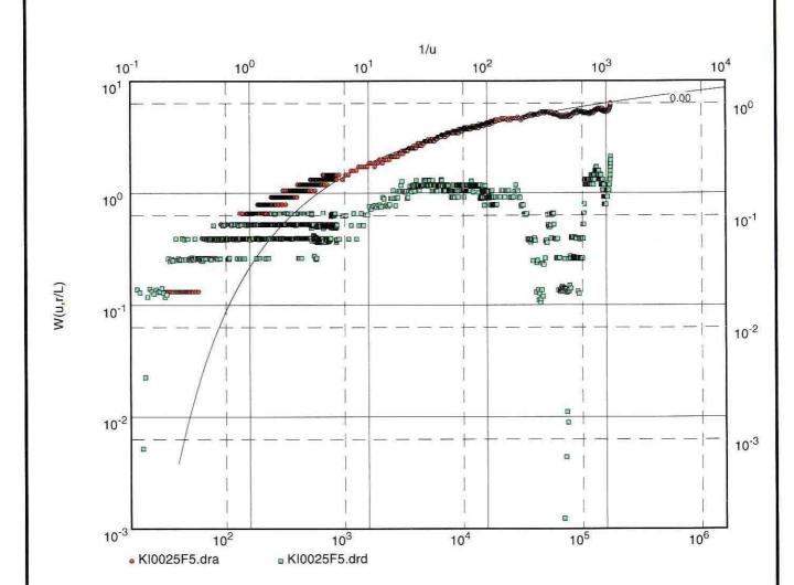
Transmissivity [m<sup>2</sup>/s]: 2.59 x 10<sup>-5</sup>
