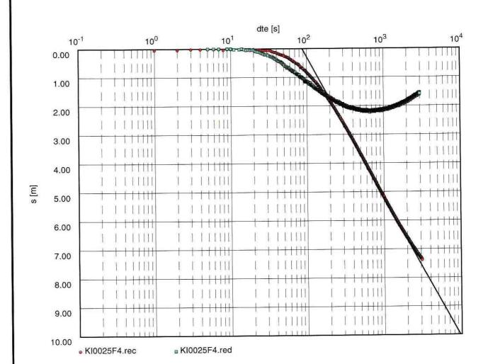
Transmissivity [m<sup>2</sup>/s]: 9.63 x 10<sup>-7</sup>
