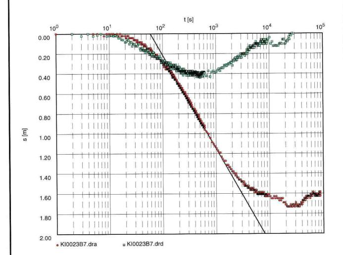
Transmissivity [m<sup>2</sup>/s]: 1.12 x 10<sup>-6</sup>
