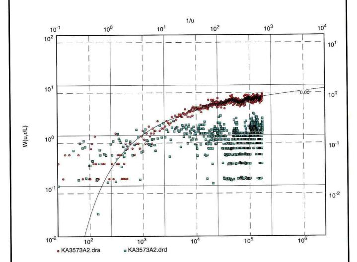
Transmissivity [m<sup>2</sup>/s]: 2.91 x 10<sup>-5</sup>
