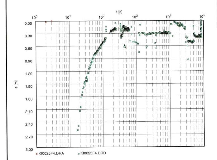
Transmissivity [m<sup>2</sup>/s]: 1.54 x 10<sup>-6</sup>
