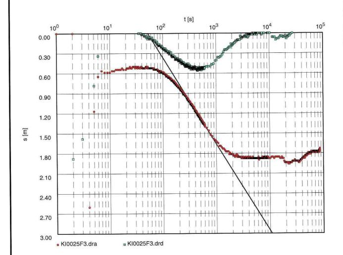
Transmissivity [m<sup>2</sup>/s]: 8.11 x 10<sup>-7</sup>
