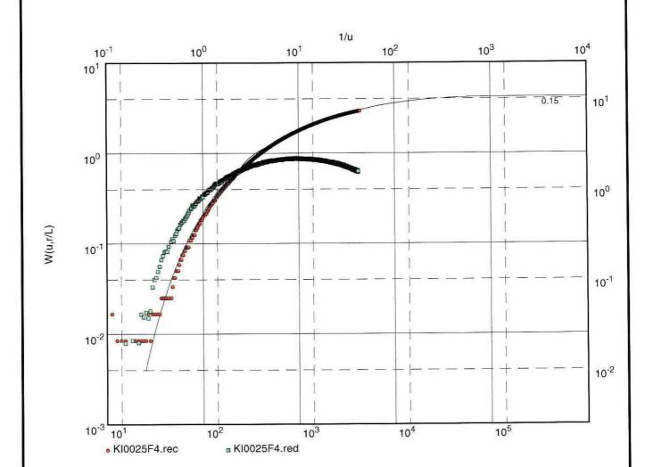
Transmissivity [m<sup>2</sup>/s]: 8.17 x 10<sup>-7</sup>
