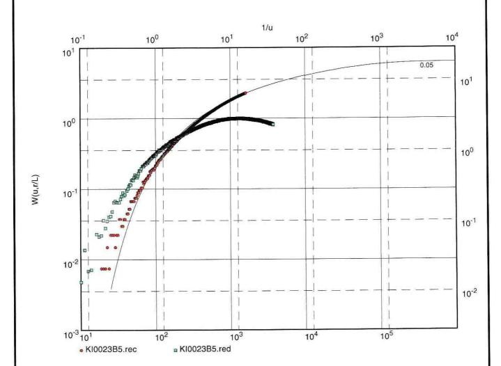
Transmissivity [m<sup>2</sup>/s]: 7.28 x 10<sup>-7</sup>
