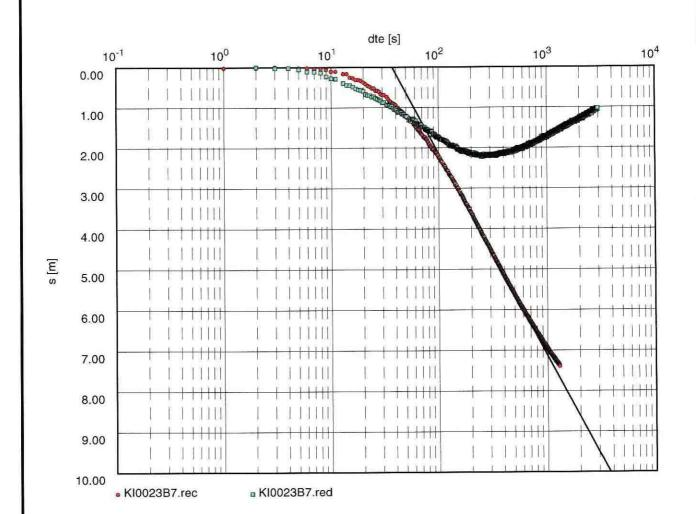
Transmissivity [m<sup>2</sup>/s]: 9.45 x 10<sup>-7</sup>
