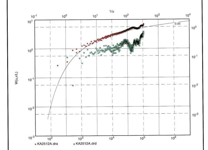
Transmissivity [m<sup>2</sup>/s]: 3.08 x 10<sup>-5</sup>
