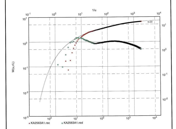
Transmissivity [m<sup>2</sup>/s]: 1.02 x 10<sup>-6</sup>
