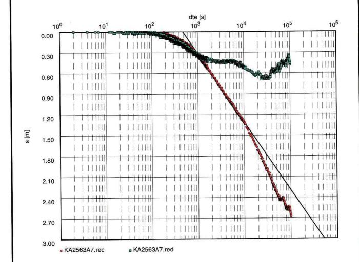
Transmissivity [m<sup>2</sup>/s]: 2.76 x 10<sup>-5</sup>
