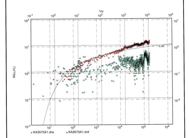
Transmissivity [m<sup>2</sup>/s]: 4.89 x 10<sup>-5</sup>
