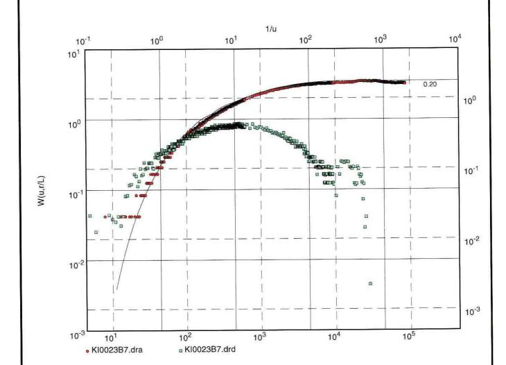
Transmissivity [m<sup>2</sup>/s]: 9.12 x 10<sup>-7</sup>
