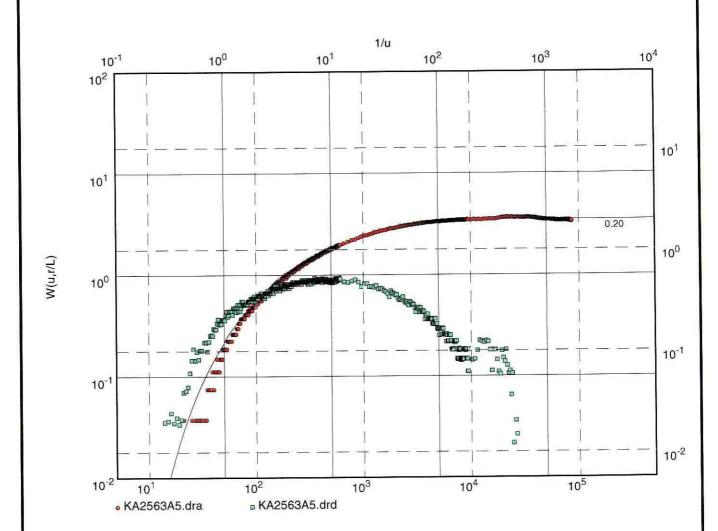
Transmissivity [m<sup>2</sup>/s]: 8.13 x 10<sup>-7</sup>
