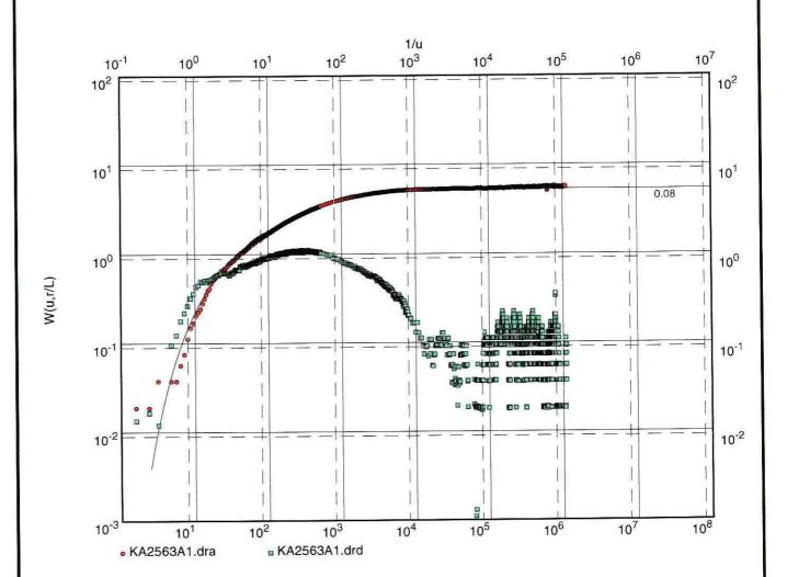
Transmissivity [m<sup>2</sup>/s]: 1.22 x 10<sup>-6</sup>
