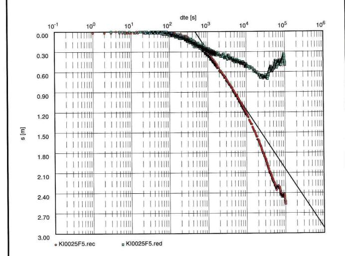
Transmissivity [m<sup>2</sup>/s]: 3.10 x 10<sup>-5</sup>
