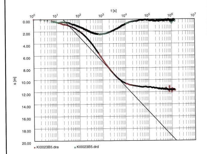
Transmissivity [m<sup>2</sup>/s]: 7.72 x 10<sup>-7</sup>
