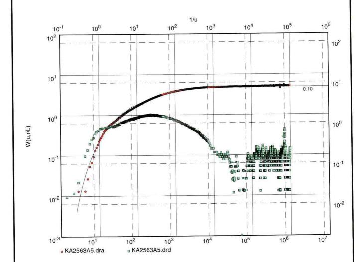
Transmissivity [m<sup>2</sup>/s]: 8.68 x 10<sup>-7</sup>
