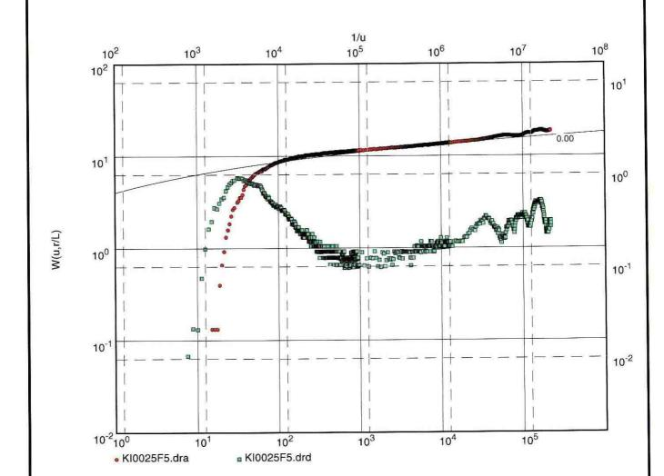
Transmissivity [m<sup>2</sup>/s]: 3.46 x 10<sup>-5</sup>
