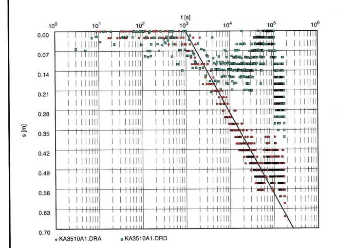
Transmissivity [m<sup>2</sup>/s]: 3.18 x 10<sup>-5</sup>
