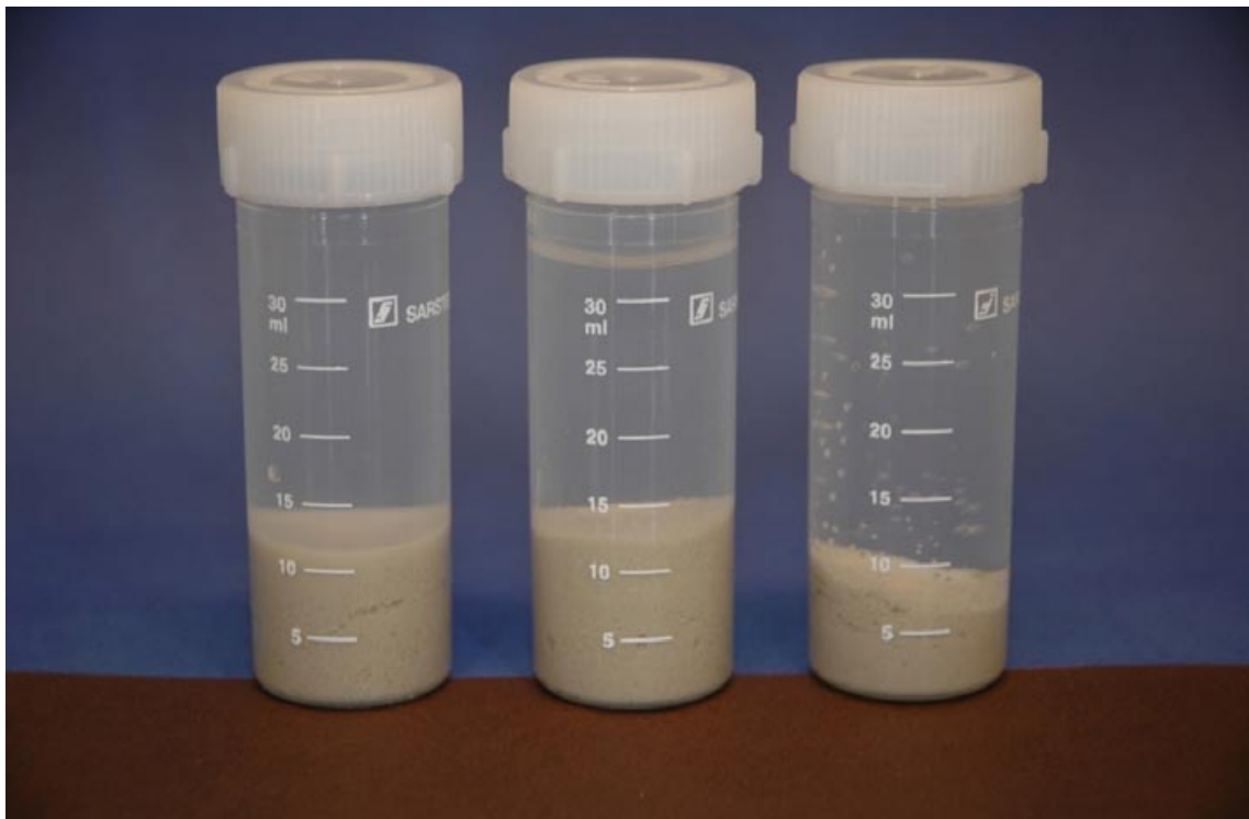
Figure 3-42. Swelling of Wy-Ca with the dry mass 2.47 g from (left to right) powder, dry compacted sample and saturated sample.
