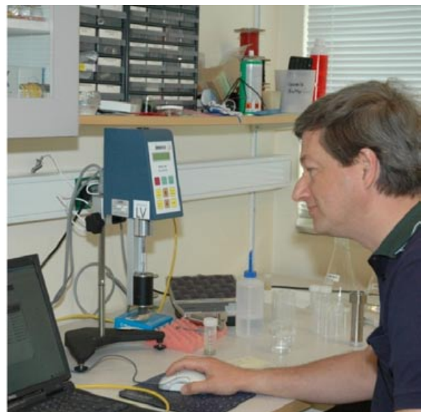
Figure 3-7. Test principles for and a picture of the Brookfield viscometer. The spindle rotates inside the cup filled with the bentonite slurry and the torque and the torsional angle are measured.
