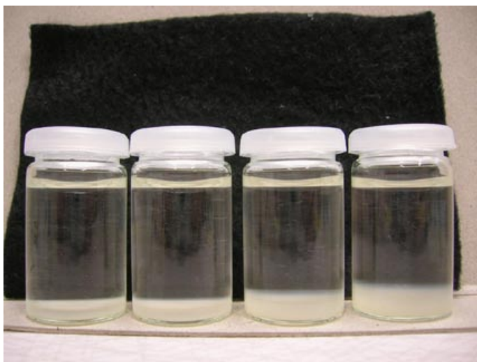
Figure 7-14. From left to right: 2.5, 5, 10, and 15 mM NaCl in the initial solution (Samples 29, 35, 36 and 37). Initially 0.5 mM CaCl 2 .
