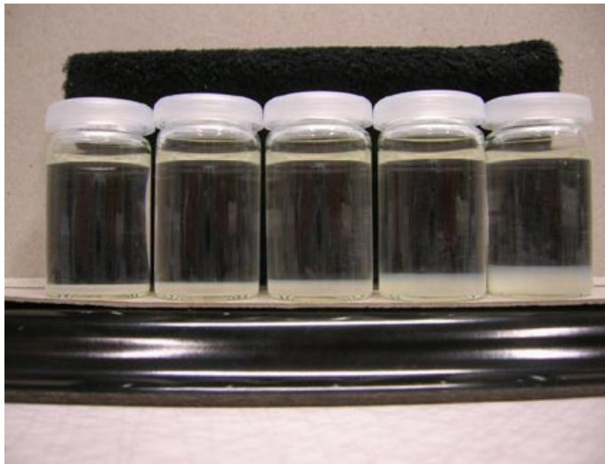
Figure 7-20. Samples with 0.4 mM CaCl 2 in equilibrium solution. From left to right: 2, 4, 6, 8, and 10 mM NaCl in the equilibrium solution (samples 49, 50, 51, 52, and 53).
