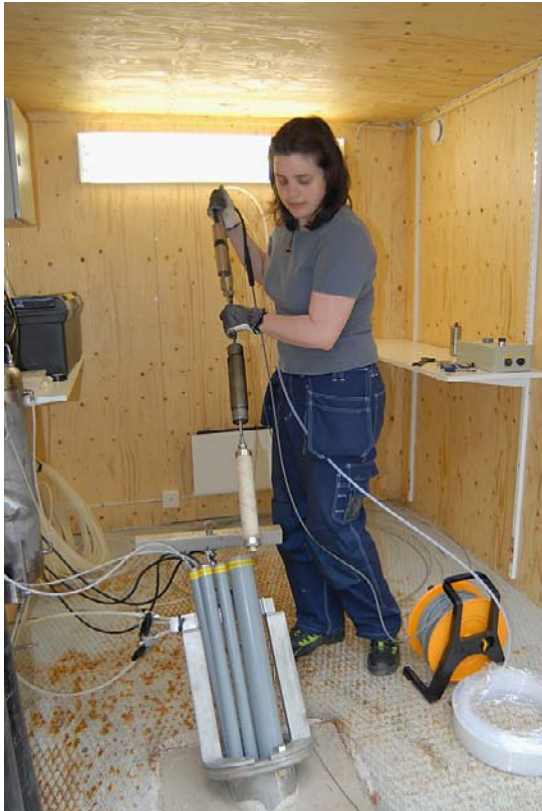
Figure 3-3. Lowering of equipment in the water stand-pipe in order to pump water from the borehole section. From the bottom; filter, small inflatable packer and pump.
