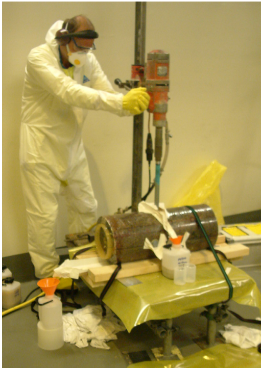
Drilling of sample cores from matrix rock surrounding the test section in the small diameter extension borehole.
