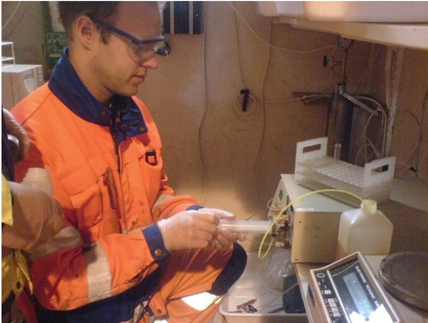
Injection of tracer in fracture
