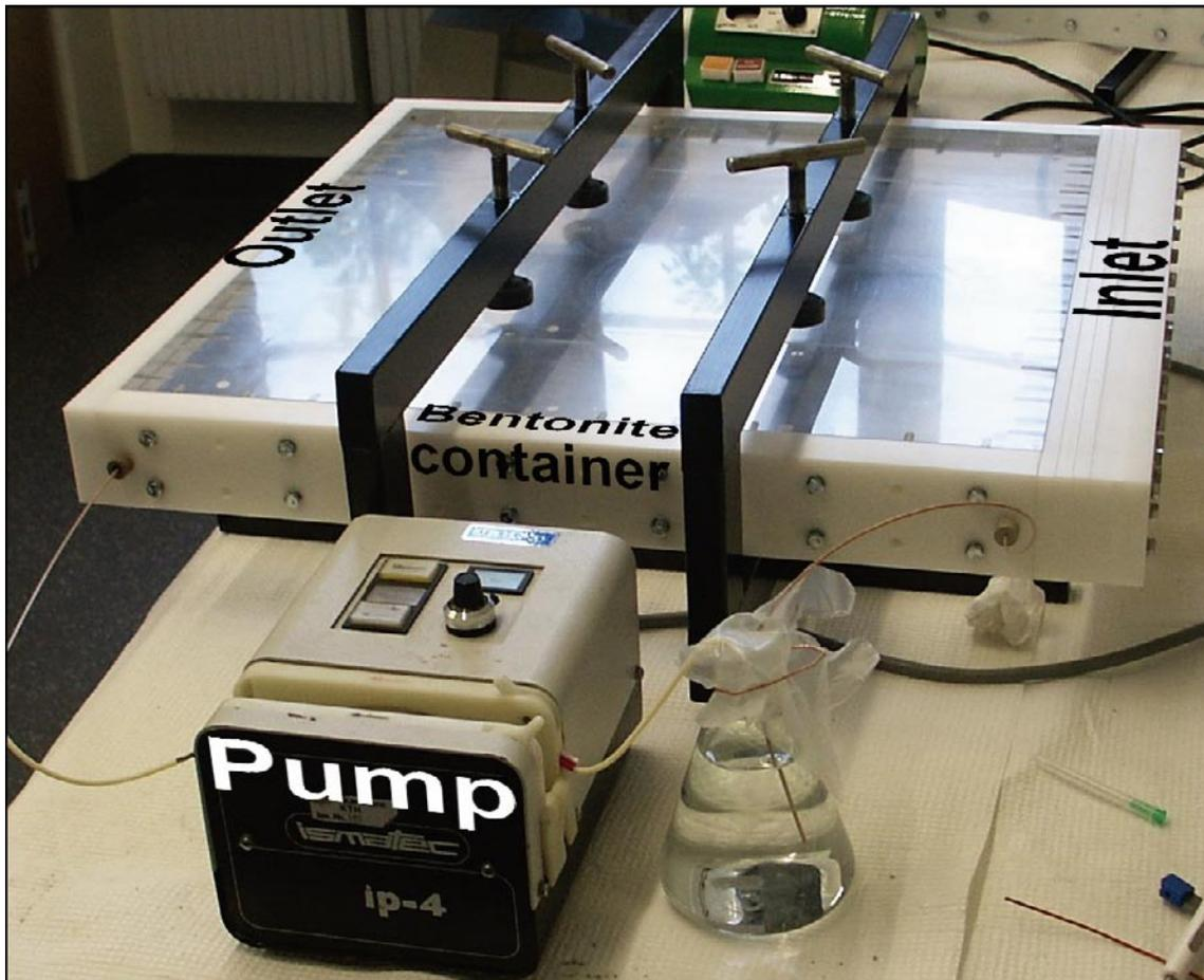
*Figure 8-2. Artificial fracture. The bentonite is being water saturated.*
