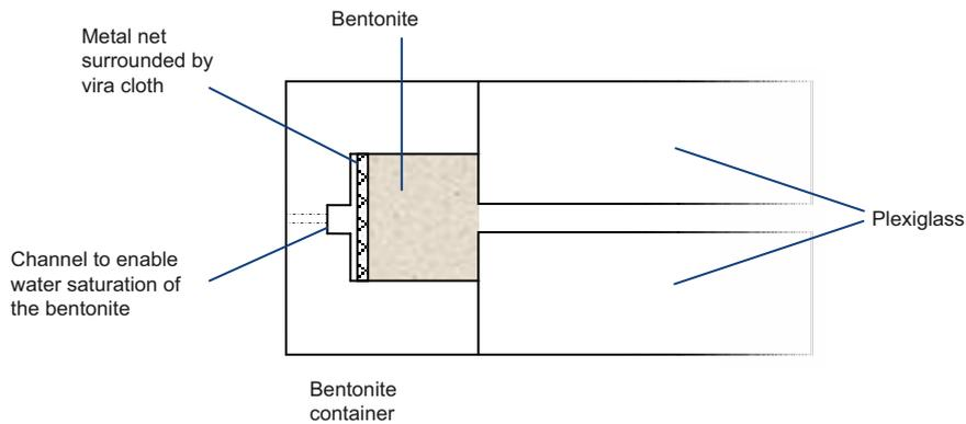
**Figure 8-3.** Enlargement of the bentonite container.
