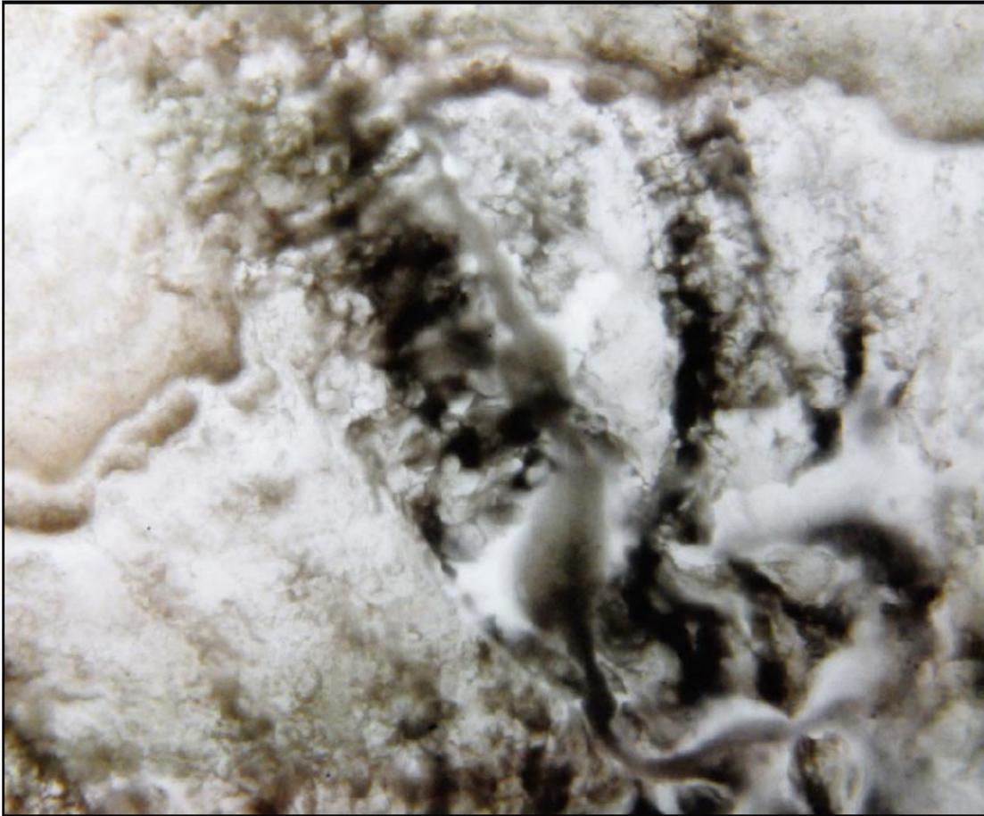
*Figure 8-7. A dark rim was observed at the border where the clay seems to change phase from gel to sol.*
