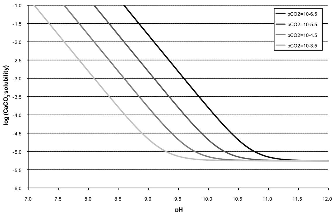
**Figure 5-1.** The solubility of  $\text{CaCO}_3$  as a function of pH. The data is modeled with Medusa Chemical Diagrams, see also Appendix I.
