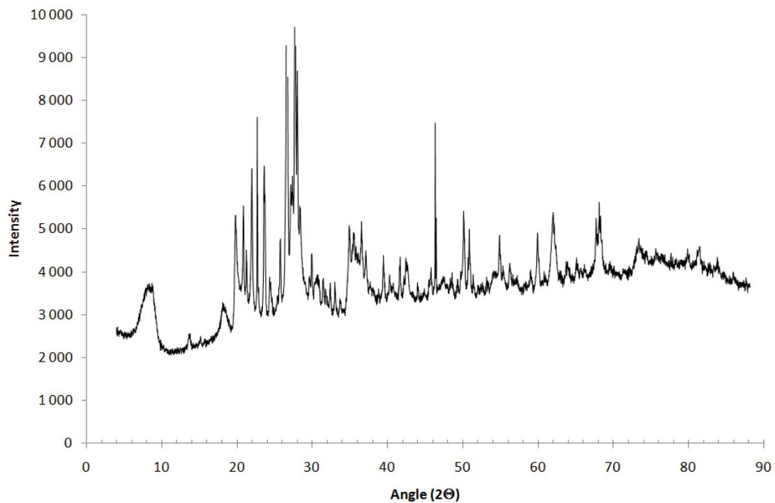
**Figure 8-9.** XRD spectra of the dark rim that was found in the experiment with the artificial fracture.
