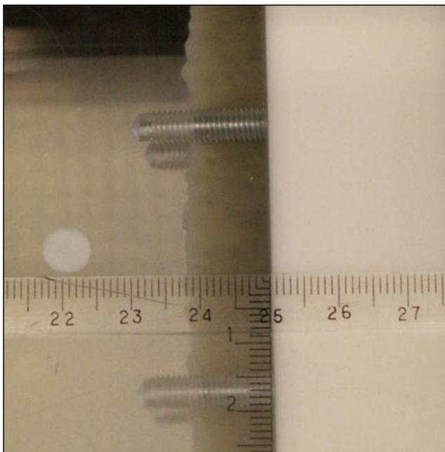
**Figure 8-4.** After water saturation the bentonite had expanded 12–14 mm into the fracture.
