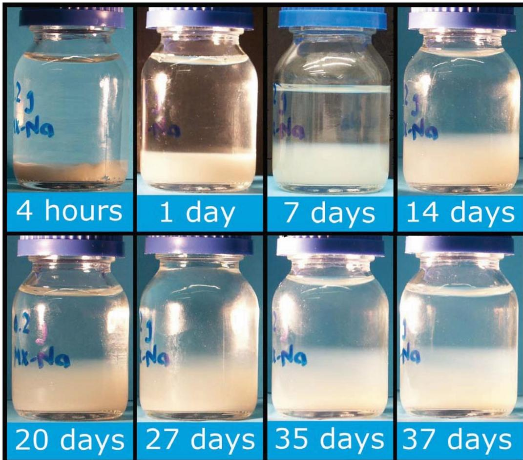
**Figure 6-1.** Swelling of sodium montmorillonite. The difference in water volume is due to sampling for measuring colloid concentrations. At intervals the water was replenished.
