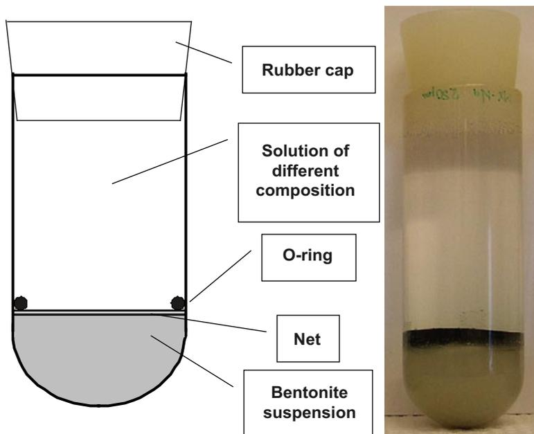
Figure 5-2. Experimental set-up for the test tube studies.
