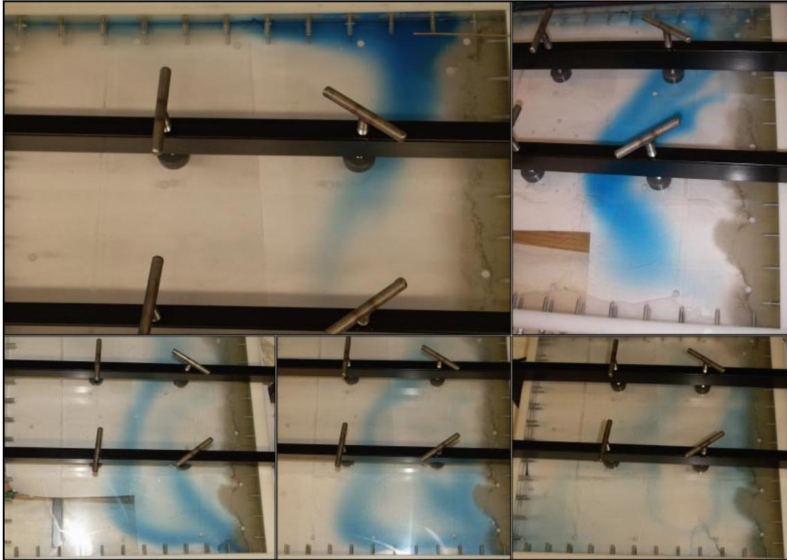
**Figure 8-10.** To see how the flow path looked like a dye was added to the inlet solution. As can be seen the flow path varies a lot with time and is not evenly distributed.
