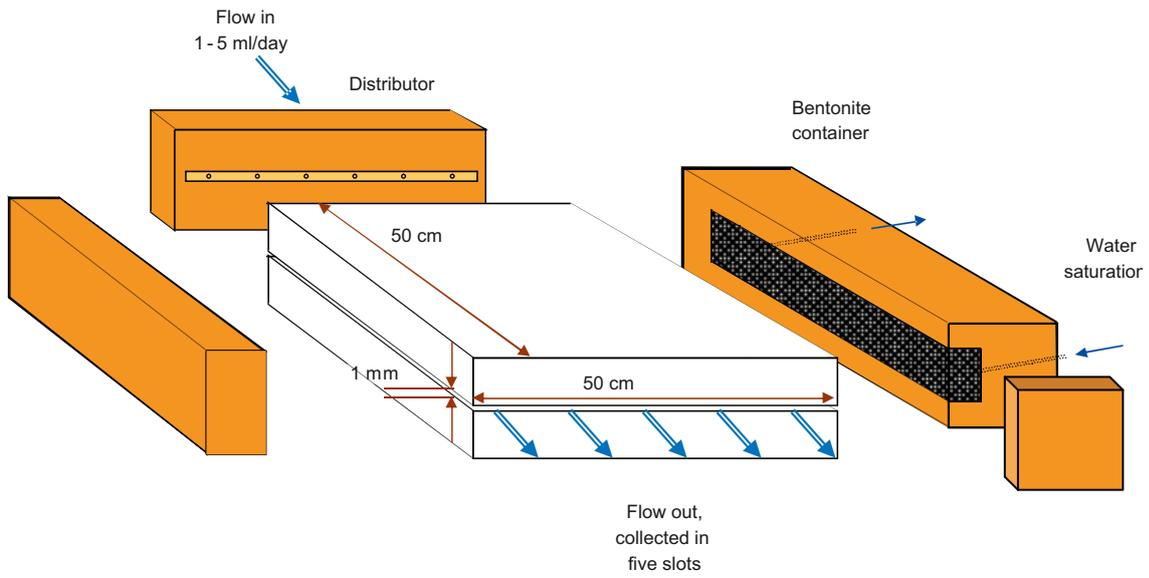
*Figure 8-1. Principal drawing of the set-up for the experiments in the artificial fracture.*
