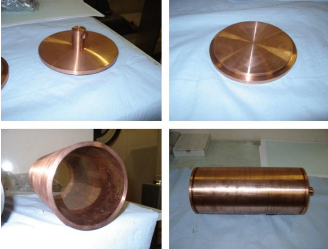
Figure 3-5. Copper components of miniature canisters.
