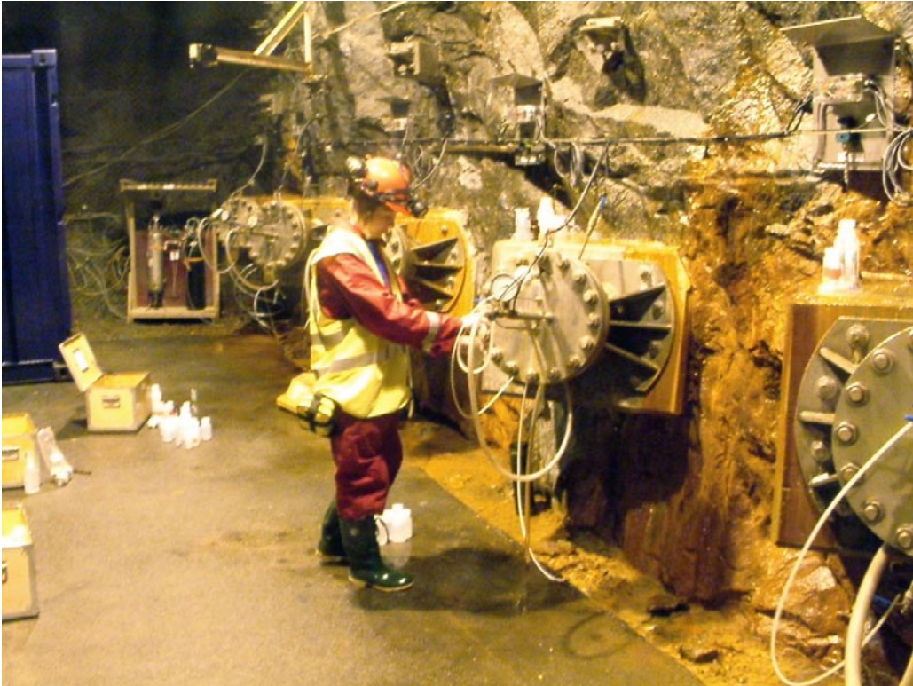
Figure 5-6. Complete Minican experimental installation at Äspö Hard Rock Laboratory, showing water samples being collected for analysis. The experiments are installed in five separate boreholes, with a control room located in an ISO container at the rear left hand corner of the tunnel.
