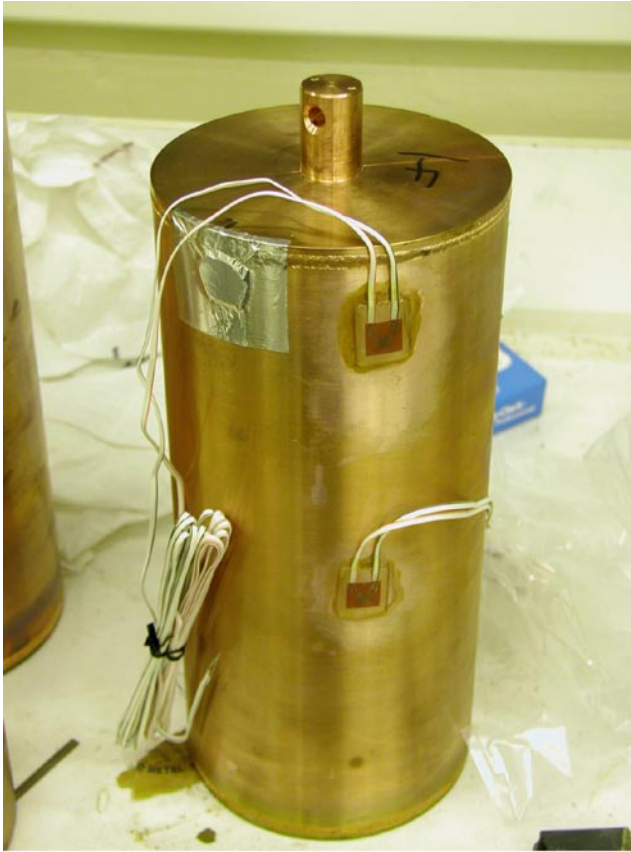
Figure 4-3. Strain gauges mounted on model canister.
