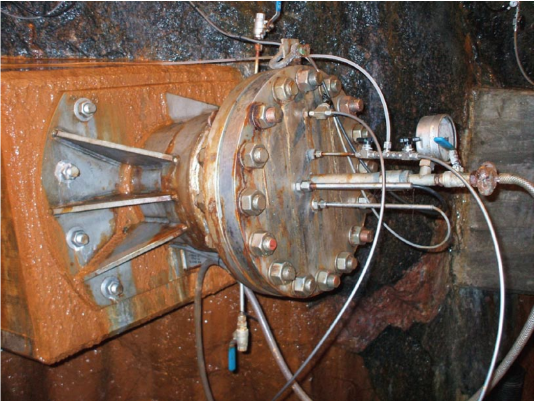
Figure 5-7. Brown slime around experiment on rock face around borehole.
