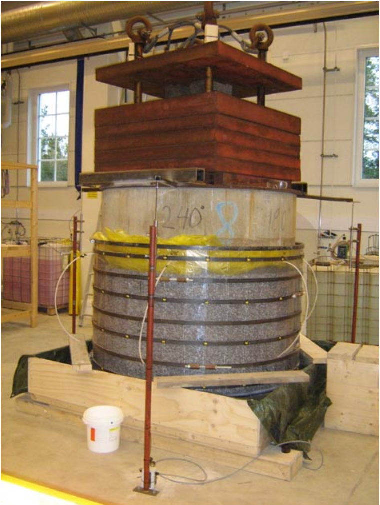
Figure 5-2. Buffer test with regards to influence by water inflow.
