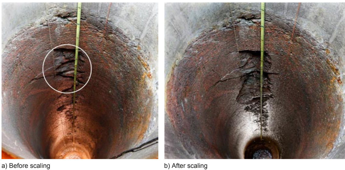
Figure 2-4. Photographs of the north-east-side of heater hole KQ0048G04, the wetter hole in the third test before a) and after b) scaling of the borehole wall.
