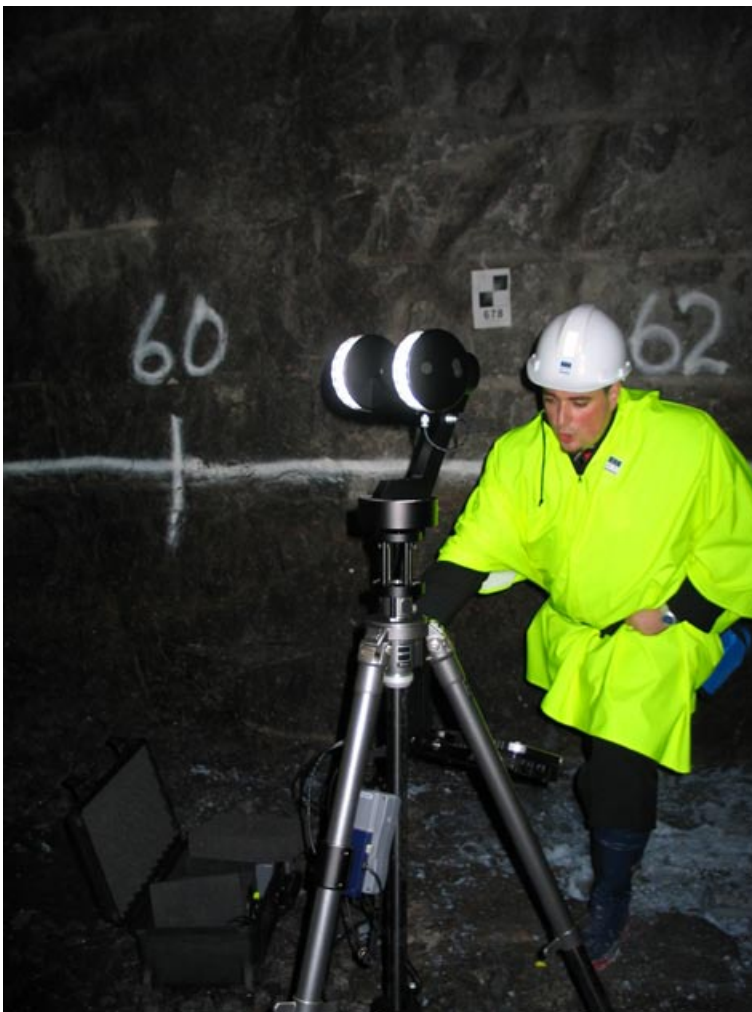
Figure 2-2. Tests with new camera equipment (SheronCam HDR) in the Tass-tunnel.
