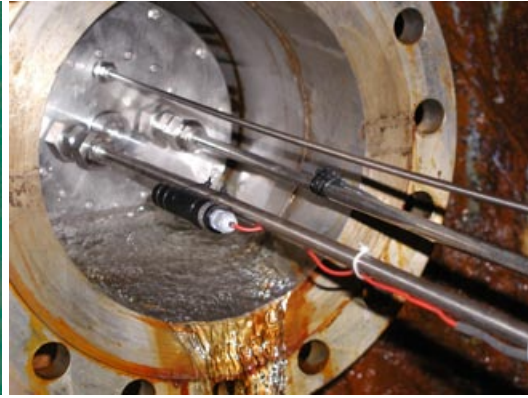
Figure 4-28. Installation of model canister experiment.
