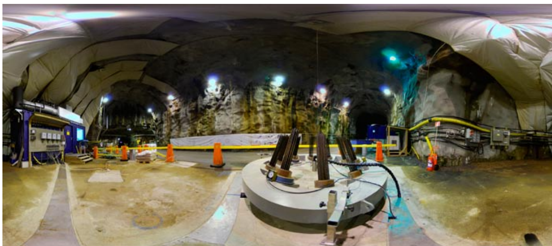
Figure 4-24. Panorama of the Large Scale Gas Injection Test at the –420 m level in Äspö HRL.
