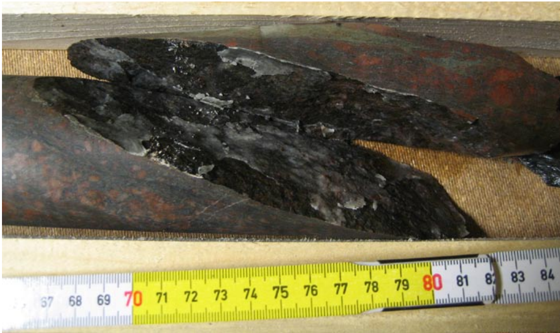
Figure 3-9. Intersected fracture with fracture filling material obtained during drilling for analysis of DNA and RNA in biofilms in the KA362A6 borehole.
