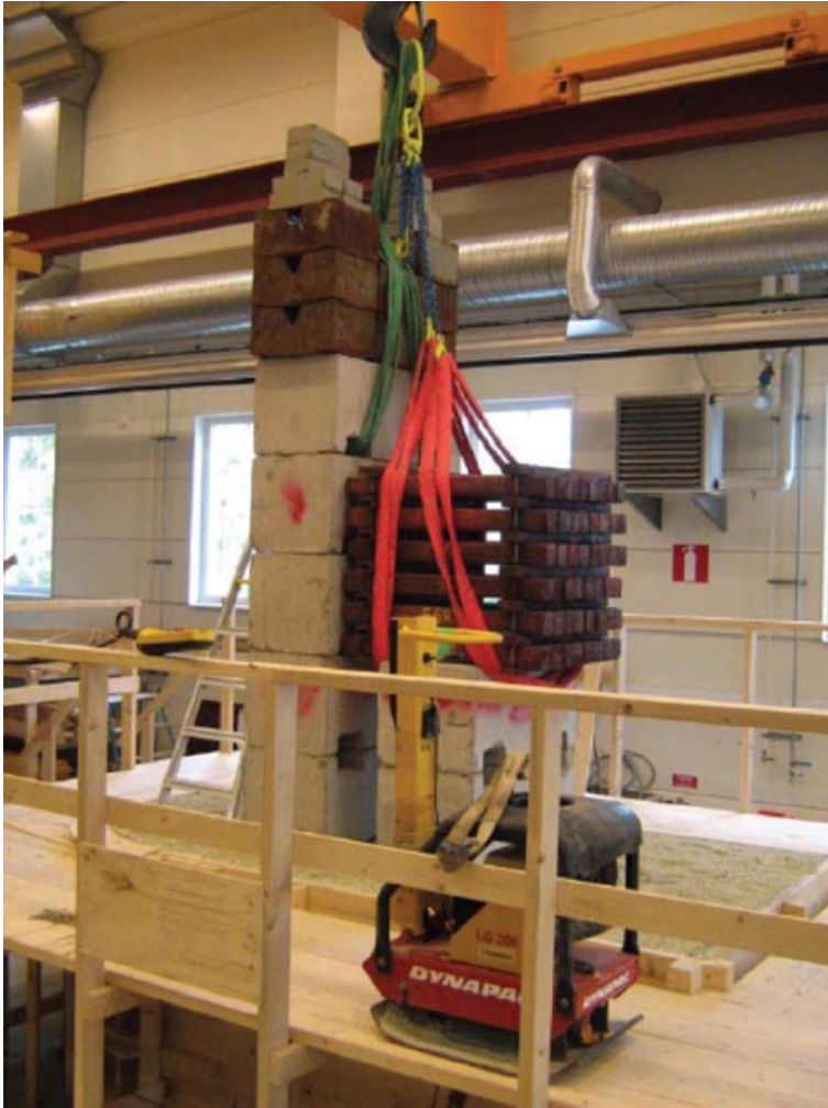
Figure 5-3. Stacking tests on backfilled bevel and buffer.
