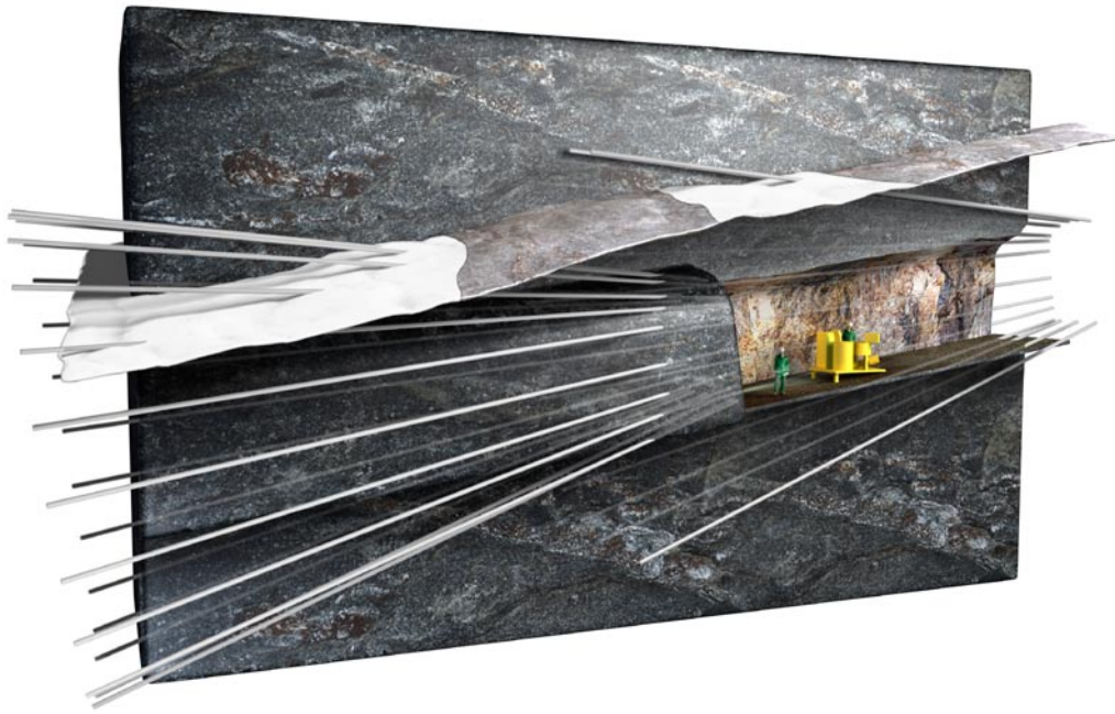
Figure 7-1. An illustration of a grouting fan in the ramp, where the holes are angled as much as possible to cross the gently dipping water-bearing fracture zones.
