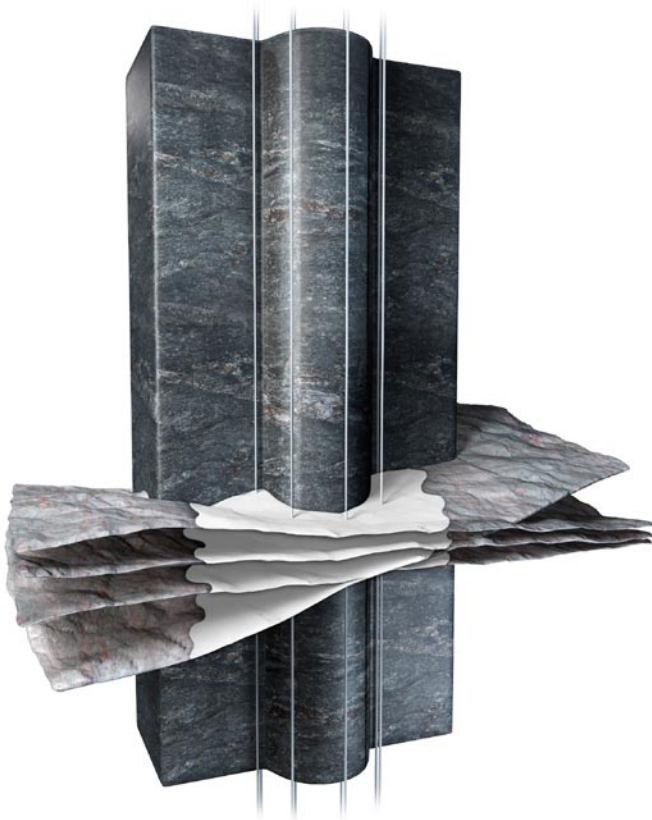
Figure 7-3. Illustration of a possible pre-grouting borehole configuration for the 6-m-diameter liftshaft and 3-m-diameter ventilation shafts.
