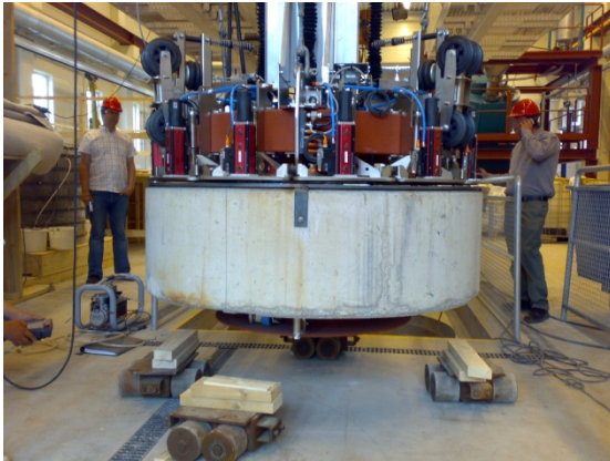
Lifting of test buffer blocks in full scale
