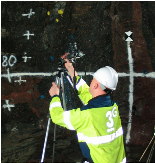
Demonstration of the JointMetrix-3D photogrammetric system by using an ordinary digital camera mounted on a tripod.
