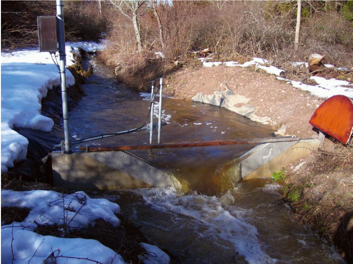
Figure 4-6. Discharge station PSM000365 during spring flood in recession on April 6, 2006. At this time the flow is 0.15\text{m}^3/\text{s} (9,000 L/min). A 45^\circ V-notch weir made of concrete with impermeable geotextile upstream. The pipes in the middle of the stream are holding the pressure gauge and the combined temperature/electrical conductivity sensor. The pipe to the left is holding the data logger and GSM transmitter.
