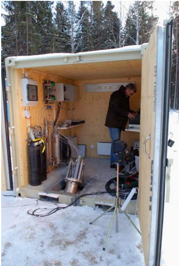
Figure 4-10. Interior of container used as borehole collar shelter after installation of groundwater level monitoring equipment in a core drilled borehole of telescopic type.
