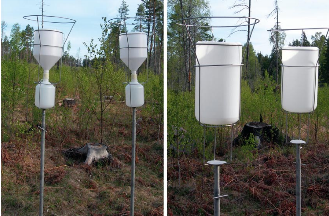
Figure 4-15. Sample collectors for precipitation at Äspö. The two collectors to the left are for rain and the ones in the picture to the right are for snow. The construction aims to prevent evaporation.
