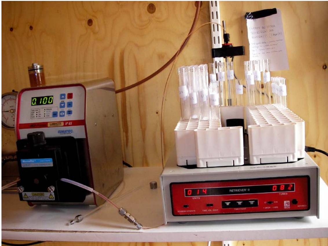
Figure 3-3. Peristaltic pump and fraction sampling equipment used at the injection hole KLX15A.
