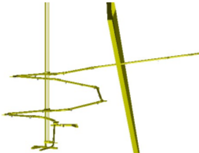
Figure 2-6. Location of deformation zone EW-3 in relation to the tunnels, iso view.
