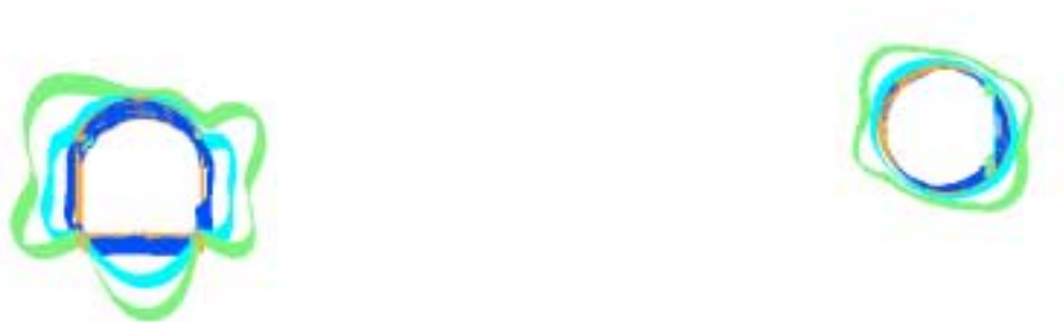
Figure 4-26. Isosurfaces of the minor principal compressive stress at magnitudes of 0 MPa (dark blue), 3 MPa (light blue) and 6 MPa (green). TASF to the left and the TBM-tunnel to the right.
