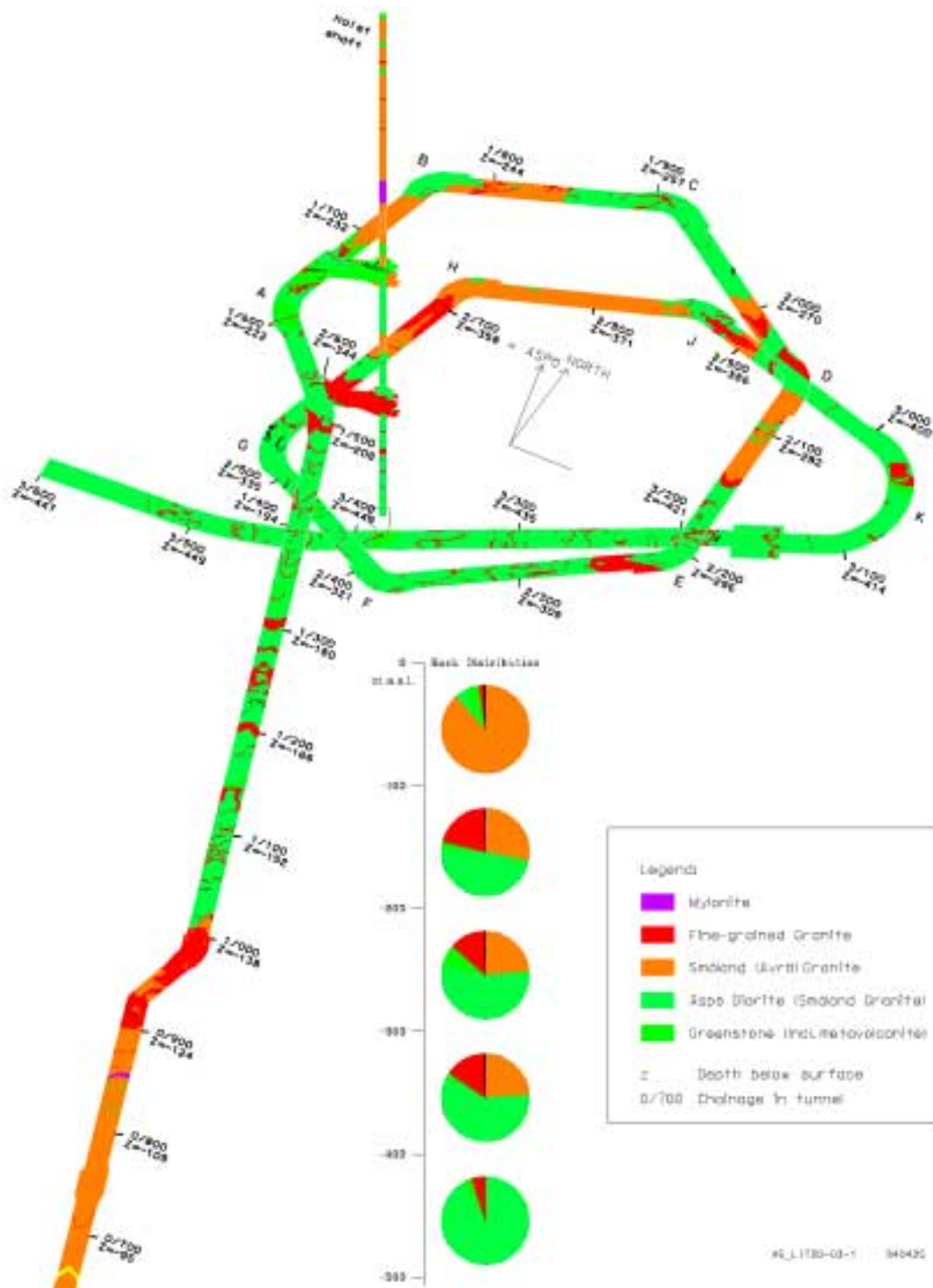
Figure 2-2. Compilation of the approximate rock distribution at different levels of the tunnel.
