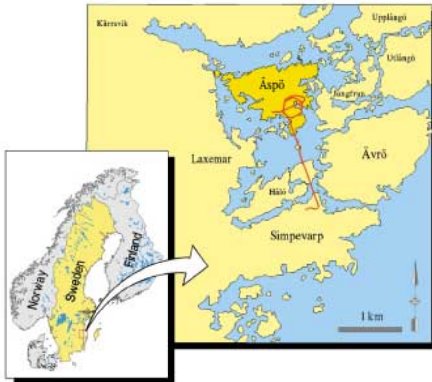
Figure 2-1. Geographical location of Äspö HRL. The red line is the planar view of the tunnel layout.
