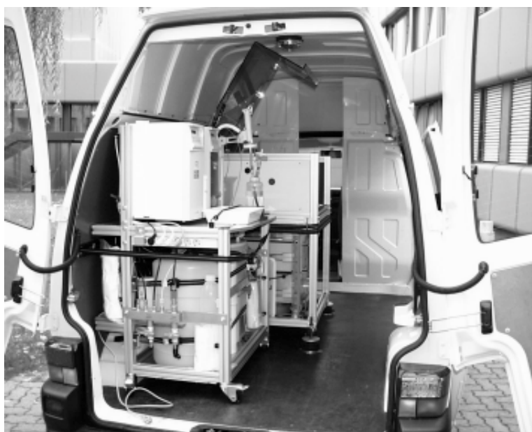
Figure 3-6 The equipment for Laser-induced Breakdown-Detection (LIBD) of colloids is installed in a van in order to allow mobility and on-line measurements at boreholes.
