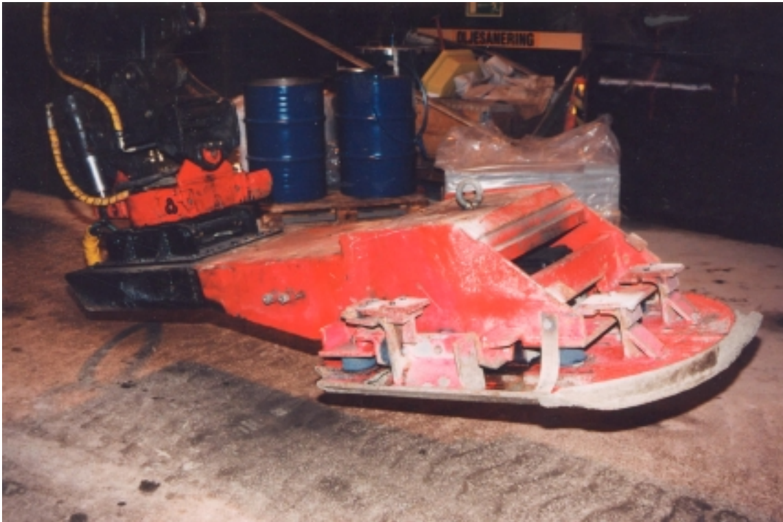
Figure 6-3. Photo of the slope compactor
