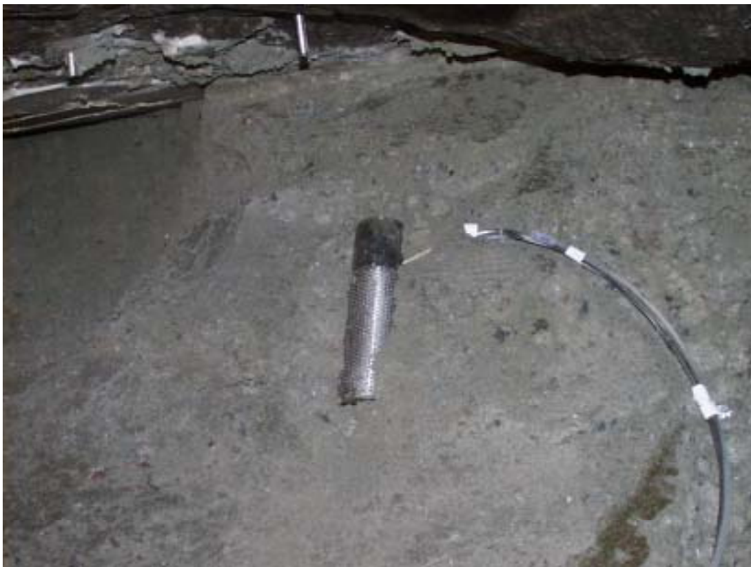
Figure 5: DPP sensor installed perpendicular to layer
