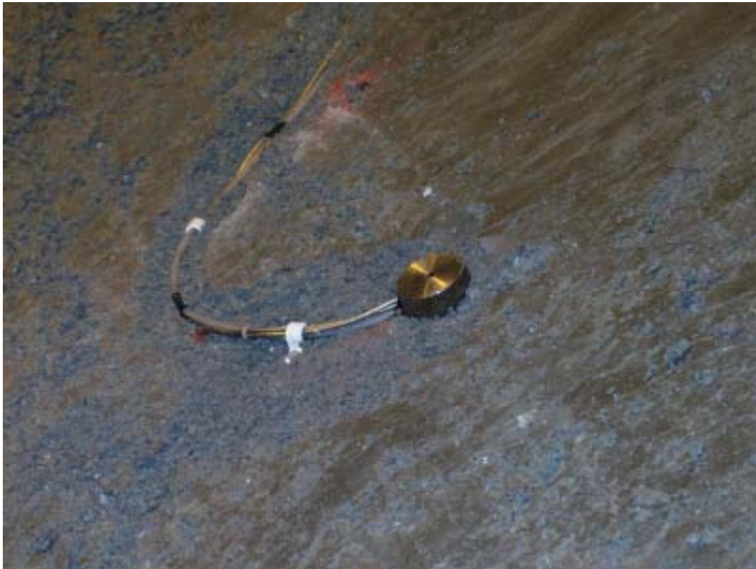
Figure 5: DPP sensor installed perpendicular to layer
