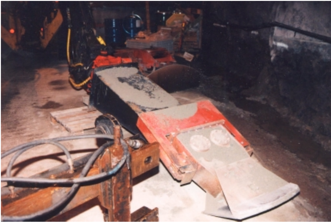
Figure 6-5. The roof compactor
