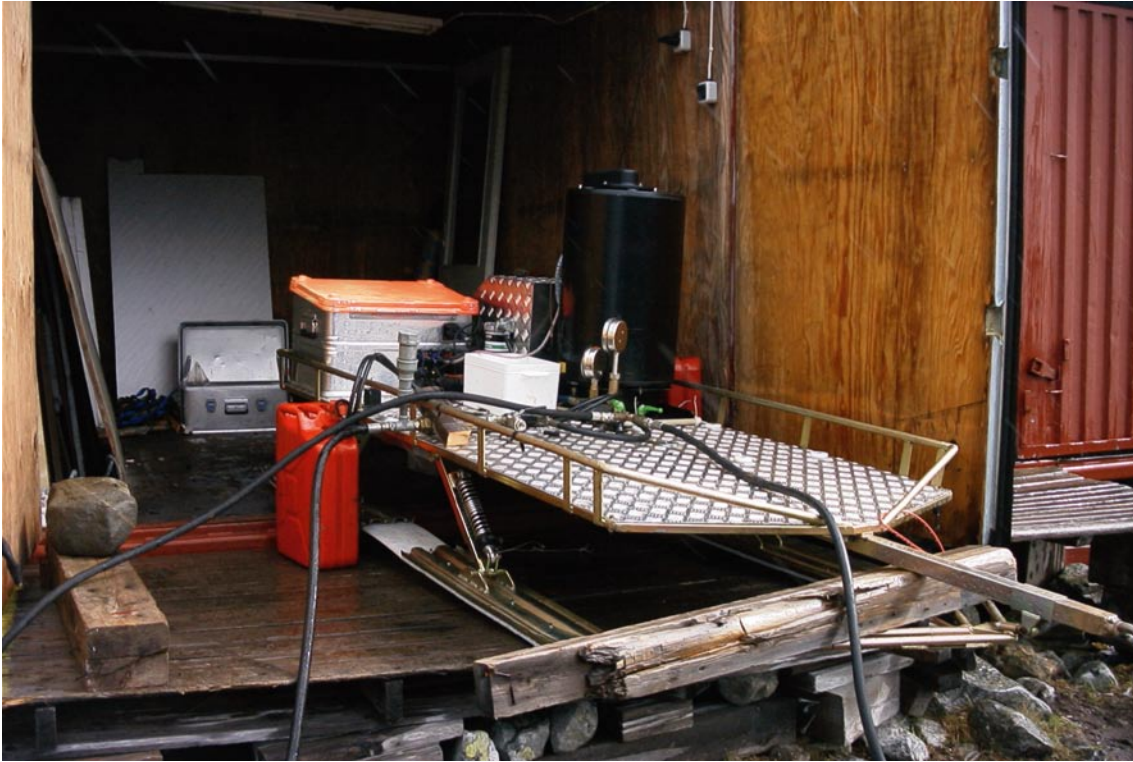
Figure 5-2. The Stockholm University hot water drill, burner and operation electronic unit assembly. Photo Peter Jansson ©.
