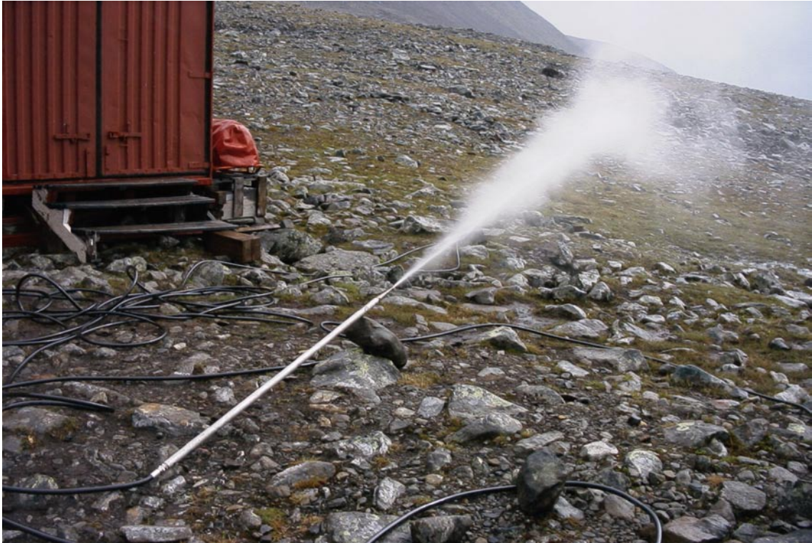
Figure 5-4. The hot water drill 2 m drill-stem and nozzle under full pressure. Photo Peter Jansson ©.
