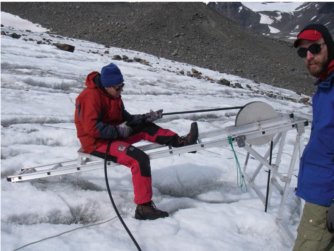
Figure 5-5. The hot water drill drill-rig in operation. Use of the rig enables better control of the drilling process to e.g. prevent non-vertical boreholes. Photo Peter Jansson ©.
