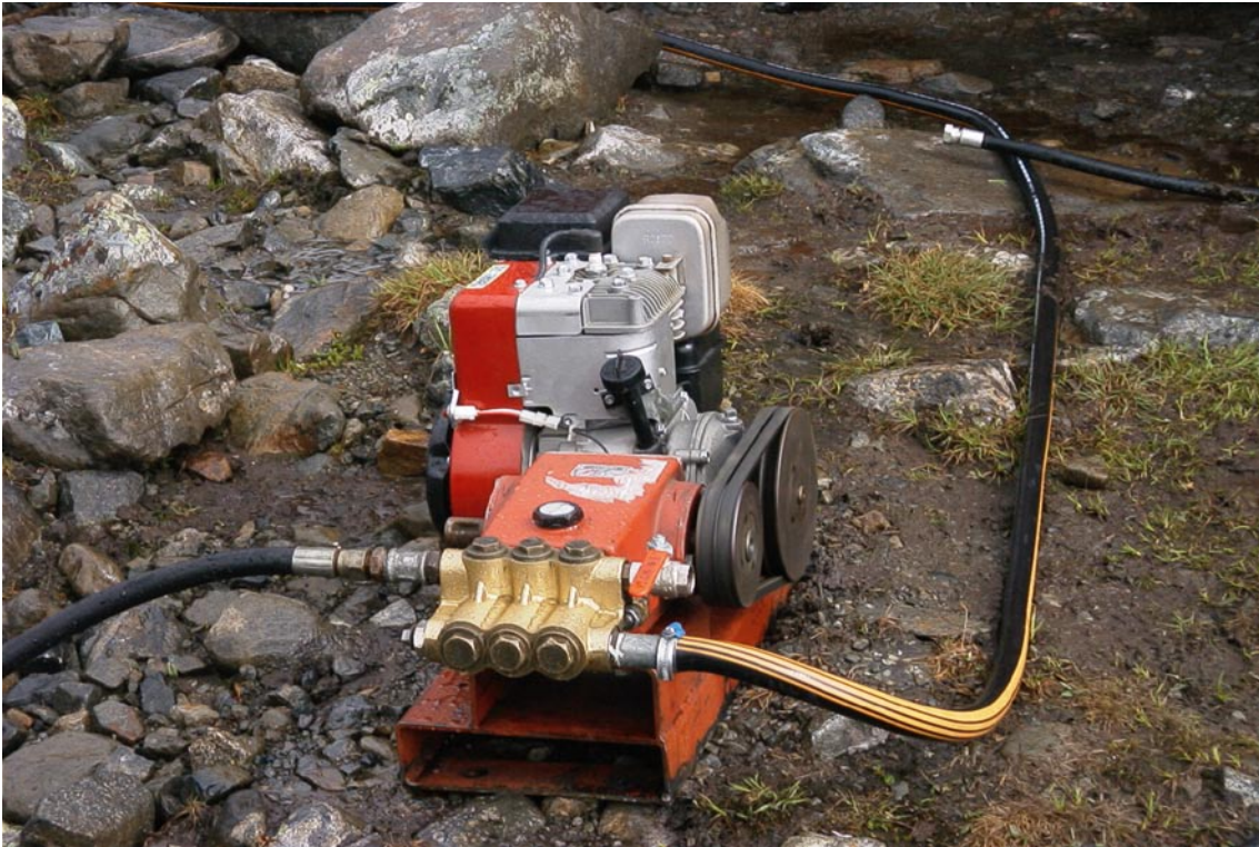
Figure 5-3. The Speck high pressure piston pump used to drive water through the hot water drill system. Photo Peter Jansson ©.
