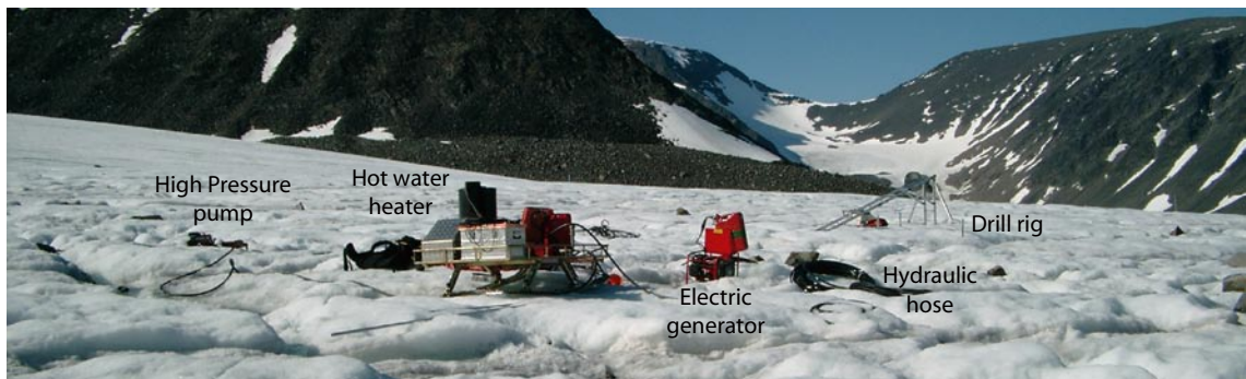
Figure 5-1. The Stockholm University hot water drill in operation on Storglaciären. Photo Peter Jansson ©.
