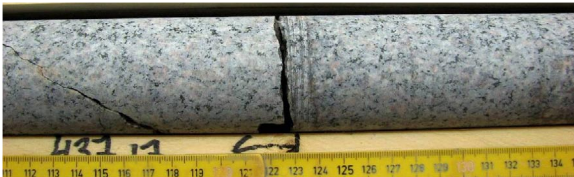
Figure 5-9. Photograph of fracture KLX09: 437.210 m.
