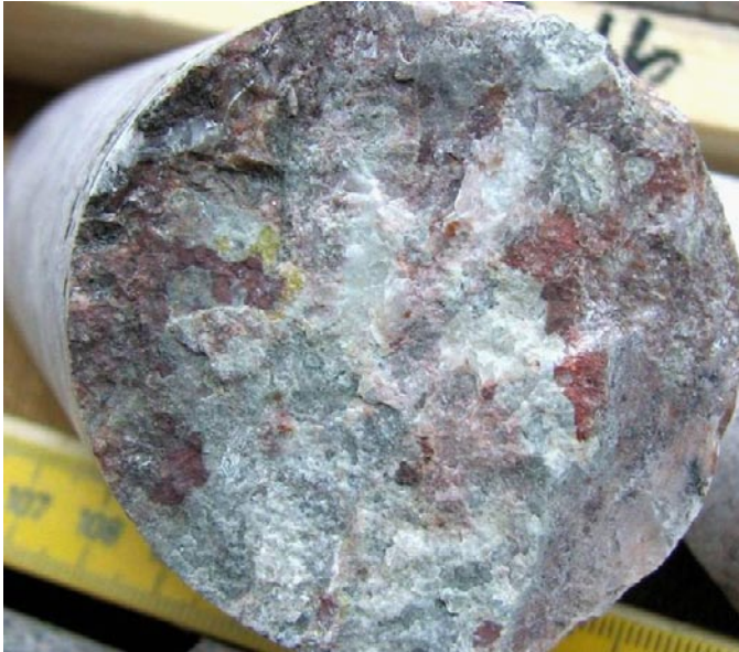
Figure 5-38. Photograph of the fracture surface of open fracture KLX16A: 348.067 m from drill core sample KLX16A: 348.01–348.14 m.
