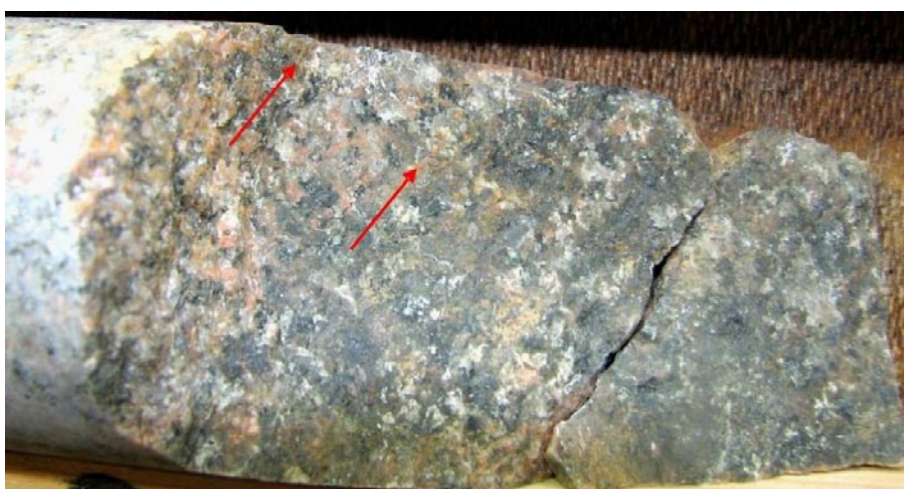
Figure 5-49. Photograph of drill core sample KLX07A: 432.15–432.27 m with open fracture KLX07A: 432.144 m. Arrows indicate powder mapped as goethite.
