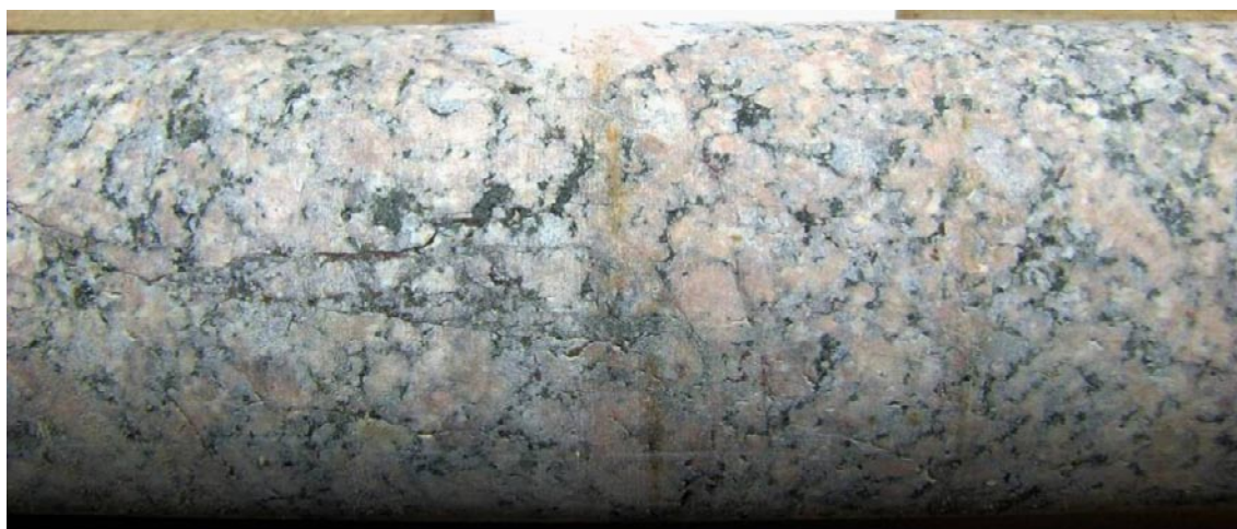
Photograph of sealed network section KLX04: 239.554–239.652 m.
