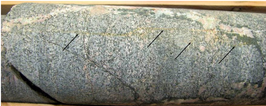
Photograph of sealed network section KLX04: 674.848–676.405 m.
