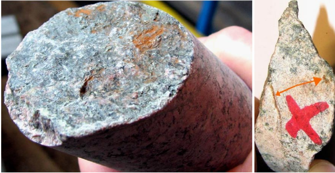
Figure 5-5. Photographs of fracture KLX08: 388.561 m. Arrows show drilling induced mineral fragments on the side of the drill core.
