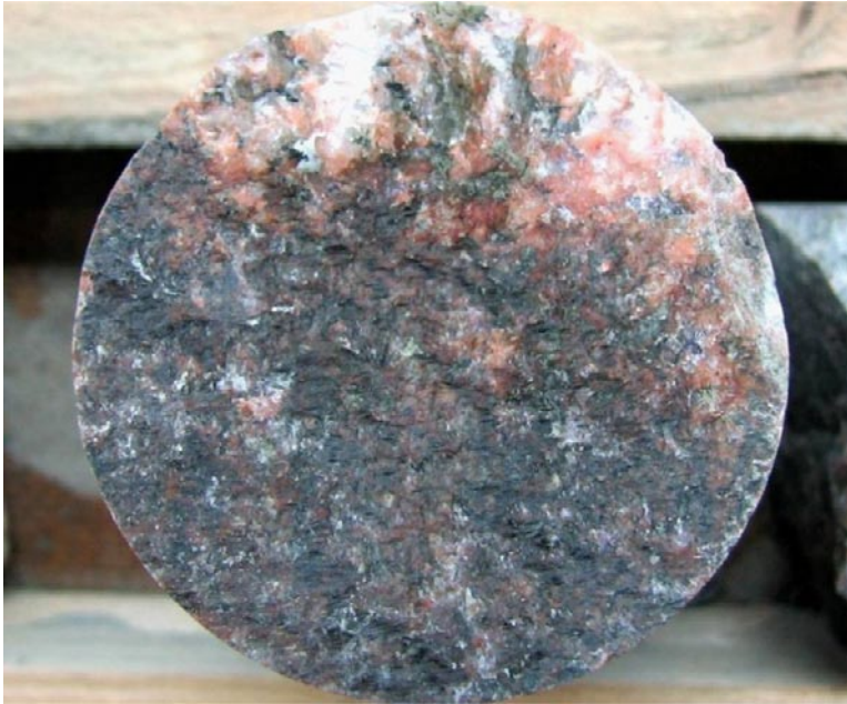
Photograph of open fracture KLX09: 574.242 m.
