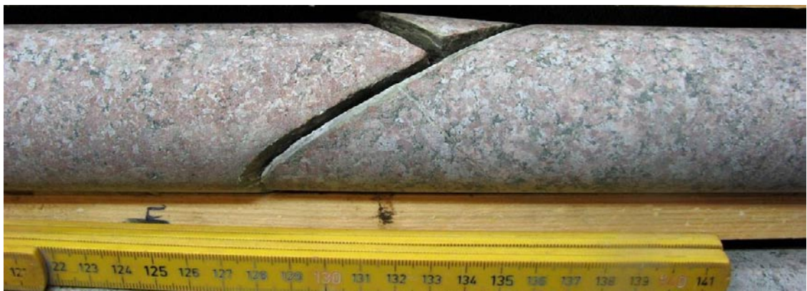
Figure 5-1. Photograph of fracture KLX08: 388.349 m.
