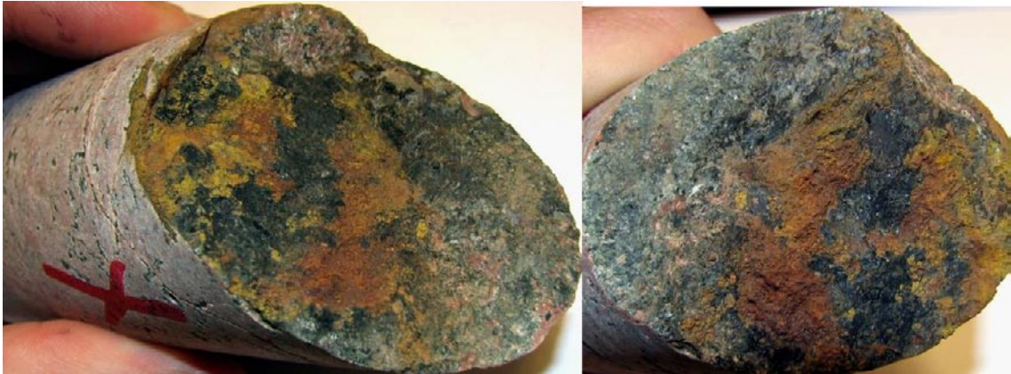
Figure 5-34. Photograph of the two fracture surfaces of open fracture KLX15A: 379.524 m (sample KLX15A: 379.39–379.63 m).
