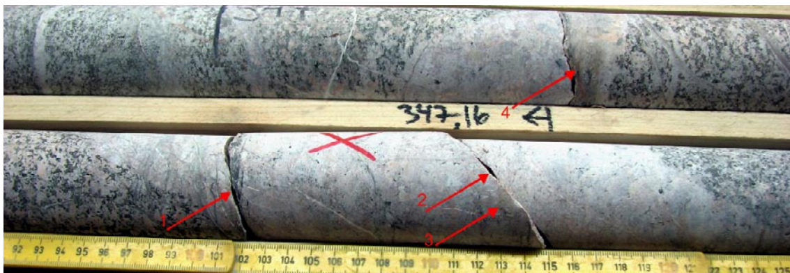
Figure 5-37. Photograph of drill core sample KLX16A: 348.01–348.14 m (X), 1) fracture 348.067 m, 2) 348.173, 3 and 4) oxidized metallic markings on the core, resulting from drill wear.
