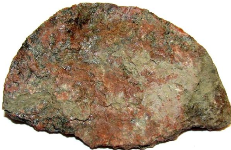
Figure 5-28. Photograph of the fracture surface of open fracture KLX13A: 550.762 m.
