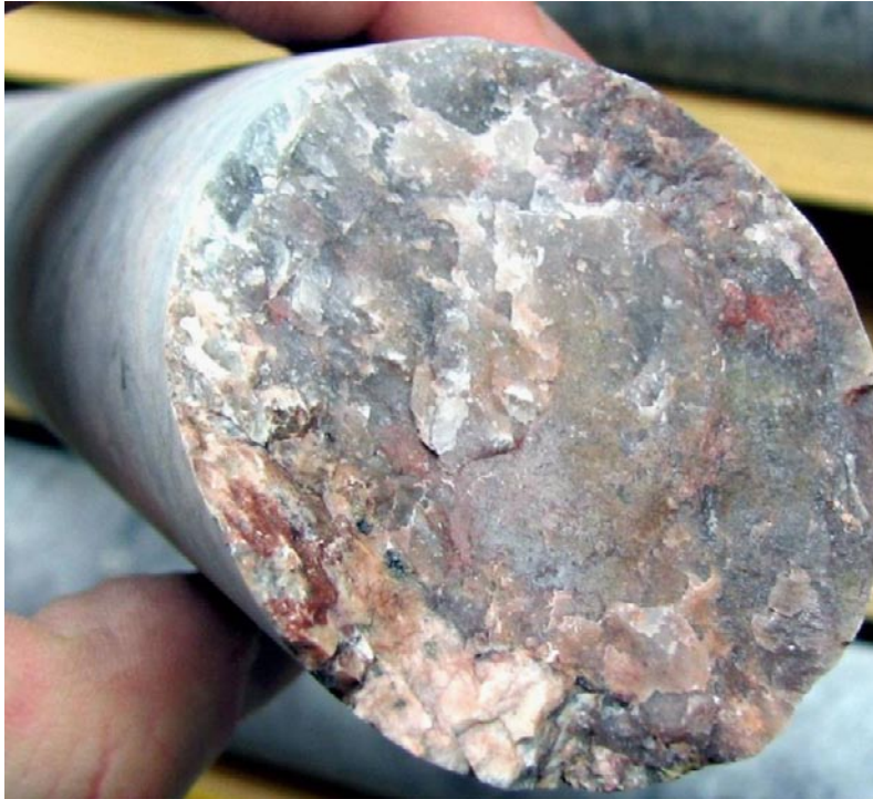
Photograph of open fracture KLX05: 518.300 m.
