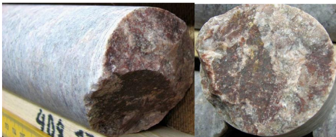
Figure 5-53. Photographs of drill core sample KLX16A: 408.23–408.27 m, showing fracture KLX16A: 408.237 m (upper fracture in photo to the left, right fracture in the photo to the right) and KLX16A: 408.241 m (lower fracture in photo to the left, left fracture in the photo to the right).
