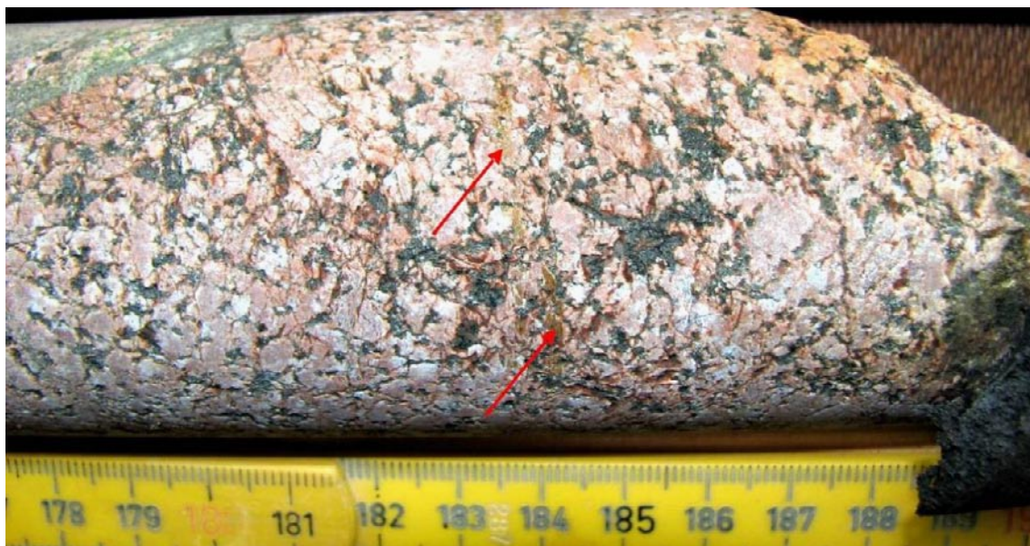
Photograph of sealed network section KLX13A: 576.768–576.897 m. Arrows indicate metallic markings on the core, resulting from drill wear.
