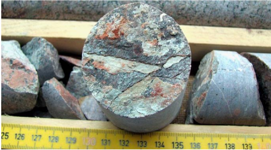
Figure 5-21. Photograph of sample KLX10: 704.32–704.44 m with fracture surface of open fracture KLX10: 704.339 m shown.
