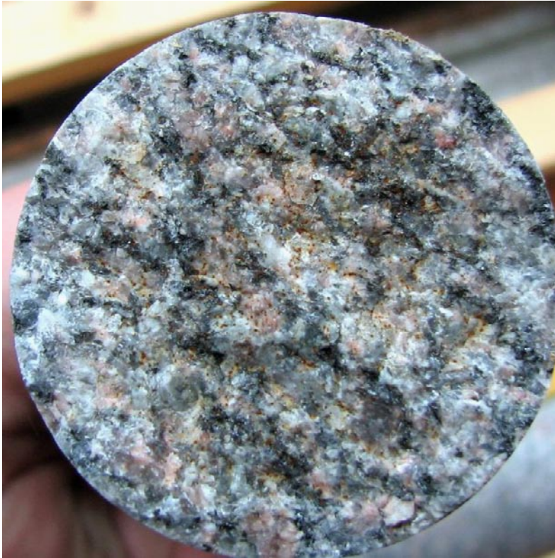
Figure 5-10. Photograph of fracture surface from open fracture KLX09: 437.210 m.
