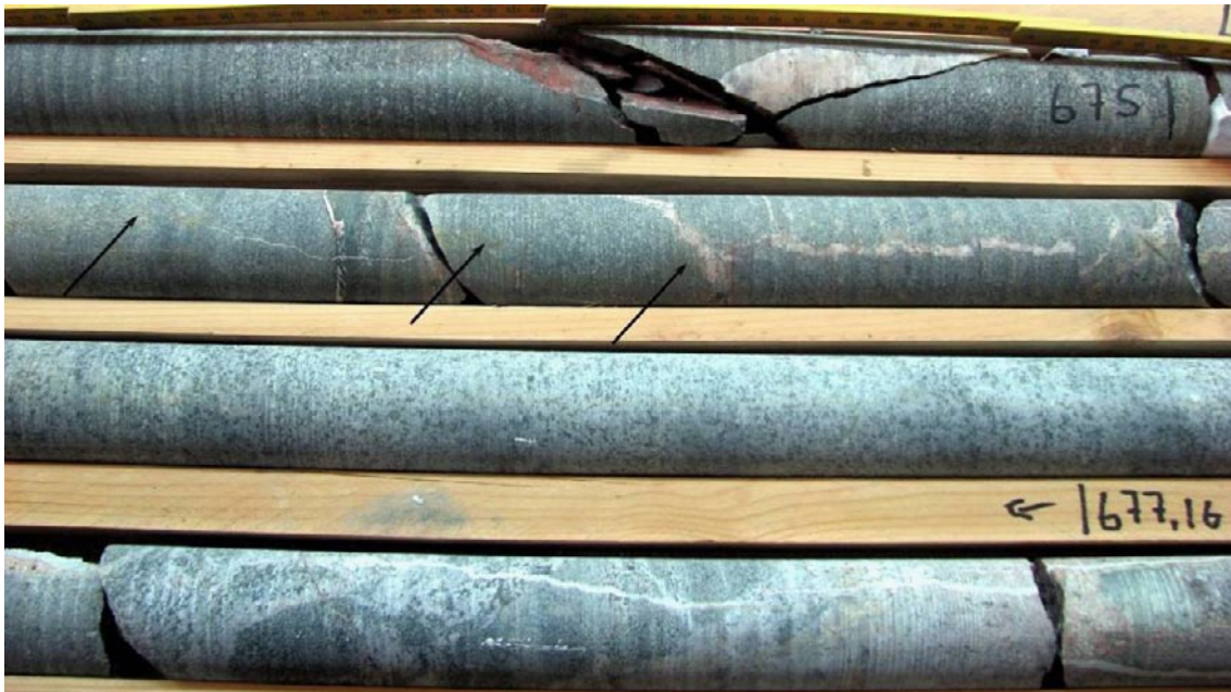
Photograph of sealed network section KLX04: 674.848–676.405 m.
