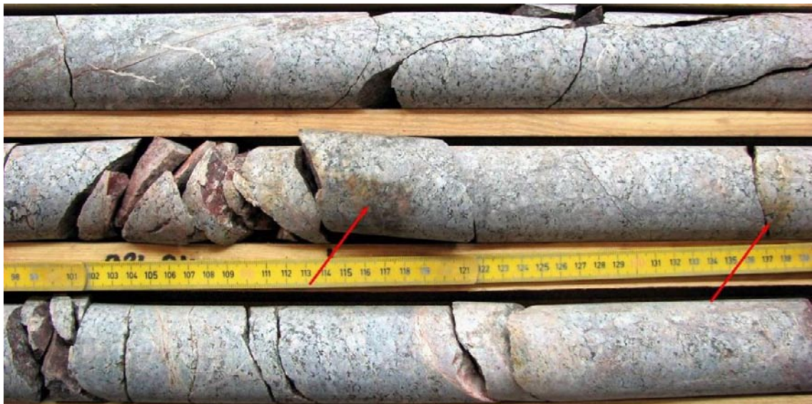
Photograph of section KLX04: 963.19–963.26 m for which goethite is included in the comment file for the alteration features.
