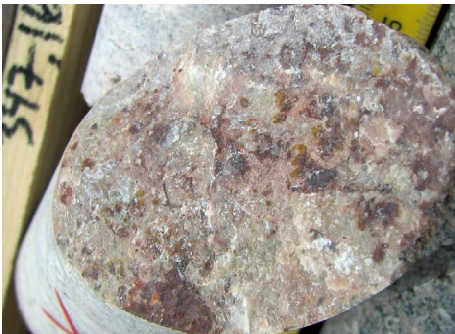
Figure 5-40. Photograph of the fracture surface of fracture KLX16A: 348.173 m from drill core sample KLX16A: 348.01-348.14 m.
