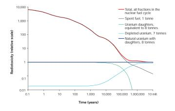
Radiotoxicity on ingestion via food for uranium ore (blue line) and all fractions that arise when the same quantity of uranium ore is used in the nuclear fuel cycle (red line). The different fractions are the spent nuclear fuel, the depleted uranium and the uranium daughters that are separated in the uranium mill.
