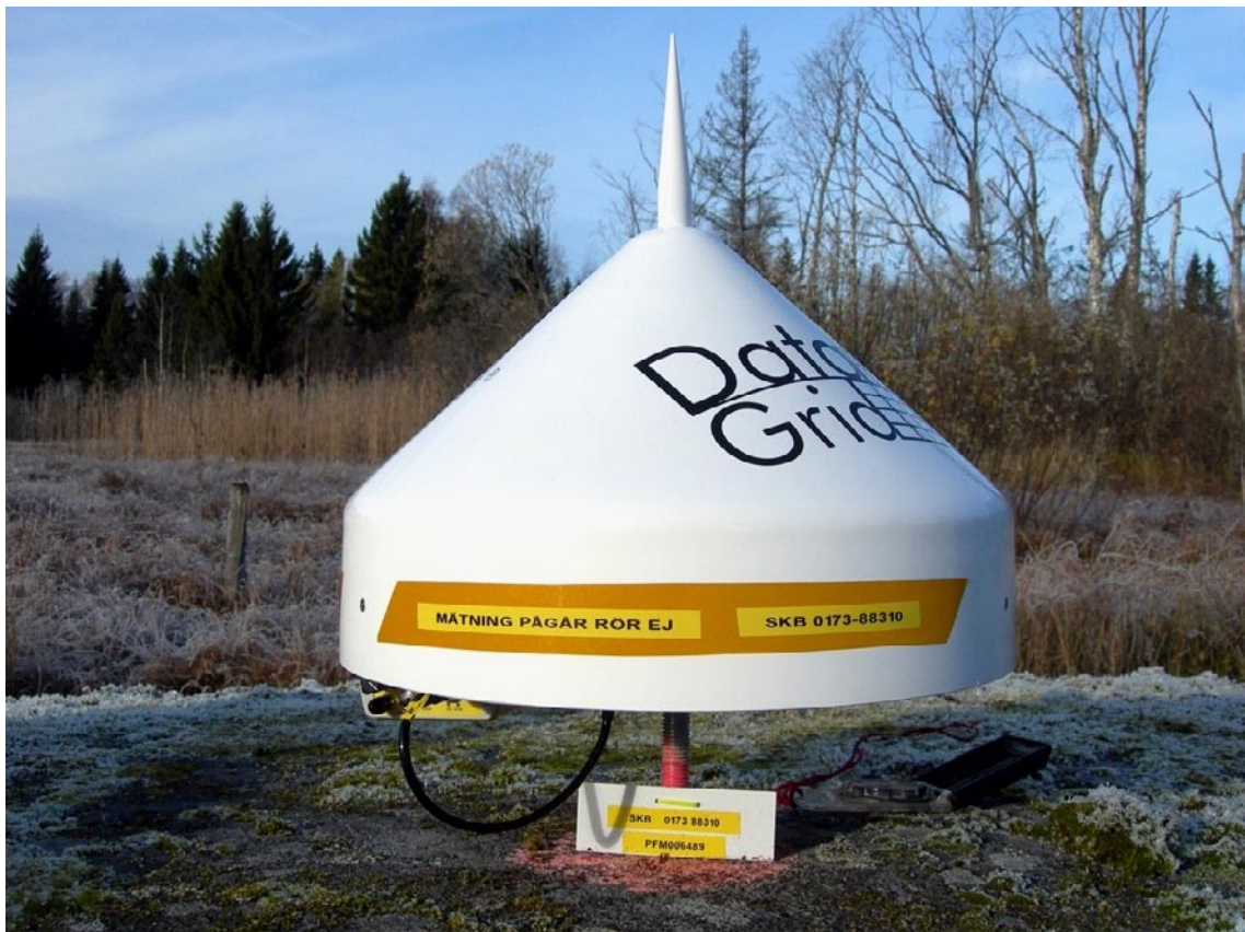
Figure 3-1. Sample station with choke ring antenna and GPS receiver mounted to the lower left. The station in this picture is PFM006489 but all sites have identical hardware (and firmware). They are mounted on a short steel rod anchored in the rock for good mechanical and thermal stability. However, the low mounts increase the demand on the GPS environment. The antenna radome and pin are designed to protect the active components of the antenna and discourage birds and other small animals from lodging on the antenna. A second cover provides additional protection between measurement campaigns.
