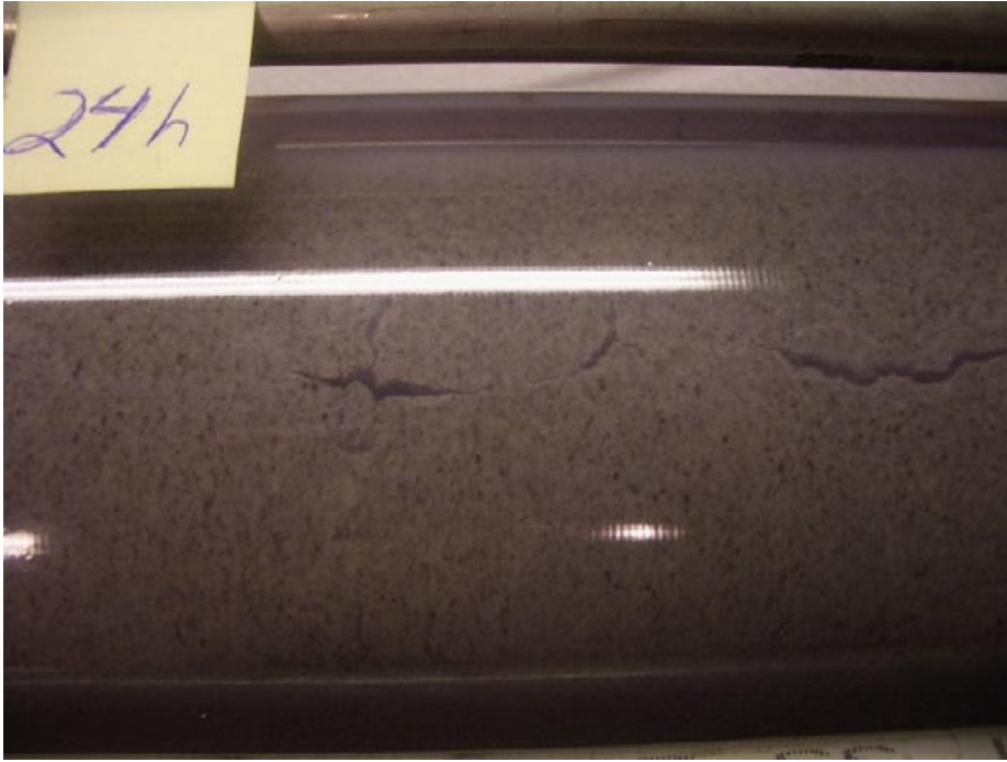
Figure 3-35. Picture taken 24 hour after finishing the pre-wetting of the outer slot. The air-pockets are still very clear.
