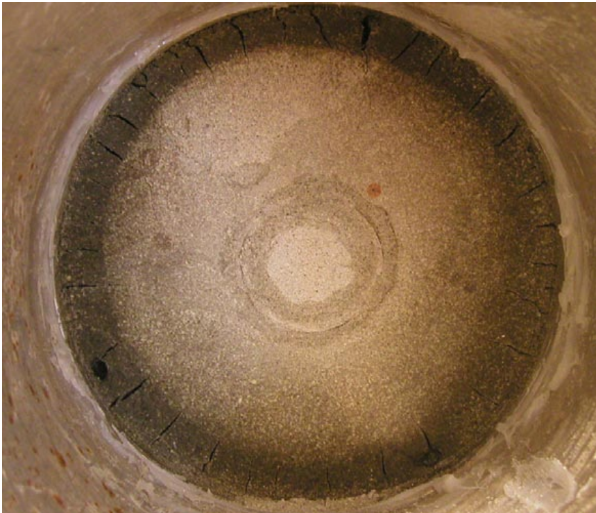
Figure 3-5. Picture showing the outermost part i.e. against the load cells after removing the fixing ring.
