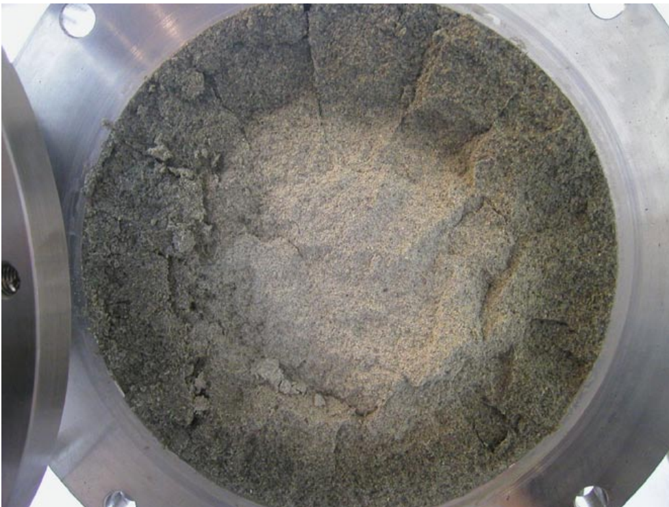
Figure 3-16. Picture taken during decomposition of the test, about 1.5 m from the supercontainer section. The dark ring has a width of 35–40 mm. The water ratio was determined in some positions; see Table 3-4.
