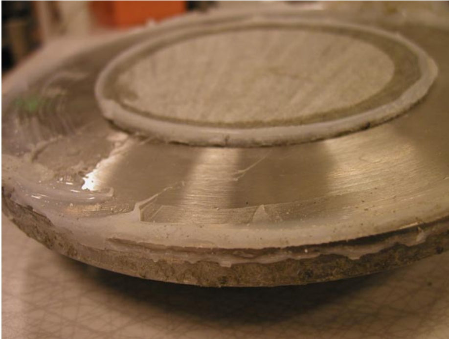
Figure 3-23. Picture showing the fixing ring after termination of the test. The block closest to the ring has been squeezed through the central hole in the steel ring. The total displacement was estimated to 12 mm.
