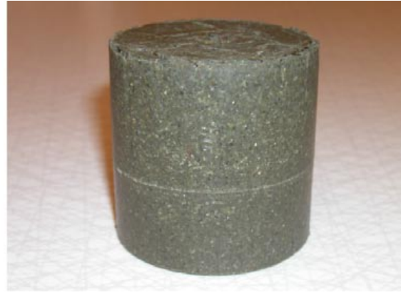
Figure 8-4. Sample of compacted bentonite after opening and removal from test set-up used in the Lasgit experiment. Note shrinkage cracking on the surface. The sample diameter is about 50 mm (from Clay Technology AB).
