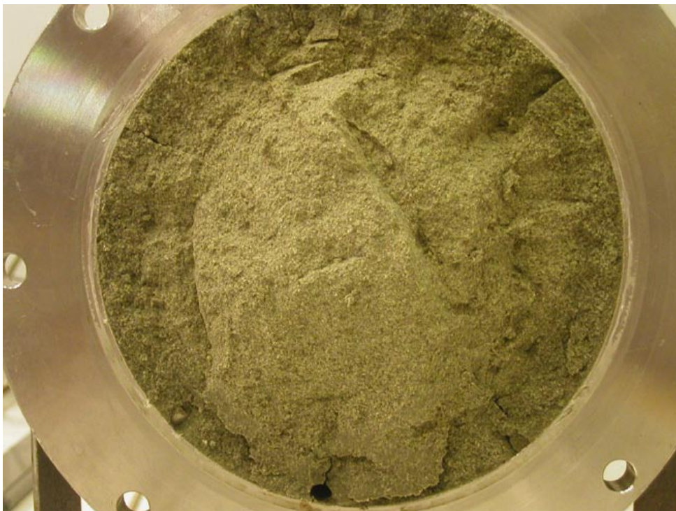
Figure 3-28. Picture taken during decomposition of the test, about 1.5 m from the supercontainer section. The remaining hole from the drainage tube is still open.
