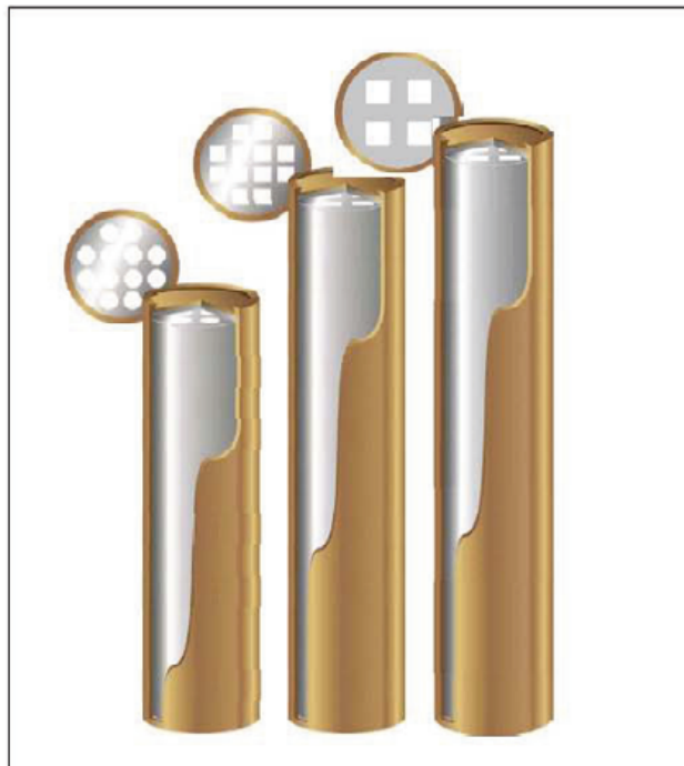
FIGURE 1. Artist's view of the Posiva type canisters, VVER 440 type left, BWR type middle, and EPR type right.
