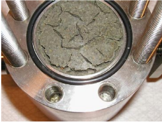
Figure 8-4. Sample of compacted bentonite after opening and removal from test set-up used in the Lasgit experiment. Note shrinkage cracking on the surface. The sample diameter is about 50 mm (from Clay Technology AB).
