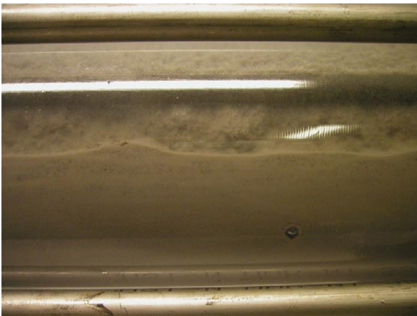
Figure 3-32. Picture taken just after finishing the pre-wetting of the outer slot. Bentonite has loosened from the blocks and settled down. Half of the slot is still filled with clear water.
