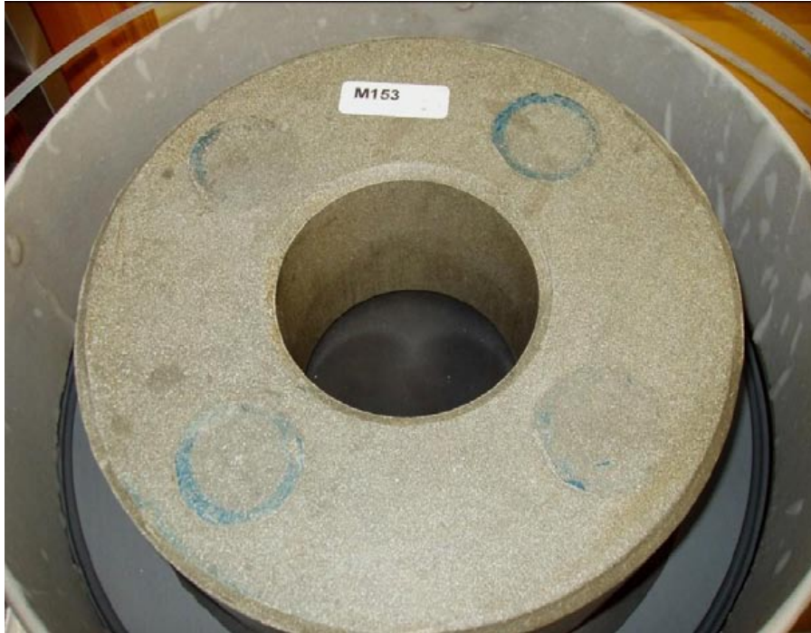
Figure 2-19. Picture showing block sample M153 after 3 months test duration. No cracks could be seen on the surface.
