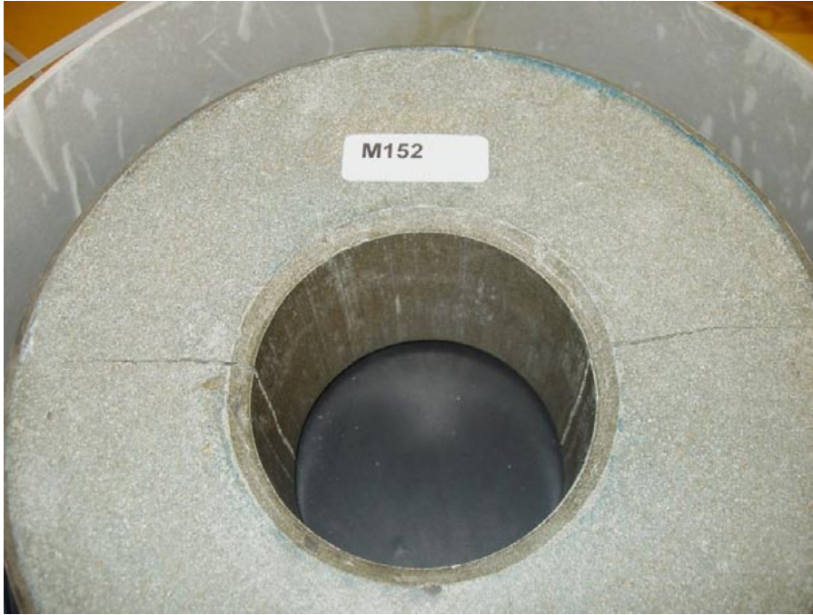
Figure 2-17. Picture showing block sample M152 ( w_{mi} = 20\% , RH = 100\% , gap = 45\text{ mm} ) after 7 days test duration.
