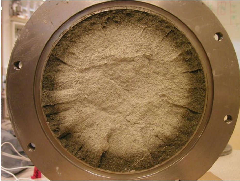
Figure 3-6. Picture from the middle of the sample about 0.5m from the pressure side. The water ratio was determined in some positions with the following results: Uppermost 5 mm = 30%, next 5 mm = 29%, next 5 mm = 28%, next 5 mm = 25%, and in the centre = 17%.
