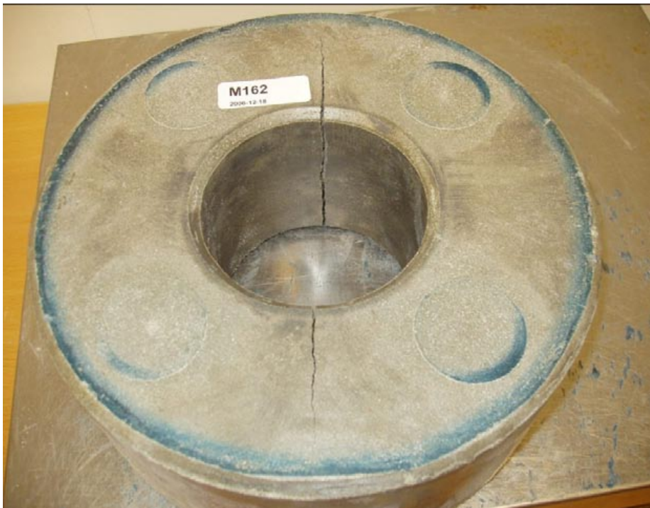
Figure 2-18. Picture showing block sample M162 ( w_{mi} = 20\% , RH = 100\% , gap = 65\text{ mm} ) after 3 months test duration. The block was still in one piece but there was an evidently diametrical crack which occurred after about one months test duration.
