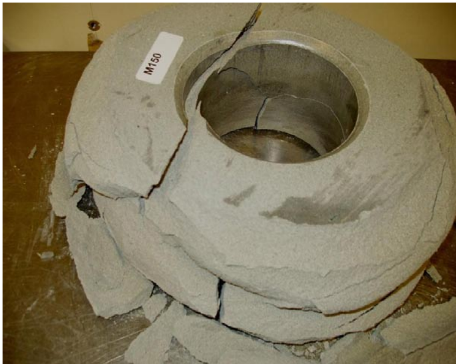
Figure 2-16. Picture showing block sample M150 ( w_{ini} = 13\% , RH = 100\% , gap = 45\text{ mm} ) after 8 hours test duration.
