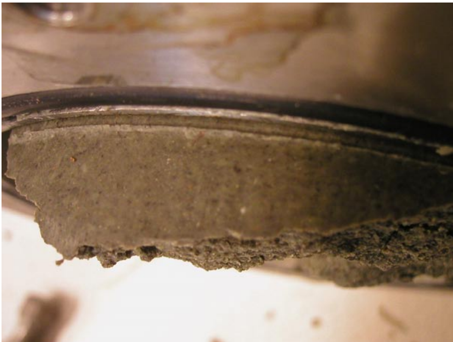
Figure 3-8. Picture from the middle of the sample showing a part of the outer surface. No cracks could be seen.
