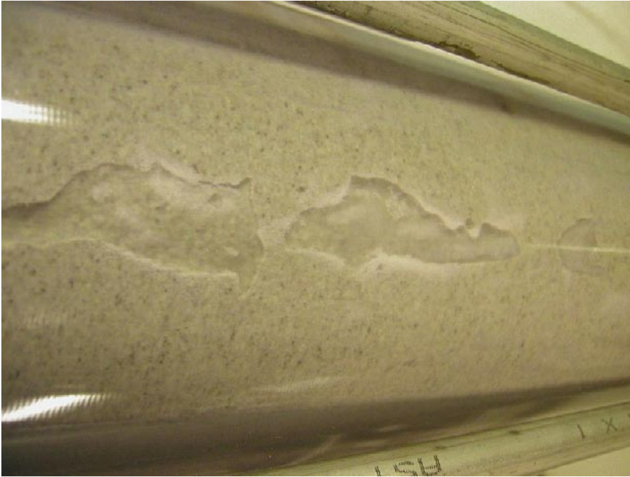
Figure 3-33. Picture taken from above about 0.5 hour after finishing the pre-wetting of the outer slot. In spite of the inclination of the tube (about 2°) there are a number of air-pockets on the upper side.
