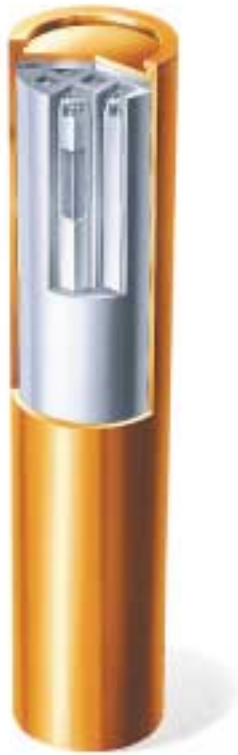
Figure 4-3 Copper canister with a cast iron insert.
