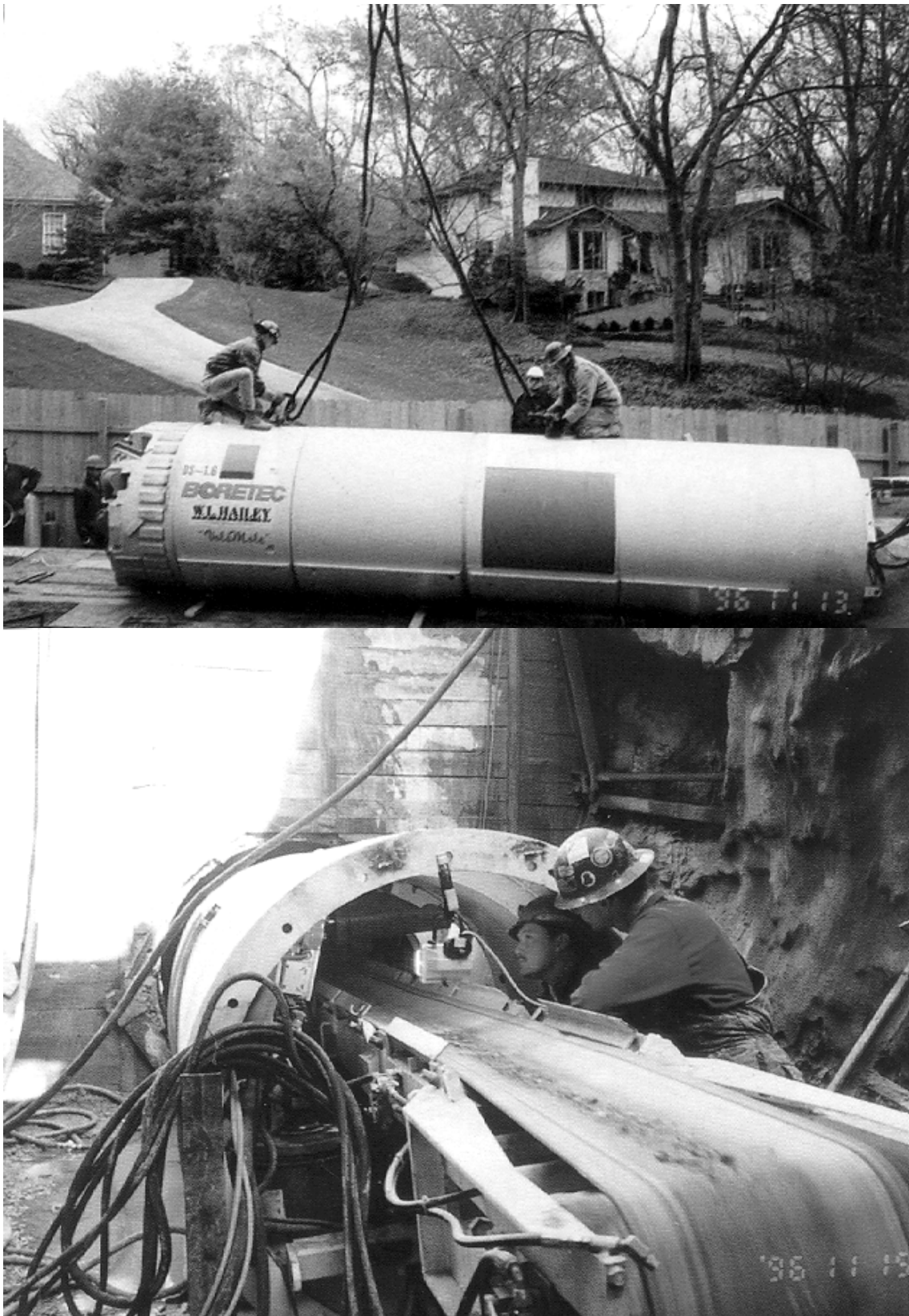
Figure 3-2 Tunnel boring machine suitable for boring of deposition tunnels for the MLH system (from Wallis, 1997).
