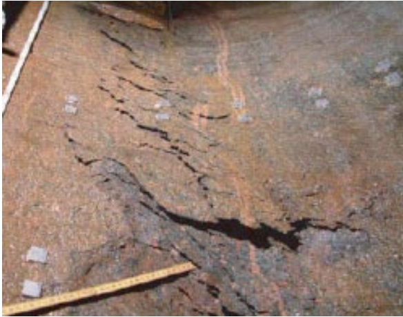
Figure 6-11. Spalling at Äspö on the vertical surface of a full-scale deposition hole in the APSE experiment /Andersson and Eng 2005/.
