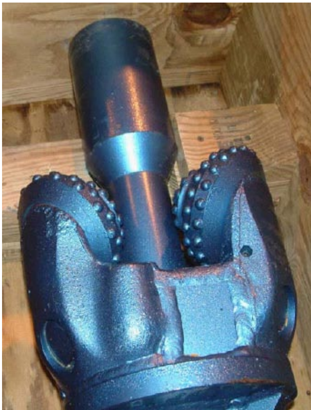
Figure 4-52. Pre-pilot hole could be reamed with a special pilot bit equipped with a guiding pin /Bäckblom and Lindgren 2005/.
