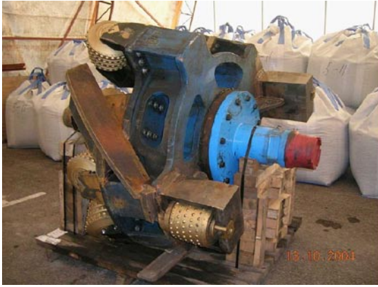
Figure 4-42. The cutter head at site (left) and during operation (right).
