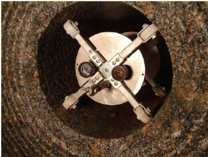
Figure 4-50. Device used for measuring the straightness of the pilot hole in the demonstration at Äspö /Bäckblom and Lindgren 2005/.
