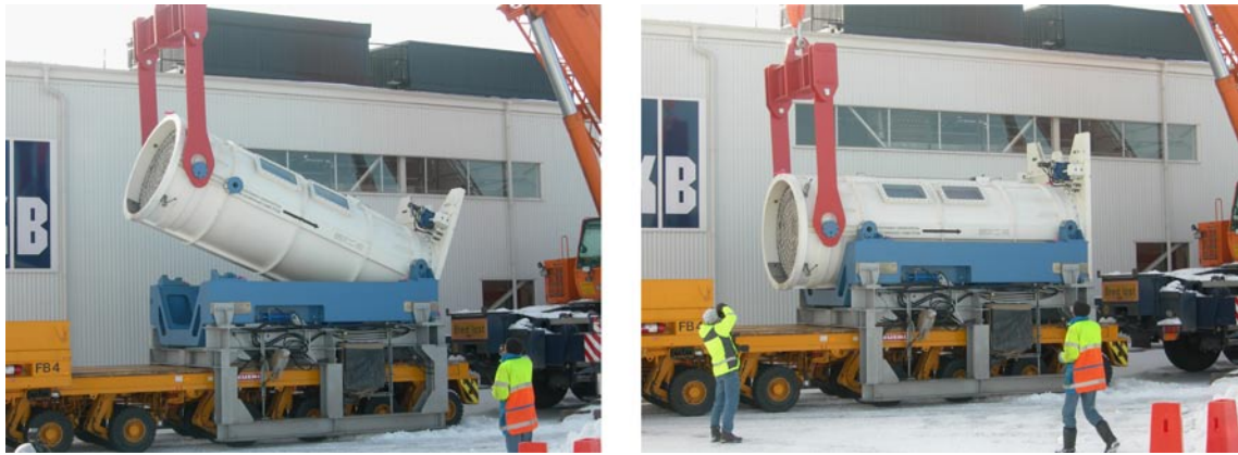
Figure 4-33. The supercontainer is placed into a transport tube for transportation down to the underground test site at Äspö HRL.
