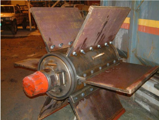
Figure 4-46. Stabilizers used to support the drill string.
