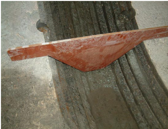
Figure 4-19. Template for verifying the shape of the notch for the compartment plug.
