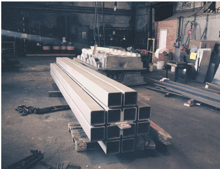
Figure 2-7. Welded cassette with 12 channels for BWR assemblies.
