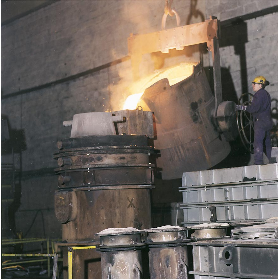
Figure 2-8. Casting of an insert.
