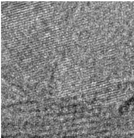
Figure 5-16. This is a magnification of the TEM image of sodium montmorillonite in Figure 5-15a showing the lamellar structure built of individual clay platelets. In some areas of the picture the resolution is high enough to reveal the individual atomic layers.
