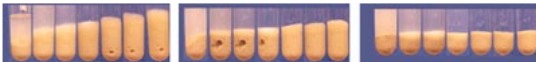
Figure 5-9. Ca montmorillonite in contact with NaCl solutions of varying concentrations; from left to right the concentrations are 0.2, 0.5 and 2 M, respectively. The tube photos in each figure has been taken after 1min, 5min, 10min, 1h, 1 day, 4 days and 20 days, respectively.
