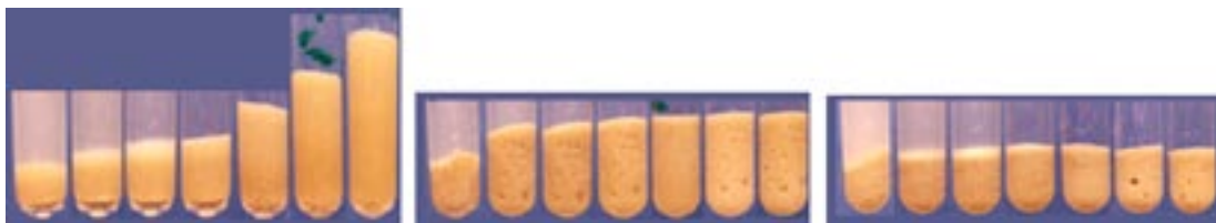
Figure 5-10. Na montmorillonite in contact with CaCl 2 solutions of varying concentrations; from left to right the concentrations are 0.01, 0.05 and 0.1 M, respectively. The tube photos in each figure has been taken after 1min, 5min, 10min, 1h, 1 day, 4 days and 20 days, respectively.
