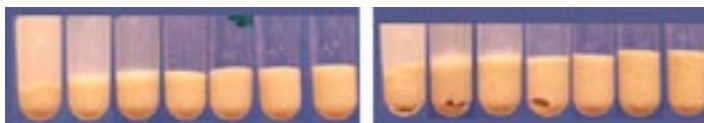
Figure 5-11. Ca montmorillonite in contact with CaCl 2 solutions of varying concentrations; from left to right the concentrations are 0.01 and 0.05, respectively. The tube photos in each figure has been taken after 1min, 5min, 10min, 1h, 1 day, 4 days and 20 days, respectively.
