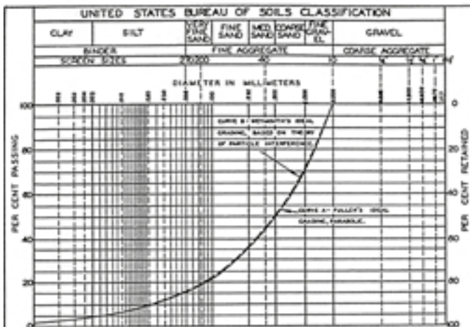
Figure 2-4. Examples of crushed muck of unweathered granitic rock. The diagram in the middle indicates that repeated crushing reduces the size of larger particles rather little, and that as much as 5–10% is finer than 0.1 mm. The curve representing TBM muck is coarser but still contains about 10% smaller than 0.1 mm /Gunnarsson et al. 2002/. The lowermost diagram shows the theoretical Fuller size distribution for comparison /Pusch 2002b/.
